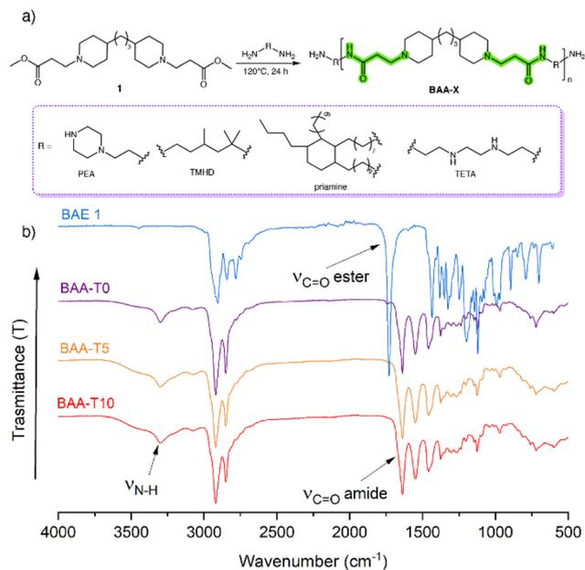
**Fig. 2** (a) Synthesis of the linear dynamic curing agent; (b) IR comparison of compound **1**, **BAA-T0**, **BAA-T5** and **BAA-T10**.
