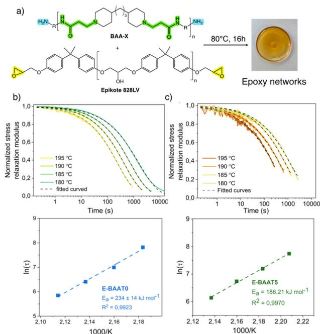
**Fig. 3** (a) Reaction scheme of the dynamic networks and representative picture of E-BAAT5 obtained; (b and c) stress relaxation curves (top) and Arrhenius plot (bottom) of E-BAAT0 (left) and E-BAAT5 (right).
