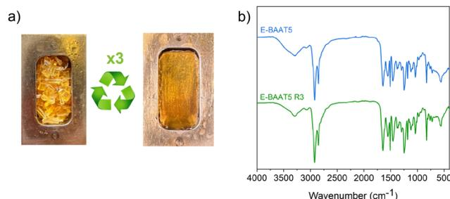
Fig. 4 (a) Reprocessing of E-BAAT5 epoxy network conducted at 200 °C for 30 minutes under a pressure of 3 tonnes/m<sup>2</sup>; (b) FTIR spectra comparison of the initial E-BAAT5 and the third-time reprocessed sampled E-BAAT5 R3.
