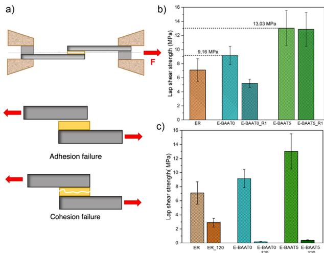
**Fig. 5** (a) Schematization of the lap shear strength experiment (top) and different types of failure that can occur across the adhesive area (bottom); (b) lap shear test results compared at room temperature and after the first recycling (top); (c) lap shear test results tested at 120 °C compared to the one at room temperature.
