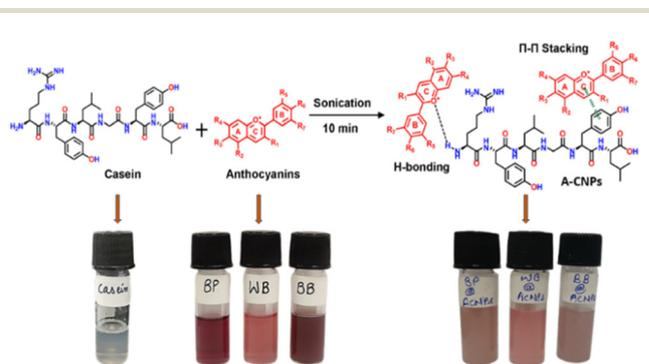
**Scheme 1** Schematic presentation the synthesis of A-CNPs from anthocyanins and casein using sonication as a top-down technique.
