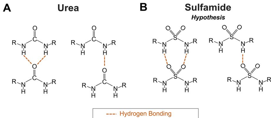
Fig. 1 Schematics of the (A) two potential H-bonding patterns in polyurea according to Mattia *et al.*<sup>32</sup> and (B) two hypothesized H-bonding patterns in polysulfamide.
