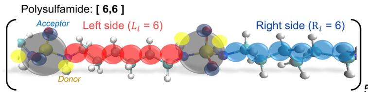
**Fig. 3** CG representation of the repeat unit in the [6,6] polysulfamide chain with six  $-\text{CH}_2-$  on the left and right sides of the sulfamide group in the repeat unit.
