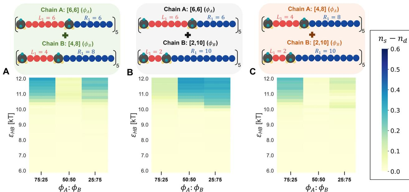
**Fig. 9** Heat maps showing the difference in H-bonding between identical chain types ( $n_s$ ) and different chain types ( $n_d$ ) using the atomistically informed CG Config-1 model for the three mixtures – (A) [6,6] and [4,8], (B) [6,6] and [2,10], and (C) [4,8] and [2,10] – at varying H-bonding strengths (y-axis) and mixture compositions (x-axis).
