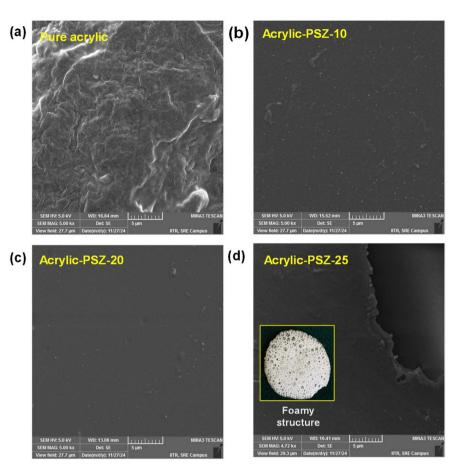
Fig. 6 SEM micrographs of adhesives with different PSZ concentrations (a) pure acrylic polymer (b) adhesive with 10 wt% of PSZ, (c) adhesive with 20 wt% of PSZ, (d) adhesive with 25 wt% of PSZ, generating a foamy structure, inset picture shows foamy structure formed by reaction with excess
