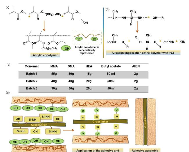
Fig. 1 (a) Copolymer synthesis reaction, (b) Curing reaction of PSZ with Acrylic copolymer, (c) different formulations of the acrylic resin, (d) schematic representation of adhesion curing and adhesive assembly.
