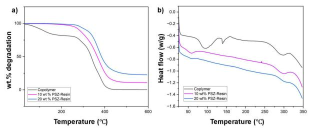
Fig. 3 (a) Thermal stability and (b) thermal transition profile of the polymer.
