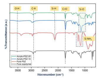
Fig. 2 FTIR spectrum between copolymer and PSZ.
