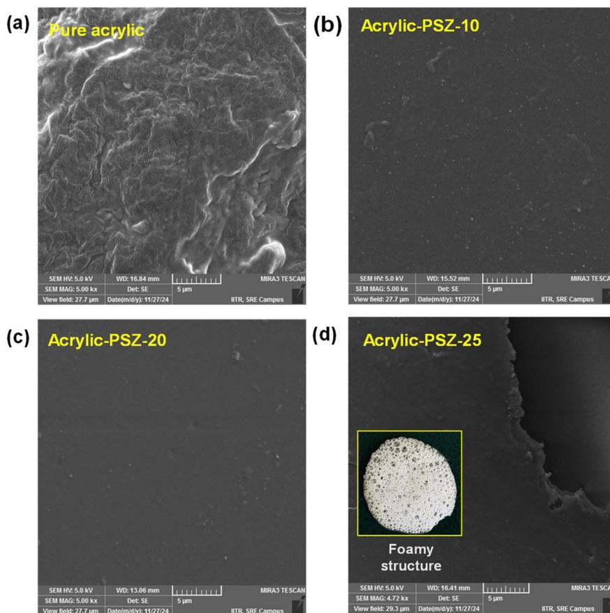
**Fig. 6** SEM micrographs of adhesives with different PSZ concentrations (a) pure acrylic polymer (b) adhesive with 10 wt% of PSZ, (c) adhesive with 20 wt% of PSZ, (d) adhesive with 25 wt% of PSZ, generating a foamy structure, inset picture shows foamy structure formed by reaction with excess PSZ.
