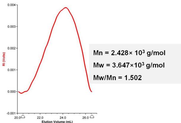
Fig. 4 Determination of molecular weight of the polymer by GPC.
