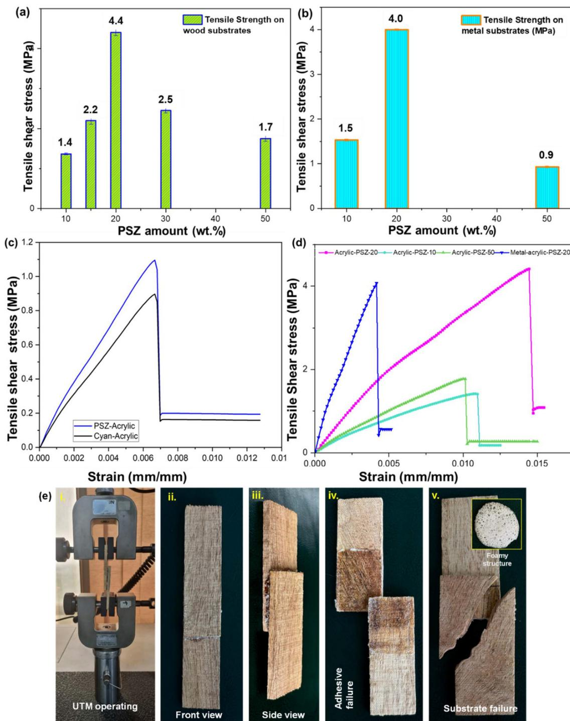
**Fig. 7** (a) Strengths of the polysilazane-cured adhesive formulations with wood substrates, (b) strengths of the polysilazane-cured acrylic adhesive formulations for metal substrates, (c) Tensile shear strengths of acrylic adhesive formulations with conventional crosslinker and PSZ, (d) Tensile shear strengths of adhesives with varying amount of PSZ, (e) UTM operating assembly and substrate pictures, with modes of failure, inset picture with foamy-structure of formulation with excess PSZ.
