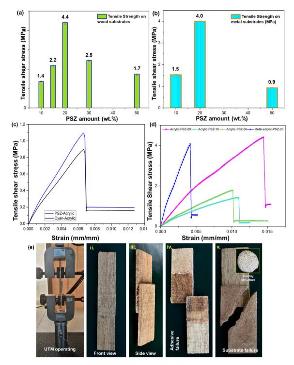
Fig. 7 (a) Strengths of the polysilazane-cured adhesive formulations with wood substrates, (b) strengths of the polysilazane-cured acrylic adhesive formulations for metal substrates, (c) Tensile shear strengths of acrylic adhesive formulations with conventional crosslinker and PSZ, (d) Tensile shear strengths of adhesives with varying amount of PSZ, (e) UTM operating assembly and substrate pictures, with modes of failure, inset picture with foamy-structure of formulation with excess PSZ.
