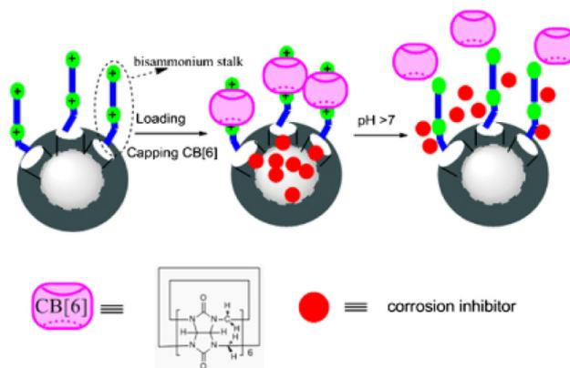
Fig. 8 Schematic illustration of the nanovalve-type smart responsive corrosion inhibitor with CB[6] macrocycle. Reproduced with permission<sup>95</sup> from IOP.
