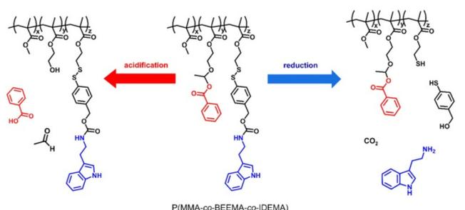
**Fig. 15** Selective release of the corrosion inhibitors benzoic acid (red) and tryptamine (blue) from a doubly reactive terpolymer by acidification and reduction. Reproduced with permission<sup>137</sup> from ACS.
