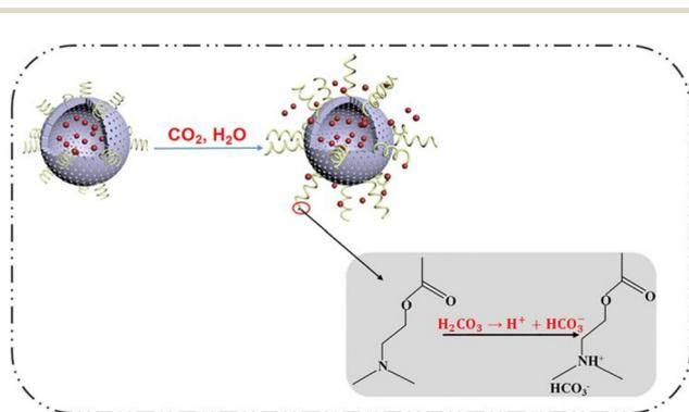
Fig. 17 Mechanism of the CO<sub>2</sub> stimulus response. Reproduced with permission<sup>39</sup> from Elsevier.
