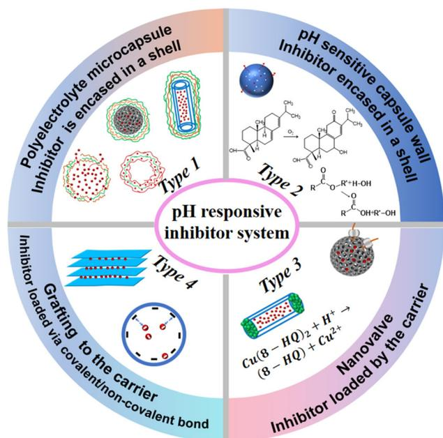
Fig. 1 Typical types of pH-responsive corrosion inhibitor system.
