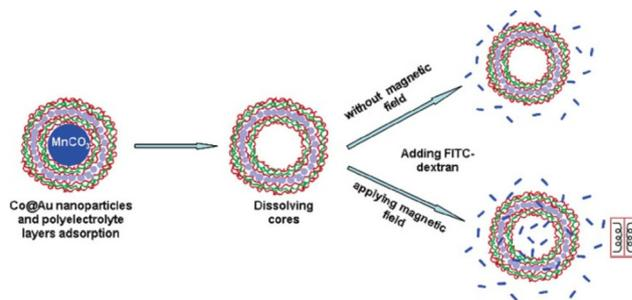
**Fig. 14** Scheme of Co@Au nanoparticle microcapsule assembly and magnetic permeability test under an oscillating magnetic field. Reproduced with permission<sup>131</sup> from ACS.
