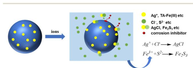
Fig. 3 Typical types of ion-responsive corrosion inhibitor system.
