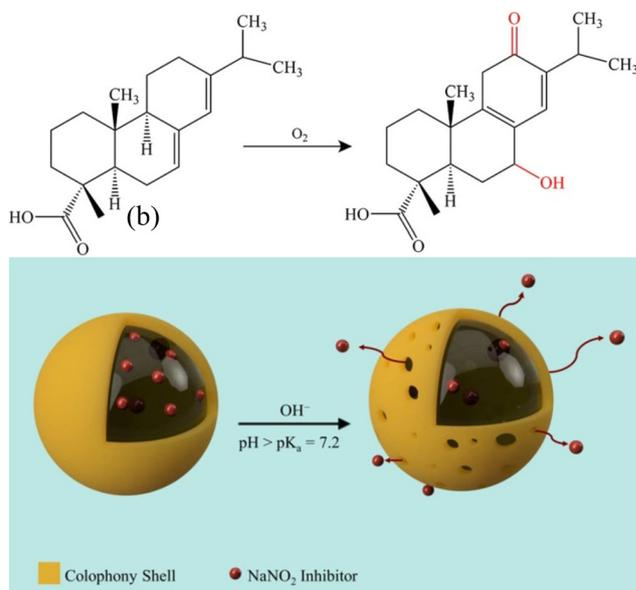
Fig. 6 Chemical structure of rosinic acid oxidation in solution and schematic illustration of the controlled release mechanism of resin microcapsules containing NaNO<sub>2</sub> inhibitor via OH<sup>-</sup>-induced porosity of the microcapsules. Reproduced with permission<sup>91</sup> from ACS.
