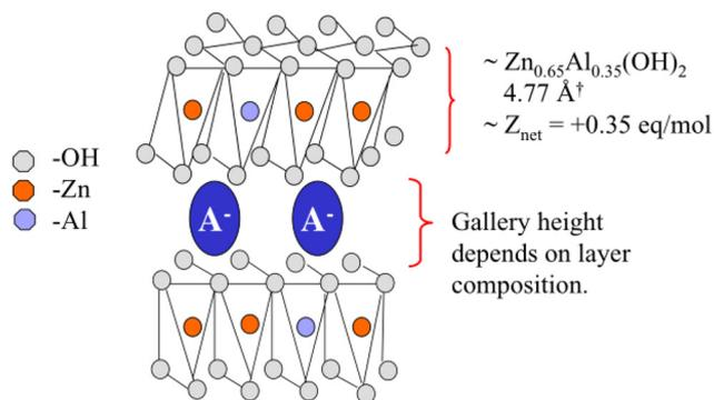
**Fig. 13** Schematic illustration of the layered structure of a hydrotalcite compound. The structure consists of alternating layers of positively charged mixed metal hydroxide sheets and anions. Reproduced with permission<sup>61</sup> from Elsevier.
