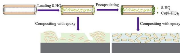
Fig. 7 Schematic illustration of the preparation of Cu-8-HQ@HNTs and Cu-8HQ@HNTs/epoxy coatings. Reproduced with permission<sup>92</sup> from Elsevier.
