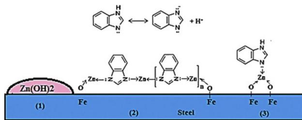
Fig. 12 Adsorption model of inhibitors released by Zn-MMT + BIA-MMT within artificial defects on steel surfaces. Reproduced with permission<sup>120</sup> from Elsevier.
