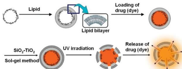
Fig. 11 Preparation procedure of drug (dye) controlled release UV-responsive (PSS/PDDA)<sub>5</sub>/PSS/DDAB/SiO<sub>2</sub>-TiO<sub>2</sub> capsules. Reproduced with permission<sup>52</sup> from ACS.
