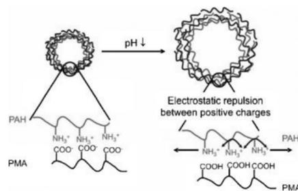
Fig. 5 Swelling model of (PAH/PMA)<sub>2</sub> capsules under acidic conditions. Reproduced with permission<sup>86</sup> from Wiley.
