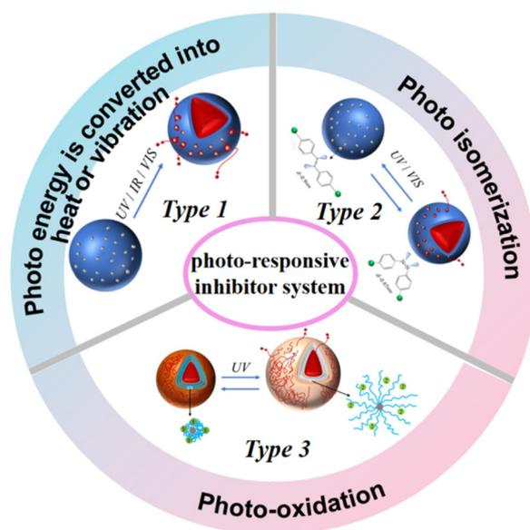
Fig. 2 Typical types of photoresponsive corrosion inhibitor system.
