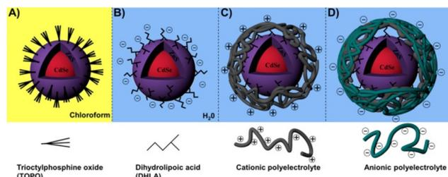
**Fig. 18** (A) TOPO-QDs in chloroform; (B) anionic water-soluble DHLA-QDs; (C) cationic polyelectrolyte-coated quantum dots; (D) anionic polyelectrolyte-coated quantum dots. Reproduced with permission<sup>150</sup> from ACS.
