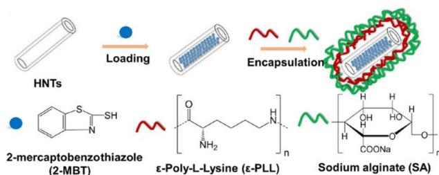
Fig. 16 Schematic illustration of the fabrication process of smart microcapsules (MCs). Reproduced with permission<sup>147</sup> from ACS.
