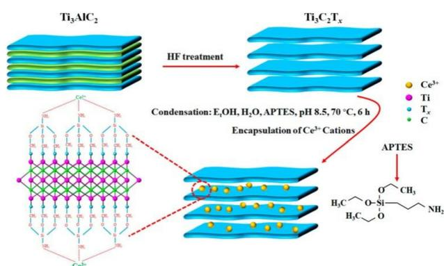
**Fig. 10** Schematic illustration of the preparation, surface modification, encapsulation principle and inhibition mechanism of  $\text{Ti}_3\text{C}_2$  MXene- $\text{Ce}^{3+}$  coating. Reproduced with permission<sup>50</sup> from ACS.
