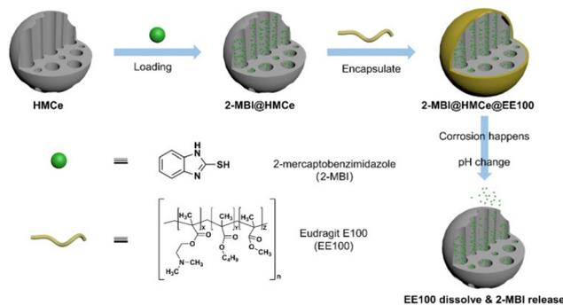
Fig. 4 Schematic illustration of the pH-responsive inhibitor system with Eudragit E100. Reproduced with permission<sup>80</sup> from Elsevier.
