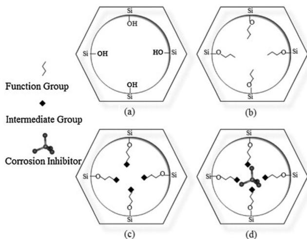
**Fig. 9** Schematic illustration for (a) cylindrical mesoporous silica, (b) mesoporous silica functionalization, (c)  $\text{FeCl}_3$  compound adsorption, and (d) the corrosion inhibitor adsorption process. Reproduced with permission<sup>18</sup> from Elsevier.
