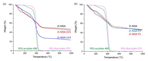
Fig. 4 TGA of (a) Zr-MSA, PEG-acylate-480, PEG-diacrylate-575, Zr-MSA-UV1 and Zr-MSA-UV2; (b) Zr-MSA, PEG-acylate-480, PEG-diacrylate-575, Zr-MSA-P1 and Zr-MSA-P2.
