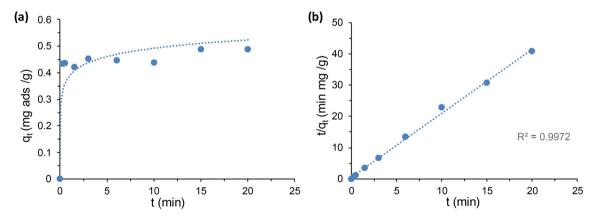
Fig. 6 (a) Hg(II) absorption kinetics of Zr-MSA-UV2 for 20 minutes contact. (b) The pseudo-second-order kinetic plot for the absorption (Hg(II) concentration of 10 mg  $L^{-1}$ ).
