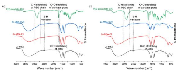
Fig. 2 FT-IR measurements of (a) PEG-acrylate-480, Zr-MSA-UV1, Zr-MSA-P1 and Zr-MSA; (b) PEG-diacrylate-575, Zr-MSA-UV2, Zr-MSA-UV2 and Zr-MSA.
