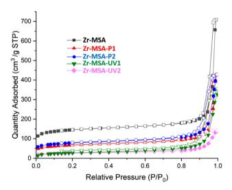
Fig. 3 N<sub>2</sub> adsorption-desorption isotherms measured at 77 K for pristine Zr-MSA, Zr-MSA-UV1, Zr-MSA-UV2, Zr-MSA-P1 and Zr-MSA-P2. Filled and empty symbols represent adsorption and desorption processes, respectively.
