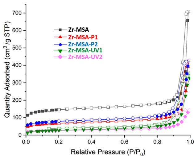
Fig. 3  $N_2$  adsorption-desorption isotherms measured at 77 K for pristine Zr-MSA, Zr-MSA-UV1, Zr-MSA-UV2, Zr-MSA-P1 and Zr-MSA-P2. Filled and empty symbols represent adsorption and desorption processes, respectively.
