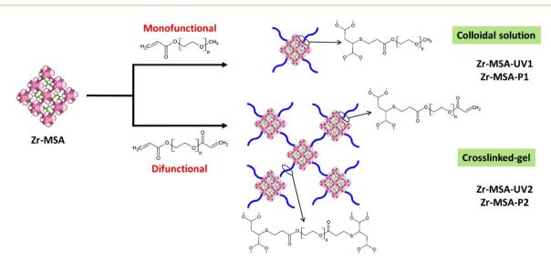
Scheme 1 PSM via thiol-ene click reactions used for the modification of Zr-MSA with PEG acrylates.
