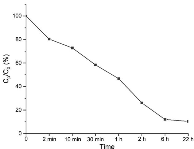
Fig. 7 Absorption of Cr(VI) on Zr-MSA-UV2 at pH3.
