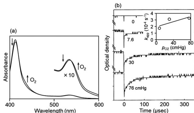
**Fig. 3** (a) Visible absorption spectra of the CoTPP–OIm membrane at 25 °C under oxygen at 0 and 7 atm. (b) Absorption recovery at 430 nm after laser flash irradiation at –15 °C, ascribed to the recombination reaction of the photo-dissociated oxygen to the CoTPP complex with OIm in the solid membrane state under an oxygen partial pressure of 0–76 cmHg. Inset: plots of apparent oxygen-binding rate constant ( $k_{app}$ ) vs. oxygen partial pressures at –15 °C.
