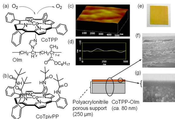
**Fig. 1** Chemical structures of (a) cobalt tetraphenylporphyrin (CoTPP) and poly(vinylimidazole-co-octyl methacrylate) (OIm), and (b) cobalt meso-tetra( $\alpha,\alpha,\alpha,\alpha$ -*o*-pivalamidophenyl)porphyrin (CoTpivPP). (c) and (d) Atomic force microscopy images of the CoTPP-OIm membrane on a porous support. (e) Photograph of the CoTPP-OIm membrane on the porous support. (f) and (g) Cross-sectional scanning electron microscopy images of the CoTPP-OIm membrane.
