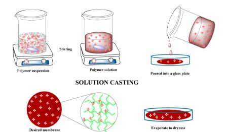
Fig. 8 Preparation of polymer membranes through solvent casting process. Reprinted with permission from ref. 95. Copyright MDPI 2017 (open access under CC-BY 4.0).
