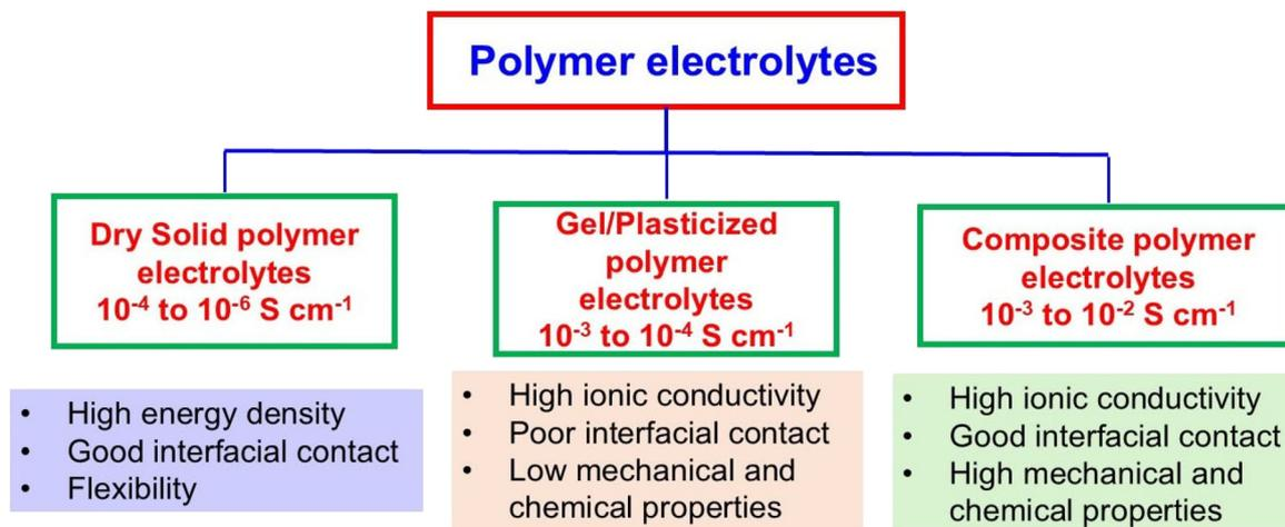
Fig. 3 Classification of polymer electrolytes and their properties.
