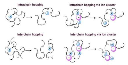
Fig. 17 Cartoon illustrating the ion transport in PEO SPE. Reprinted from ref. 133 with permission from the Royal Society of Chemistry.
