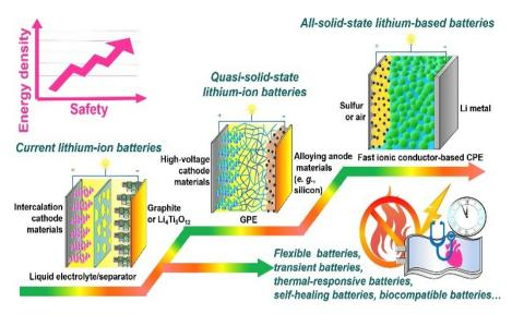
Fig. 2 History and evolution of polymer electrolytes. Reprinted with permission from ref. 33. Copyright Elsevier 2019 (license number: 5673190287905).
