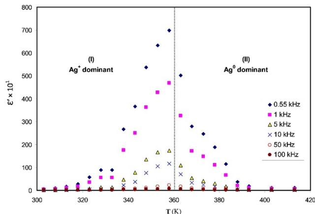
**Fig. 16** Temperature dependence of dielectric constant ( $\epsilon'$ ) at different frequencies for chitosan:AgTf (90:10) SPE. Reprinted with permission from ref. 127. Copyright Elsevier 2014 (license number: 5673210989263).
