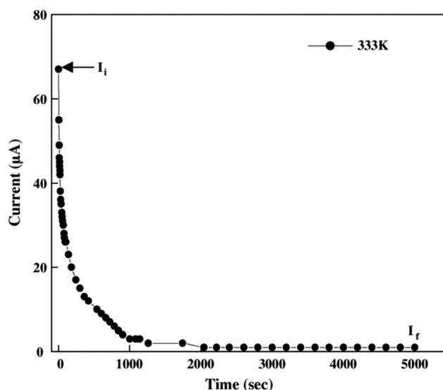
Fig. 22 Current vs. time plot of 71.25PVAc:23.75PVdF:5LiClO<sub>4</sub> polymer electrolyte at 333 K. Reused with permission from ref. 140.
