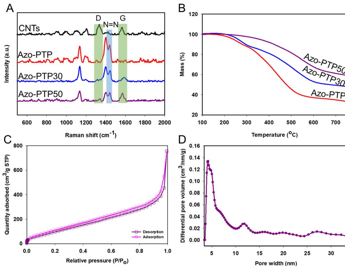
**Fig. 2** (A) Raman spectra of CNTs (black), Azo-PTP (red), Azo-PTP30 (blue), and Azo-PTP50 (purple), (B) thermogravimetric analysis curves (TGA) for Azo-PTP (red), Azo-PTP30 (blue), and Azo-PTP50 (purple), (C) N<sub>2</sub> sorption isotherm of Azo-PTP50 (77 K, pink = adsorption; purple = desorption), and (D) pore size distribution (calculated by DFT).
