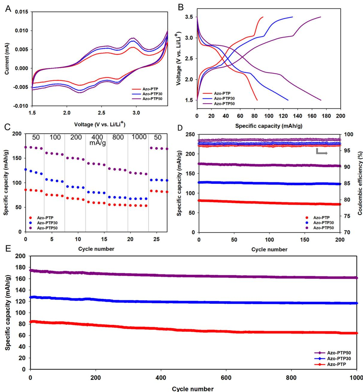
**Fig. 3** (A) Cyclic voltammograms (CVs) at a scan rate of  $0.1 \text{ mV s}^{-1}$ , (B) galvanostatic charge/discharge curves at  $50 \text{ mA g}^{-1}$ , (C) rate capability, (D) cycling stability at  $50 \text{ mA g}^{-1}$  for 200 cycles, and (E) long-term cycling stability at  $100 \text{ mA g}^{-1}$  for 1000 cycles of Azo-PTP (red), Azo-PTP30 (blue), and Azo-PTP50 (purple).
