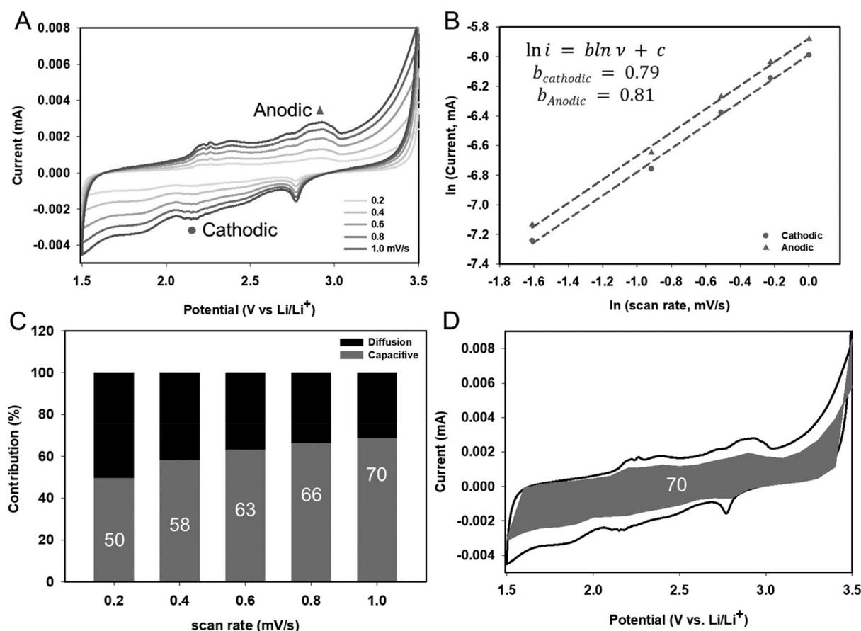
Fig. 5 (A) CV curves of Azo-PTP50 at different scan rates, (B) the corresponding plots  $\ln(i)$  versus  $\ln(v)$  at each redox peak, (C) contribution ratio of pseudocapacitance at various scan rates, and (D) capacitive contribution of Azo-PTP50 at a scan rate of  $1 \text{ mV s}^{-1}$ .
