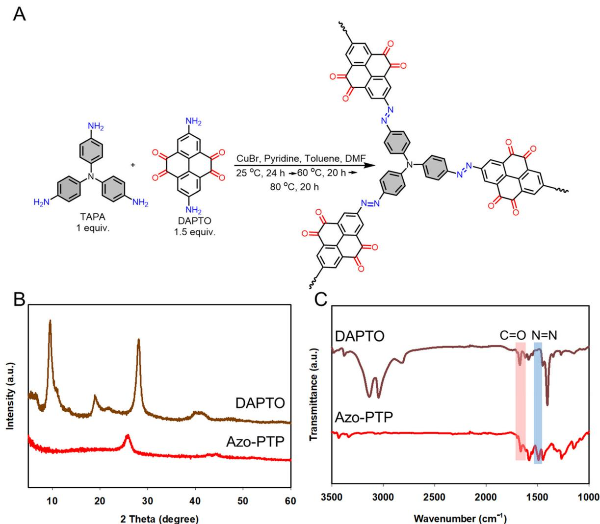
Fig. 1 (A) Synthetic scheme of the azo-linked pyrenetetraone polymer (Azo-PTP), (B) pXRD pattern, and (C) FTIR spectra of DAPTO (brown) and Azo-PTP (red).
