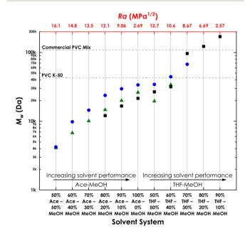
Fig. 4 Weight average molecular weight ( $M_{w_r}$  log scale) of ( $\triangle$ ) PVC K-50 single-step, ( ) PVC K-50 sequential and ( ) commercial PVC sequential fractionations in different solvent systems. Bottom X: content of solvent systems. Top X: Hansen solubility parameters (HSPs) distance  $R_a$  (MPa<sup>1/2</sup>) of corresponding solvent system (Bottom X).
