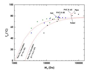
Fig. 6  $T_{\rm g}$  values measured using DSC for  $\triangle$  single-step PVC K-50 fractions, **o** sequential PVC K-50 fractions, **o** is sequential commercial PVC fractions,  $\frac{1}{3}$  other samples (individually labeled). - - Predicted  $T_{\alpha}$  values using the Flory-Fox equation.
