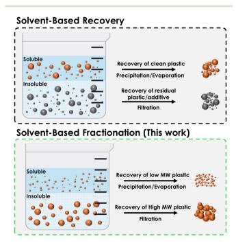
Fig. 3 Comparison between solvent-based recovery of "whole" plastic and solvent-based fractionation of specific plastic "grades". Note that the recovery method can be reversed, with the recovered material being the insoluble (in fractionation terminology, recovery of the soluble = solvent extraction, recovery of the insoluble = fractional precipitation).
