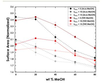
Fig. 7 Ratio of surface area for PVC in Ace-MeOH and THF-MeOH blends at different MeOH % and at different  $n_{PVC}$ .
