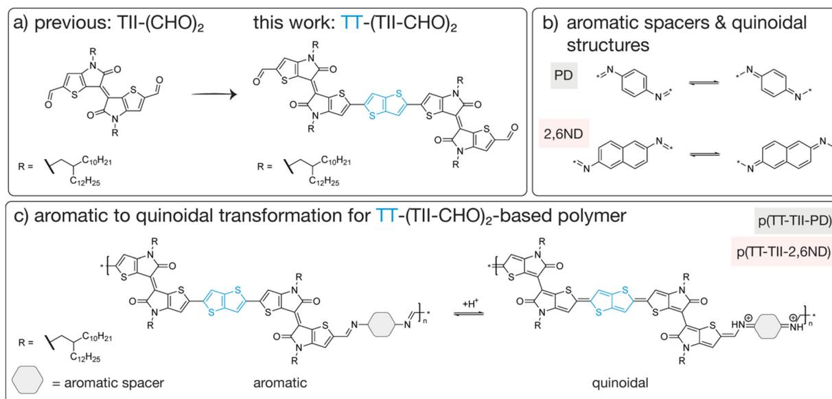
**Fig. 1** (a) Overview of previous work vs. this work focusing on the TT unit inserted TII dimer structure bearing aldehyde groups. (b) Aromatic spacers PD and 2,6ND used in this work and their quinoidal structures. (c) Aromatic to quinoidal transformation via acid-mediated protonation for polymers p(TT-TII-PD) and p(TT-TII-2,6ND).
