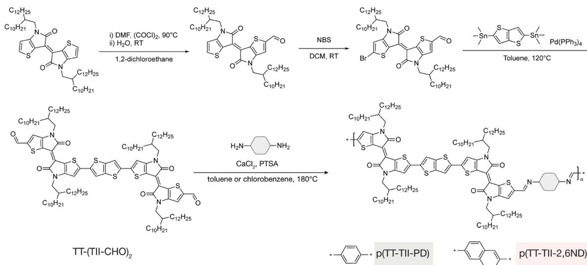
**Fig. 2** Synthetic scheme of TT-(TII-CHO)<sub>2</sub> and target polymers p(TT-TII-PD) and p(TT-TII-2,6ND).
