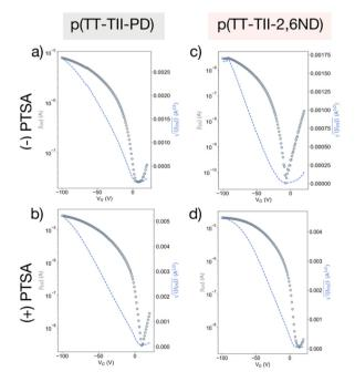
Fig. 4 Typical transfer curves of pristine ((-)PTSA) and protonated ((+) PTSA) thin films: (a) pristine p(TT-TII-PD), (b) protonated p(TT-TII-PD), (c) pristine p(TT-TII-2,6ND), and (d) protonated p(TT-TII-2,6ND).
