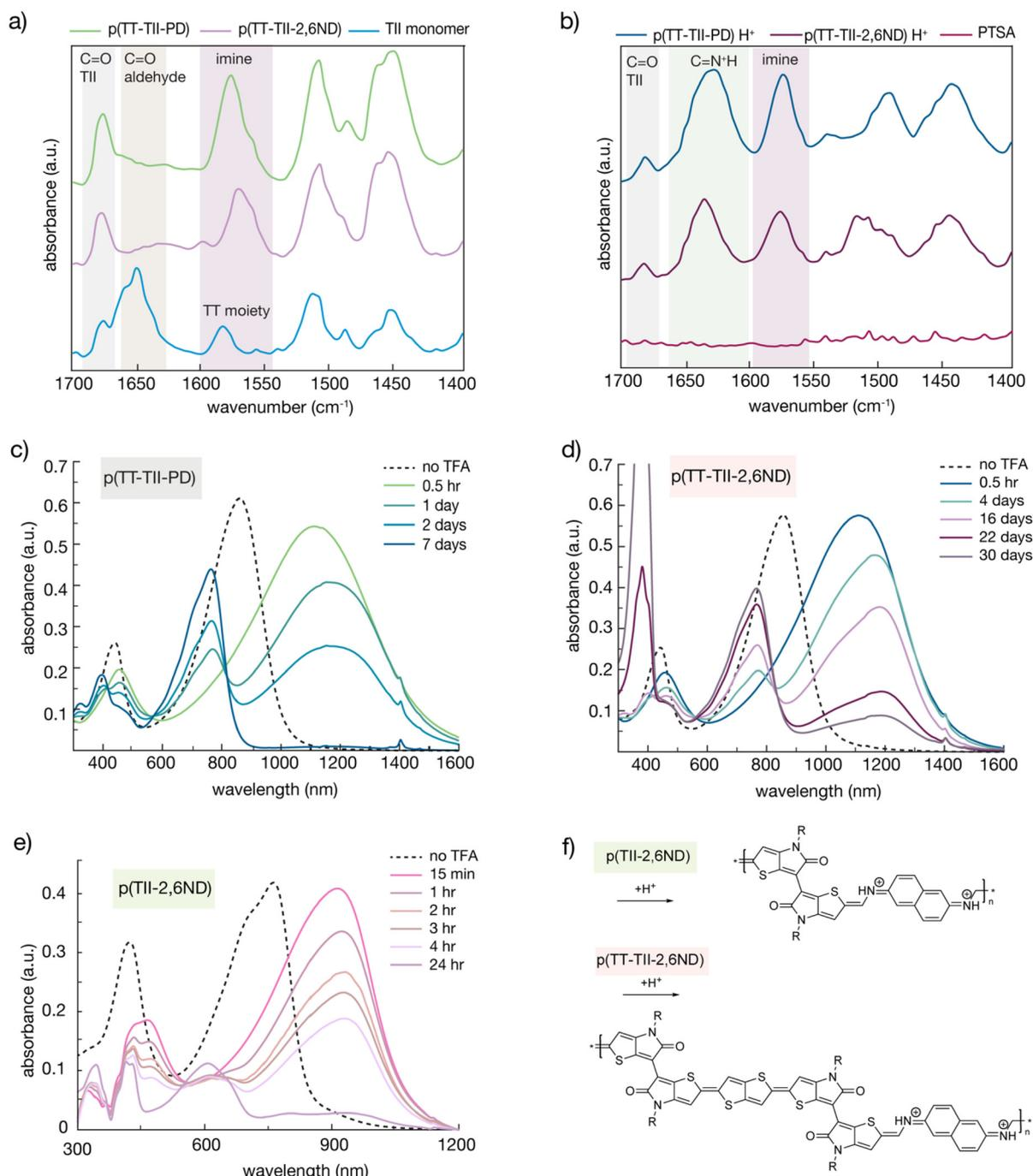
**Fig. 3** Evidence of quinoidal structure improving chemical stability. Infrared spectroscopy (IR) on (a) pristine and protonated p(TT-TII-PD) and (b) pristine and protonated p(TT-TII-2,6ND). Time-dependent UV-vis-NIR absorption profiles for (c) p(TT-TII-PD), (d) p(TT-TII-2,6ND) and (e) p(TII-2,6ND). (f) Results of DFT calculations showing coplanarity of pristine and protonated model compound based on p(TT-TII-2,6ND).
