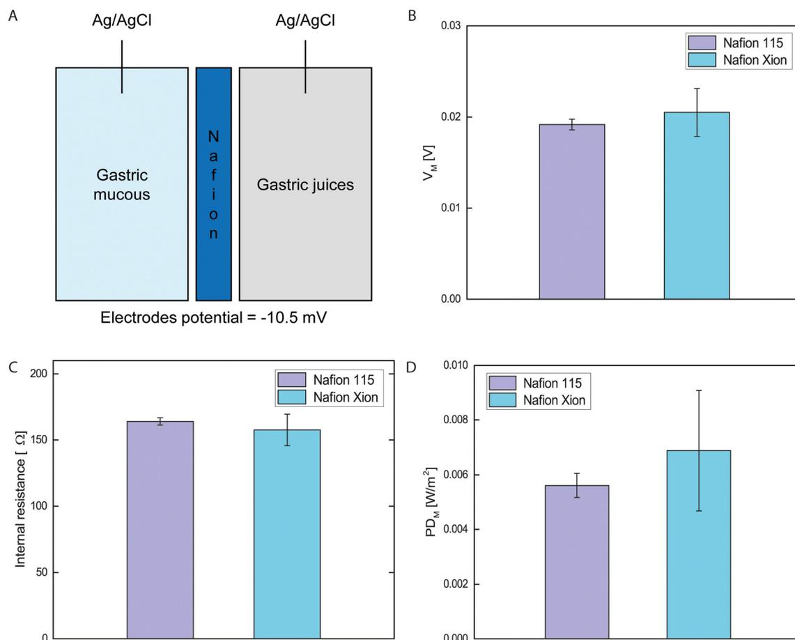
**Fig. 2** (A) Schematic representation of the cell used to measure the voltage across Nafion membranes using gastric juices as ion-rich solution and gastric mucous as ion-poor solution. (B–D) Comparison of the (B) membrane potentials, (C) internal resistance, and (D) power density (from eqn (4)) obtained with Nafion® 115 and Xion with the setup reported in A.
