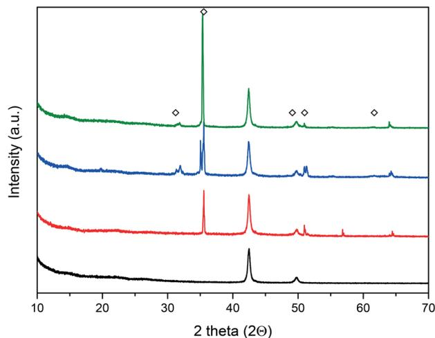
**Fig. 2** XRD patterns of the various steps involved in forming the lithium hydroxide layer. Commercial lithium metal surface (red trace), LiOH layer formation after reaction with water vapor (blue trace), and after thermal treatment to obtain the anhydrous LiOH layer (green trace). The black trace is the background signal of the Kapton sample holder. The diamond symbols represent the scattering angles of the lithium hydroxide layer.
