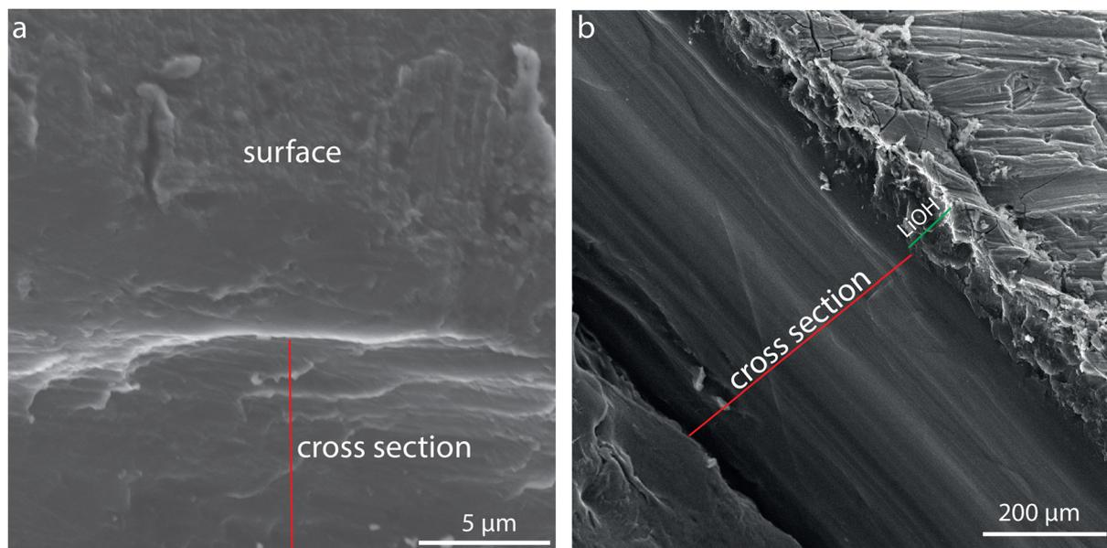
**Fig. 3** Cross-sectional SEM images of an as-received lithium metal substrate (a) and after forming a LiOH layer (b). The red line marks the cross-section, and the green line indicates the LiOH layer.
