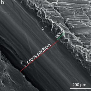
Fig. 3 Cross-sectional SEM images of an as-received lithium metal substrate (a) and after forming a LiOH layer (b). The red line marks the crosssection, and the green line indicates the LiOH layer.
