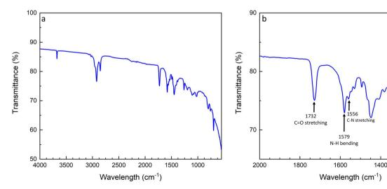
Fig. 5 FT-IR spectra of the P(S-*r*-MMA) isocyanate reaction to the lithium hydroxide substrate (a) and zoom into the amide characterization region to confirm the conversion reaction (b).
