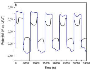
Fig. 9 Galvanostatic cycling traces of pristine lithium electrode (black trace) and P(S-r-MMA)-covered lithium electrode (blue trace) at a current of 0.095 mA (0.047 mA cm $^{-2}$ ) (a) and 0.19 mA (0.095 mA cm $^{-2}$ ) (b).
