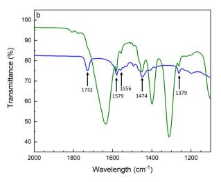
Fig. 10 FT-IR spectra of the P(S-r-MMA)-covered lithium substrate before (blue trace) and after (green trace) galvanostatic cycling (a). The zoom into the amide region (b) shows the peaks marked with arrows corresponding to the amides I, II, and III.
