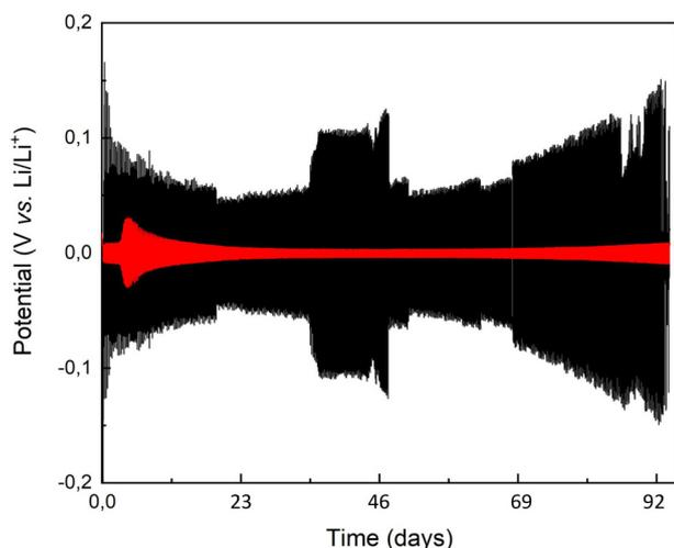
**Fig. 4** Galvanostatic cycling of symmetrical pristine (black trace) and lithium hydroxide covered (red trace) electrodes, using the EC-DMC liquid electrolyte, at ambient temperature with a constant current density of 0.2 mA (0.1 mA cm<sup>-2</sup>).
