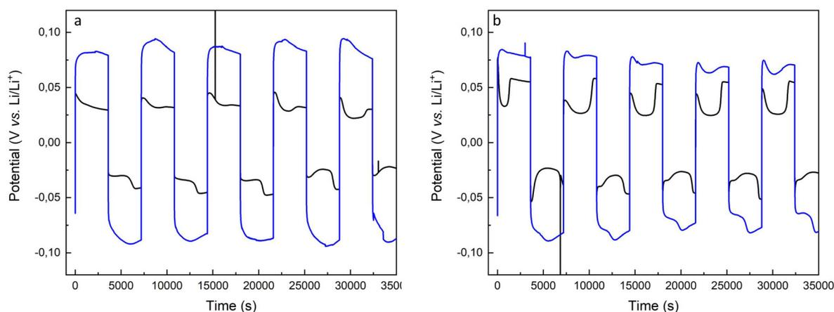
Fig. 9 Galvanostatic cycling traces of pristine lithium electrode (black trace) and P(S-*r*-MMA)-covered lithium electrode (blue trace) at a current of 0.095 mA (0.047 mA cm<sup>-2</sup>) (a) and 0.19 mA (0.095 mA cm<sup>-2</sup>) (b).
