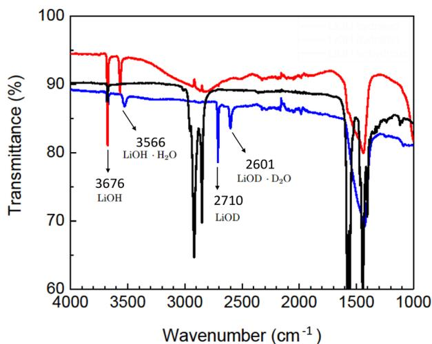
**Fig. 1** FT-IR spectra of lithium hydroxide on lithium metal substrates after reaction with hydrogenated (red trace) and deuterated (blue trace) water, and the anhydrous LiOH layer after thermal treatment (black trace).
