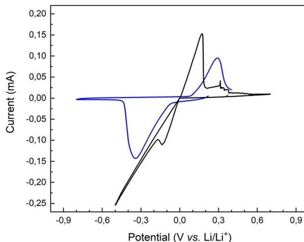
**Fig. 7** Cyclic voltammetry traces of a pristine lithium surface (black trace) and a P(S-*r*-MMA)-covered lithium substrate (blue trace).
