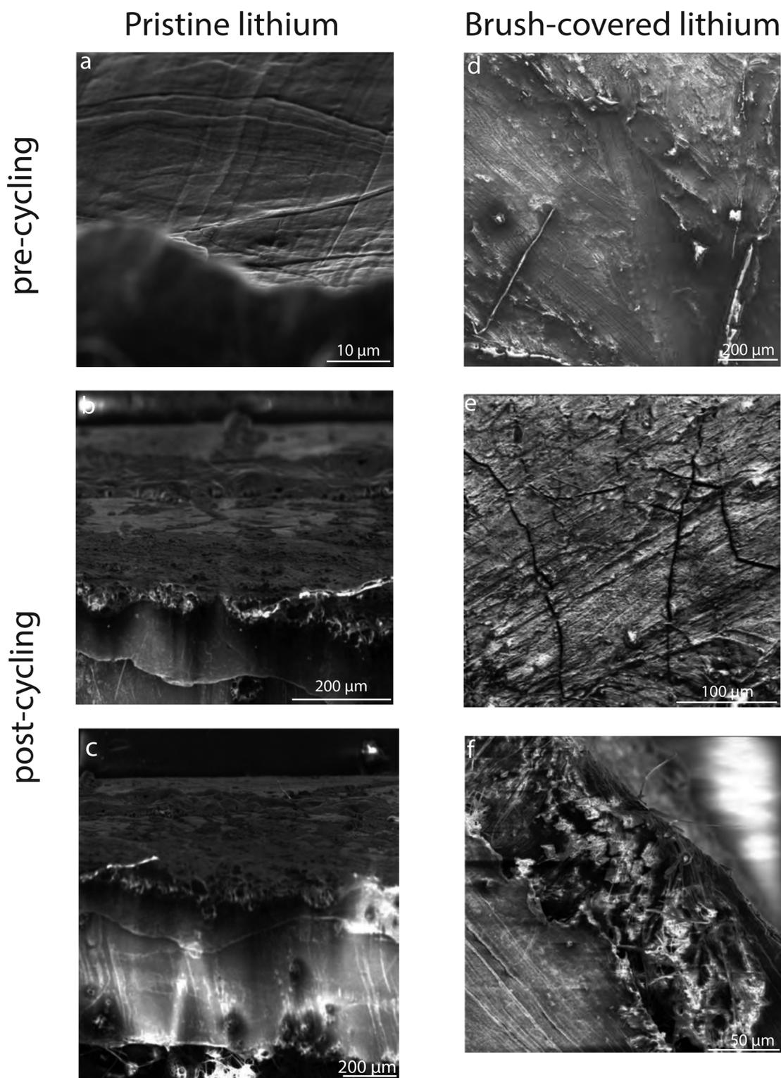
**Fig. 11** SEM images of pristine lithium surfaces, pre-cycling (a), post-cycling (b), and cross-section (c). P(S-*r*-MMA) brush-covered lithium surfaces, pre-cycling (d), surface post-cycling (e), and cross-section (f).
