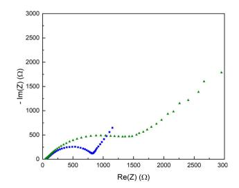
Fig. 8 Nyquist plot of the P(S-r-MMA) copolymer covered lithium substrate before (blue squares) and after (green triangles) electrochemical cycling.
