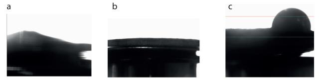
Fig. 6 Contact angle images of a water droplet placed on a pristine metallic lithium surface (a) and the P(S-r-MMA) copolymer brush-coated lithium surface (c), demonstrating its improved stability. For reference, the P(S-r-MMA) copolymer coated lithium surface is shown without a water droplet (b).
