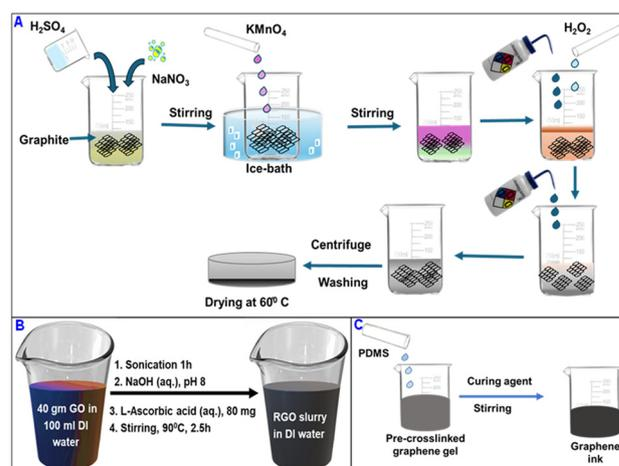
**Fig. 1** The modified Hummers' method (A) has been adapted to synthesize GO whereas the process for synthesizing reduced graphene oxide (B) from GO is schematically shown in B and the formulation of the graphene-based ink recipe has been described in C.
