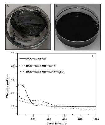
Fig. 4 The images of the hydroxyl PDMS crosslinked rGO gel (A) and the corresponding ink (B) after adding PDMS and the curing agent. The rheological studies of different variants of rGO-reinforced materials are represented in C.
