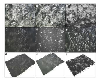
Fig. 7 The optical images of the printed layers using 15% rGO inks on Kevlar (A), fiberglass (B), and polyester (C) cloths respectively. The surface and 3D topographic images of films were obtained by printing 10% (D & G), 15% (E & H), and 20% (F & I) rGO-based inks where the scale bar is 150 µm.
