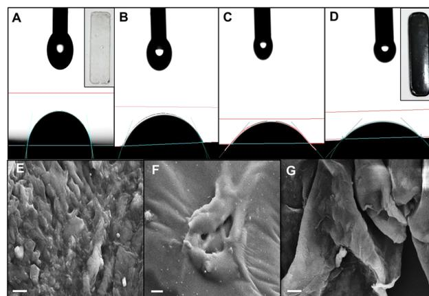
**Fig. 5** The water contact angles of the rGO-based film of PDMS (A), 10% (B), 15% (C), and 20% (D) loading are observed to be 80°, 61.1°, 52.1°, and 41.9° whereas the actual free-standing PDMS and nanocomposite film are shown in the inset of the figure. The cross-sectional SEM images of film 10% (E), 15% (F), and 20% (G) loadings are presented (scale bar is 1 μm) in Fig. E–G.
