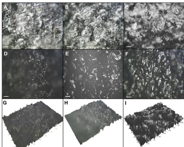
**Fig. 7** The optical images of the printed layers using 15% rGO inks on Kevlar (A), fiberglass (B), and polyester (C) cloths respectively. The surface and 3D topographic images of films were obtained by printing 10% (D & G), 15% (E & H), and 20% (F & I) rGO-based inks where the scale bar is 150  $\mu\text{m}$ .
