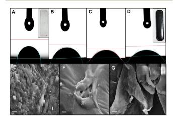
The water contact angles of the rGO-based film of PDMS (A), 10% (B), 15% (C), and 20% (D) loading are observed to be 80°, 61.1°, 52.1°, and 41.9° whereas the actual free-standing PDMS and nanocomposite film are shown in the inset of the figure. The cross-sectional SEM images of film 10% (E), 15% (F), and 20% (G) loadings are presented (scale bar is  $1 \mu m$ ) in Fig. E-G.
