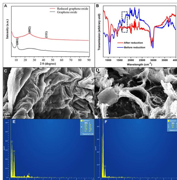
**Fig. 3** X-ray diffraction patterns (A), FT-IR spectra (B) before and after reduction of graphene oxide, scanning electron microscopy images (C and D), and energy dispersive X-ray analysis results (E and F) of the developed GO and rGO samples.
