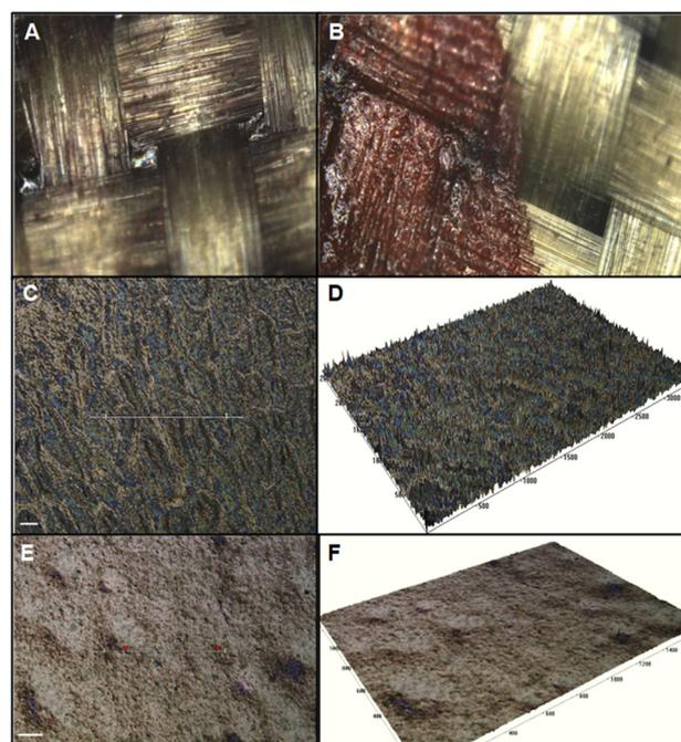
**Fig. 6** The 3D optical images of the non-contact mode of the back side of the printed layers on 75 (A) and 300 (B) grams per square metre (GSM) Kevlar fabric. The surface (C and E) and topographic (D and F) images of the printed textile surface before and after annealing respectively where the scale bar is 150  $\mu\text{m}$ .
