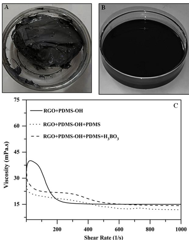
**Fig. 4** The images of the hydroxyl PDMS crosslinked rGO gel (A) and the corresponding ink (B) after adding PDMS and the curing agent. The rheological studies of different variants of rGO-reinforced materials are represented in C.
