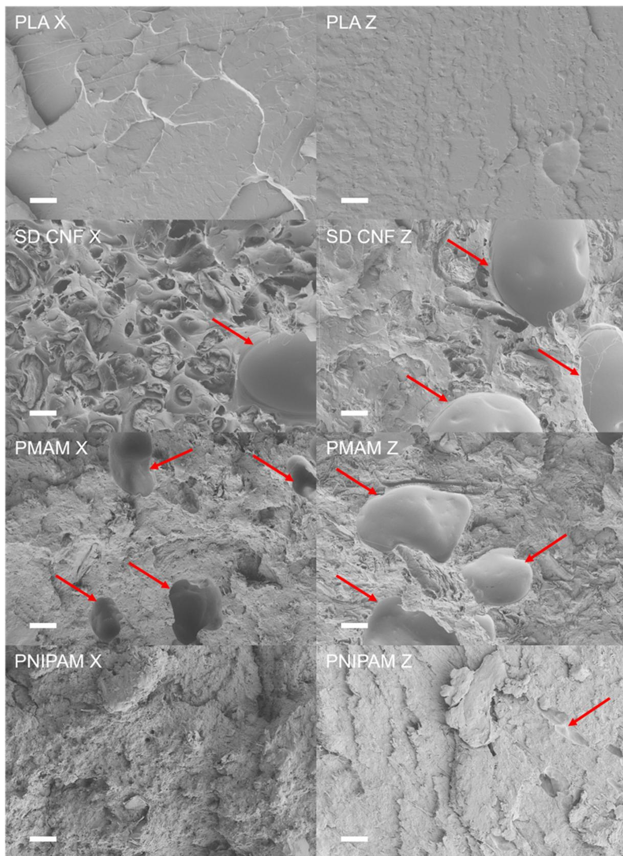
**Fig. 6** SEM images of x- and z-directional fracture surfaces for printed composite samples. All images are at 500x magnification with scale bars of 20 μm. Red arrows point to apparent voids in the composite matrix.
