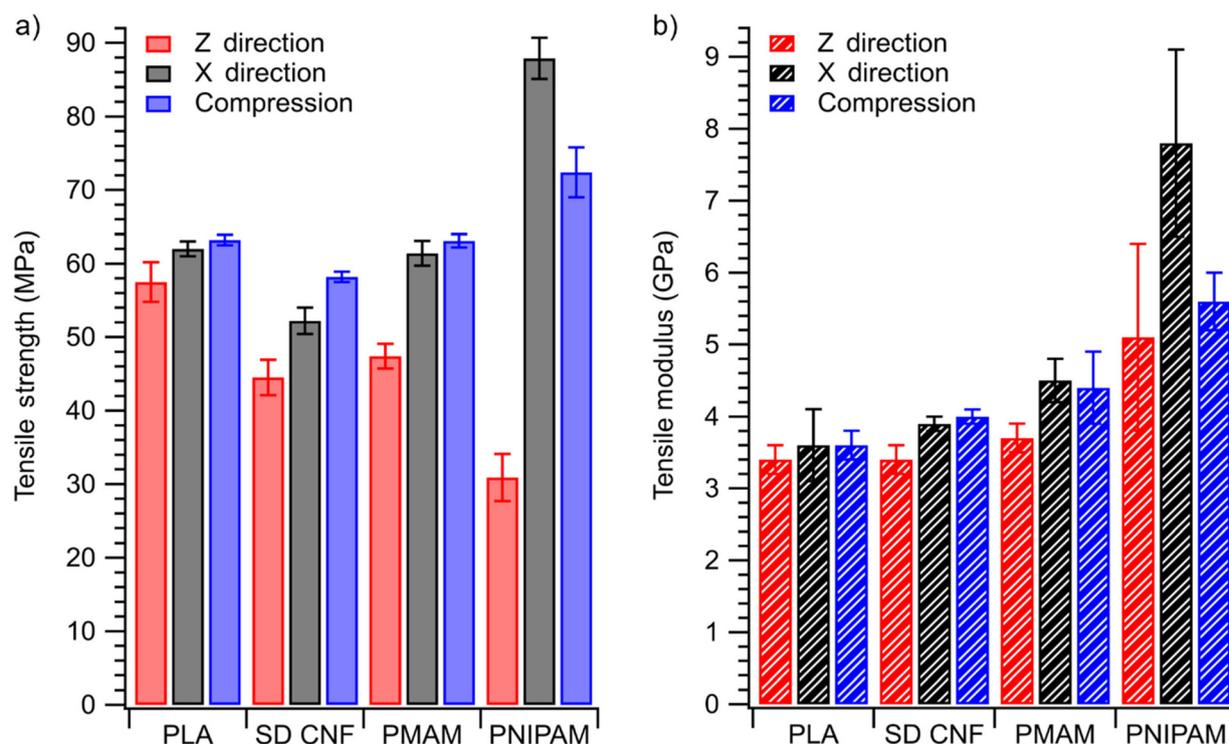
Fig. 5 (a) Tensile strength and (b) tensile modulus of elasticity of 3D printed samples milled along the bead direction (*x* direction) and across the interlayer direction (*z* direction) with compression-moulded isotropic samples of the pellets used for 3D printing. Values are averages, with error bars indicating 95% confidence intervals.
