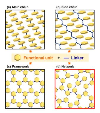
Fig. 1 Organizational states of functional molecules. (a) Main-chain type. (b) Side-chain type. (c) Crystalline framework. (d) Amorphous CPN.
