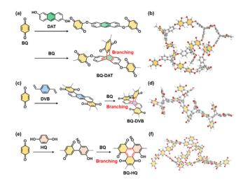
Fig. 12 Molecular design of amorphous CPNs containing redox-active BQ moieties. (a and b) BQ-DAT. (c and d) BQ-DVB. (e and f) BQ-HQ. Reproduced from ref. 9 with permission from the Royal Society of Chemistry
