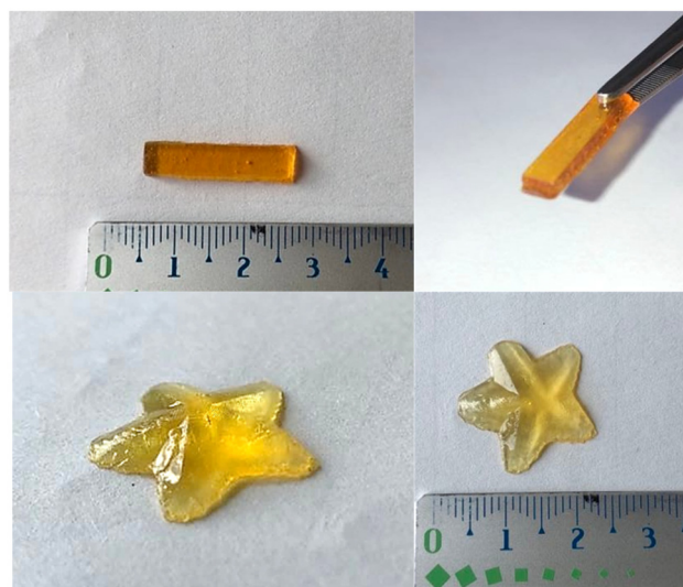
Fig. 8 3D photo-printing of a star and a rod with the TT/Lin/SOA (25%/25%/50% w/w) formulation with P-3Ac (0.5 wt%) using DLP technology upon 405 nm light emitting diode exposure. Dimensions of the star: x = 15.129 \text{ mm} , y = 16.469 \text{ mm} and z = 2.953 \text{ mm} . Dimensions of the rod: x = 30.40 \text{ mm} , y = 9.80 \text{ mm} and z = 2.58 \text{ mm} .
