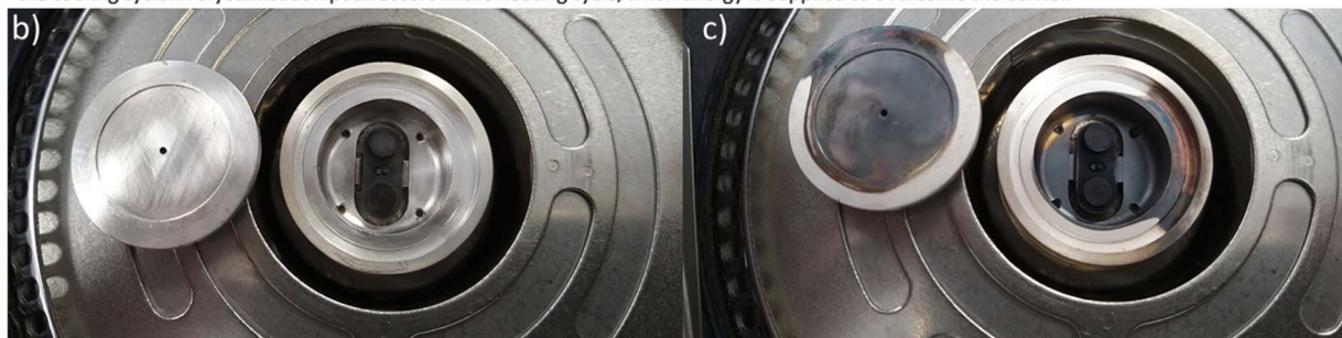
Fig. 14 (a) An annotated diagram of a DSC thermogram of a typical inverse vulcanised polymer, showing all the major features to expect. Note that this is not the thermogram of a real inverse vulcanised polymer. 32–37,75–89,101 (b) A clean DSC cell and lid, made of silver metal. (c) A DSC cell and lid where a sample pan has ruptured, leaking inverse vulcanised polymer into the cell, causing the inverse vulcanised polymer to react with the silver metal to form silver sulfide. This requires the cell to be filed down to remove the silver sulfide, which in turn requires full baseline conditioning and cell calibration.
