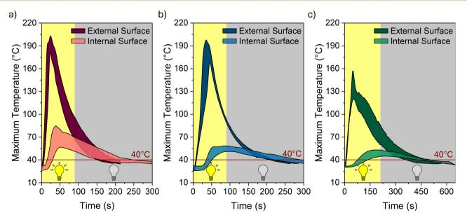
Fig. 4 Maximum temperatures measured on the external and internal surface during the curing through LED lamp of (a) a cylindrical single-layer composite with the insulation level #A; (b) cylindrical single-layer composite with the insulation level #B; (c) cylindrical double-layer composite with the insulation level #B.
