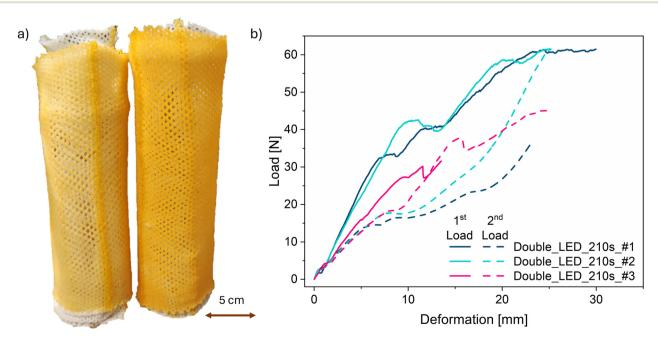
Fig. 3 (a) Picture of 2.1 T67/2 ITX double-layer composites; (b) load vs. deformation of the cured cylindrical double-layer composites irradiated with LED lamp, including multiple testing.
