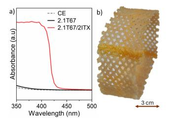
Fig. 1 (a) UV-visible spectra of CE-based formulation with and without additives; (b) picture of a 2.1 T76/2 ITX composite cylindrical sample with a net's stretching of +80%.
