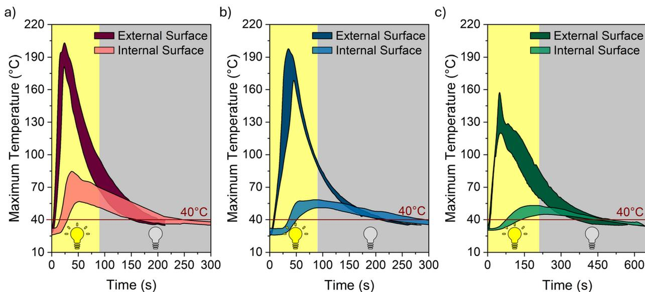
**Fig. 4** Maximum temperatures measured on the external and internal surface during the curing through LED lamp of (a) a cylindrical single-layer composite with the insulation level #A; (b) cylindrical single-layer composite with the insulation level #B; (c) cylindrical double-layer composite with the insulation level #B.
