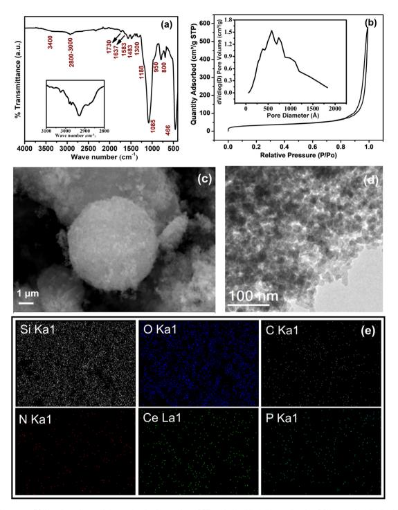
Fig. 5 (a) IR spectra, (b) N<sub>2</sub> adsorption and desorption isotherms from BET analysis with the inset showing BJH pore size distribution, (c) SEM image, (d) TEM image and (e) SEM elemental mapping of fCP-SiO<sub>2</sub>.
