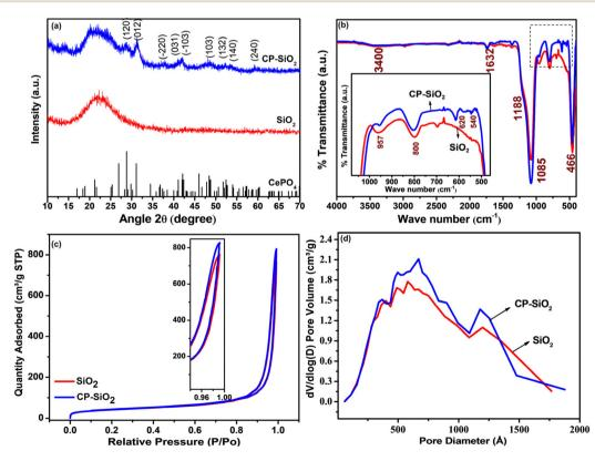
Fig. 2 (a) PXRD pattern, (b) IR spectra, (c) N<sub>2</sub> adsorption and desorption isotherms from BET analysis and (d) BJH pore size distribution of silica and hybrid pigment CP-SiO<sub>2</sub>
