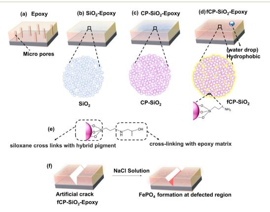
Fig. 10 Schematic representation of (a-d) bare epoxy, SiO<sub>2</sub>, CP-SiO<sub>2</sub> and fCP-SiO<sub>2</sub> loaded epoxy coatings. (e) Bonding of APS with the pigment and epoxy matrix, and (f) FePO<sub>4</sub> formation in the defect region.
