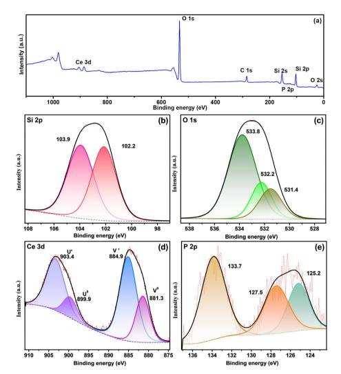
Fig. 3 XPS spectra of CP-SiO<sub>2</sub> (a) and survey and high-resolution spectra of (b) Si 2p, (c) O 1s, (d) Ce 3d and (e) P 2p.
