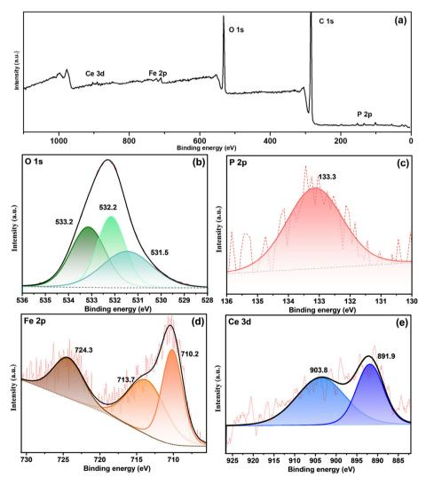
Fig. 9 XPS curve fitting of (a) the survey spectrum. (b) O 1s, (c) P 2p, (d) Fe 2p and (e) Ce 3d of the inhibitive film beneath the CP-SiO<sub>2</sub> loaded epoxy coating on steel depart from the 3.5 wt% NaCl solution.
