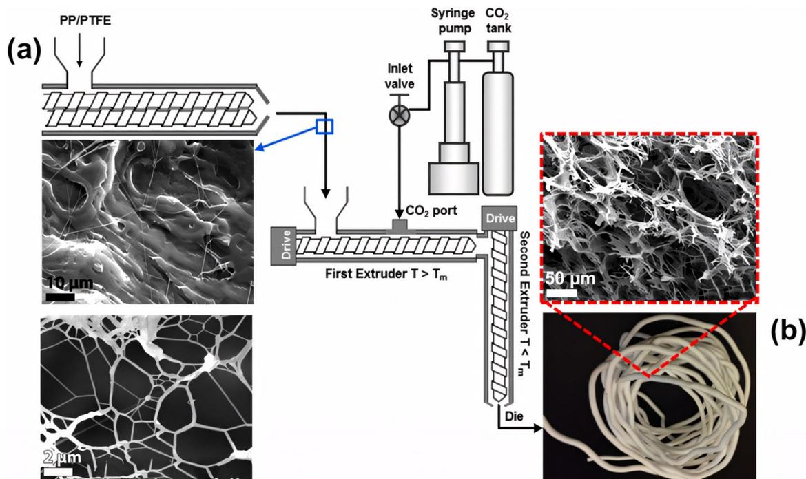
Fig. 7 Extrusion foaming of PP/PTFE fibrillar blends: (a) PP-homopolymer blended with PTFE in a twin-screw extruder; (b) images of an open-cell foam filament produced *via* extrusion. (Reproduced from ref. 91, Copyright 2014 American Chemical Society.)
