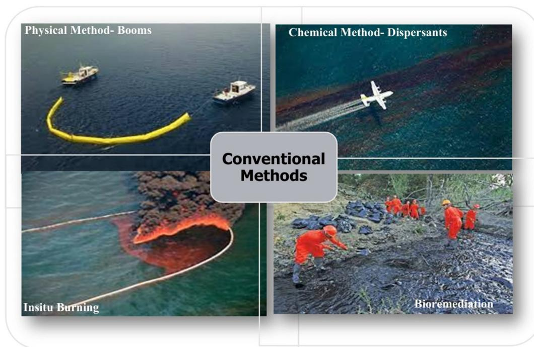
Fig. 2 The conventional oil spill remediation methods. (Reproduced from ref. 8. Copyright 2022 Elsevier Inc.)
