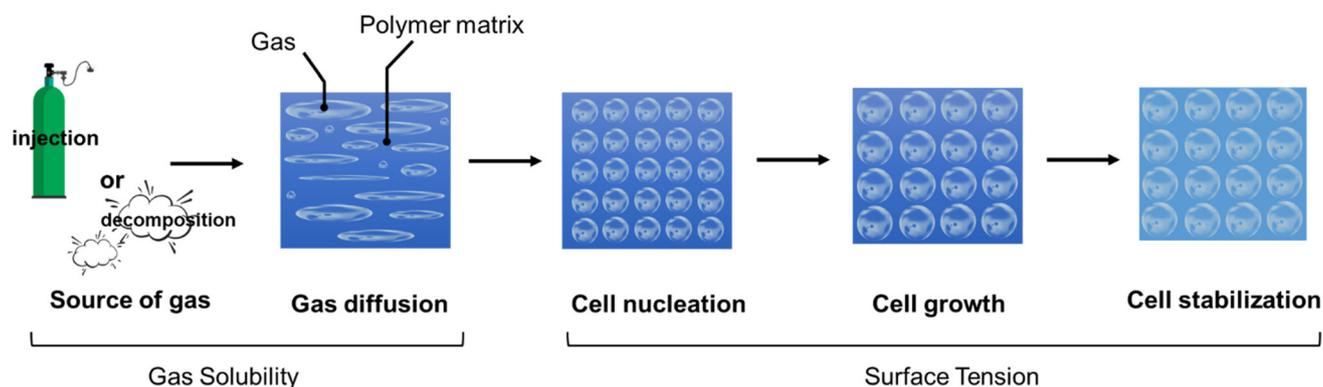
Fig. 5 Cell-formation procedure of polymeric foam.
