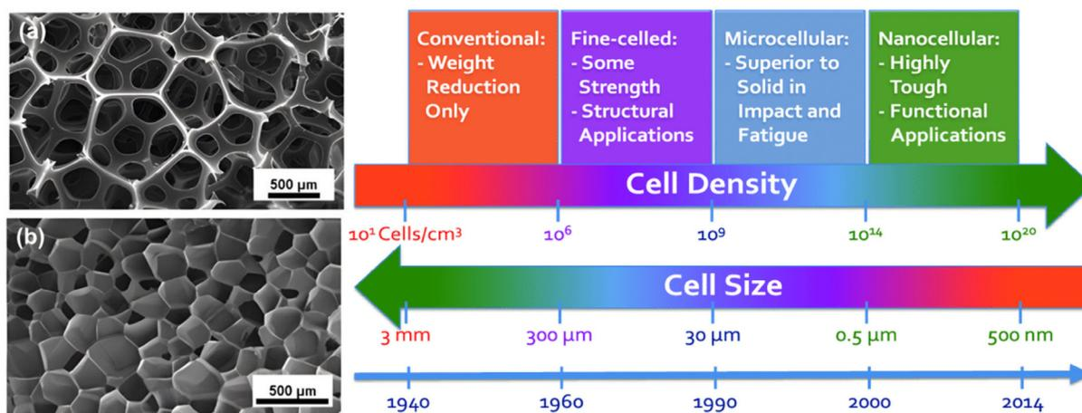
Fig. 4 (a) Open-cell<sup>59</sup> and (b) closed-cell<sup>60</sup> structures of polymeric foams; (c) cell sizes and cell density of the developed foams over time.<sup>66</sup> (Reproduced from ref. 59, 60 and 66. Copyright 2004 and 2005 Elsevier Inc.)
