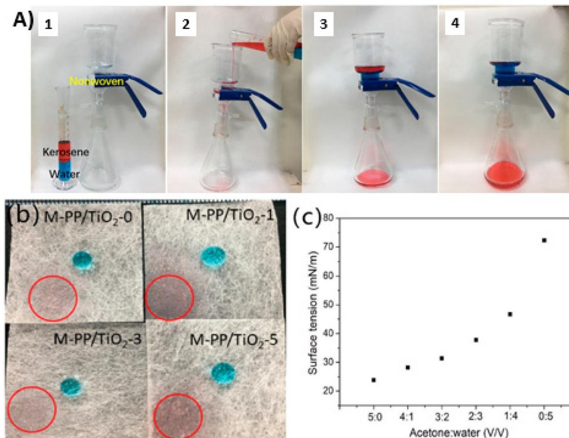
Fig. 17 (a) The oil–water separation process of M-PP/ $\text{TiO}_2$ , (b) the oil and water drip on the melt-blown membrane (the red circle is kerosene, the blue drop is water), and (c) the surface tension of different acetone solutions. Reproduced from ref. 193, Copyright 2019 MDPI.
