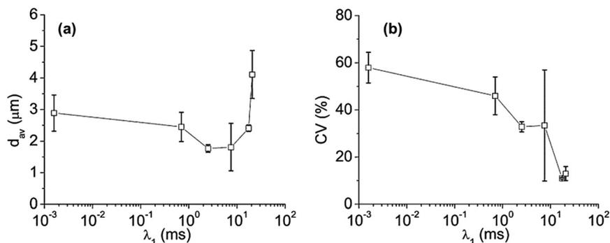
Fig. 14 (a) Average diameter ( $d_{\text{av}}$ ) and (b) coefficient of variation (CV) of melt-blown polystyrene fibers at approximately constant viscosities. Reproduced from ref. 179. Copyright 2010 Elsevier Inc.
