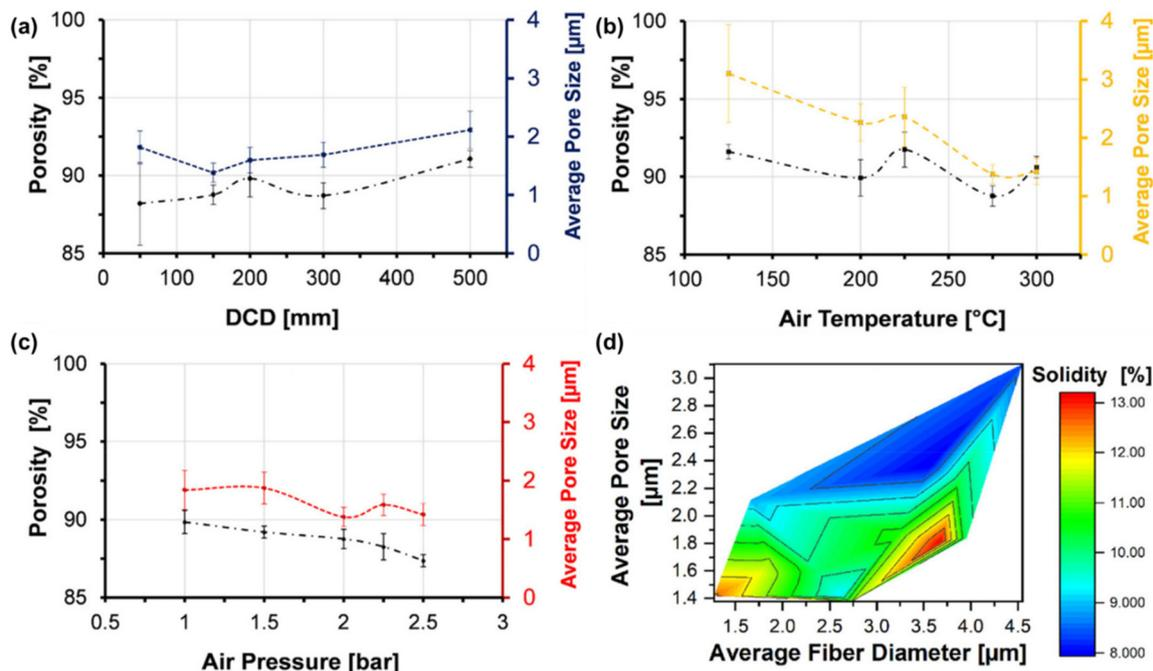
**Fig. 15** Porosity and pore size of PP melt-blown fibers as a function of (a) die-to-collector distance, (b) air temperature, (c) air pressure; (d) 2D contour plot of fiber solidity and pore size as a function of fiber diameter. (Reproduced from ref. 174. Copyright 2021 John Wiley & Sons, Inc.)
