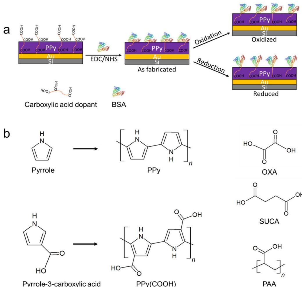
**Fig. 1** (a) Illustration of the route of immobilization of BSA on the PPy surface and the presentation change of BSA in different redox states of PPy; (b) structure of pyrrole, PPy, pyrrole-3-carboxylic acid, and PPy(COOH), and the dopants used for electropolymerized PPy: oxalic acid (OXA), succinic acid (SUCA), and poly(acrylic acid) (PAA).
