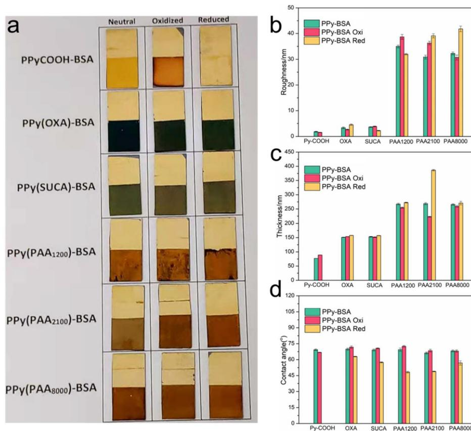
**Fig. 6** (a) Photographs of PPy-BSA films in different redox states. The physical properties, (b) roughness, (c) thickness, and (d) wettability in different redox states. Note: PPy-BSA (as-fabricated/non-stimulated) gave the same results as shown in Fig. 4. Data represent mean  $\pm$  standard deviation.
