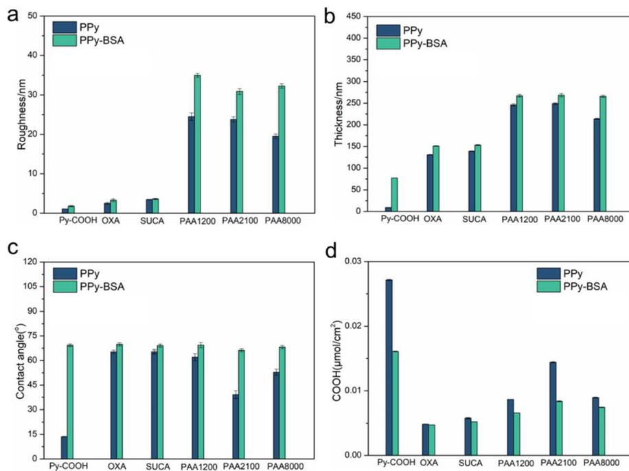
**Fig. 4** Surface characterization of PPY and PPY-BSA films. (a) roughness ( $R_a$ ), (b) thickness, (c) water contact angle, and (d) TBO staining results. Data represent mean  $\pm$  standard deviation.
