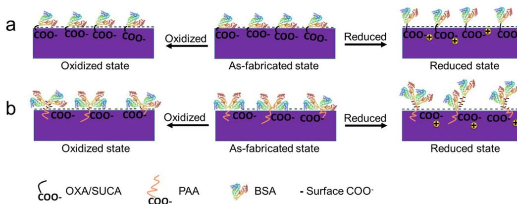
**Fig. 7** A schematic illustration of the BSA presentation in different redox states. (a) BSA presentation and the number of exposed  $\text{COO}^-$  on redox PPy(OXA) and PPy(SUCA) surfaces; (b) BSA presentation and the number of exposed  $\text{COO}^-$  on the redox PPy(PAA) series surface.
