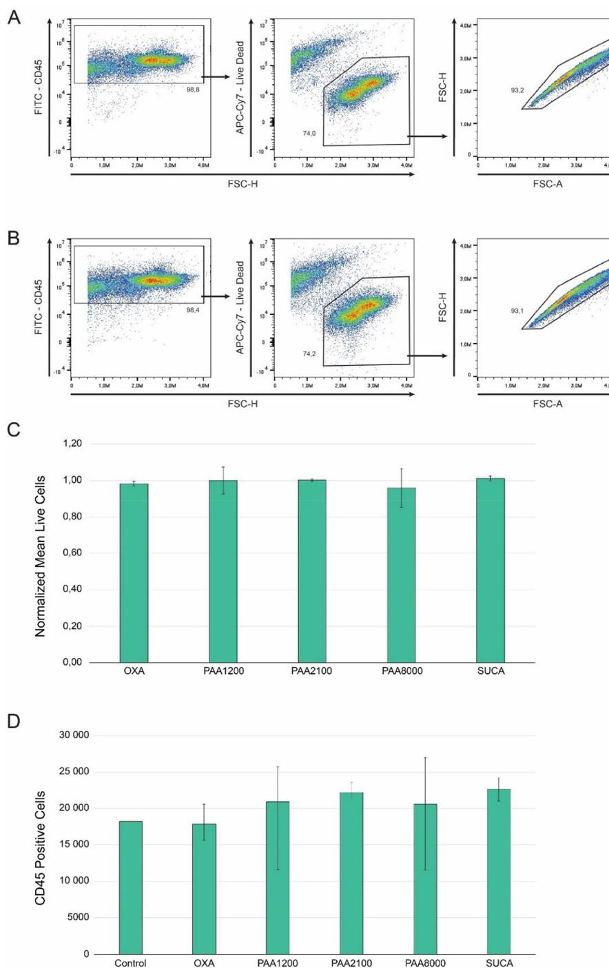
**Fig. 11** Cell viability after 48-hour incubation. Representative gating of live CD45<sup>+</sup> cells in (A) control samples, and (B) PPy-BSA surfaces. (C) Cell viability normalized to the control. (D) Live CD45<sup>+</sup> c-KIT<sup>+</sup> hematopoietic cell number. Data in bar charts represent mean  $\pm$  standard deviation.
