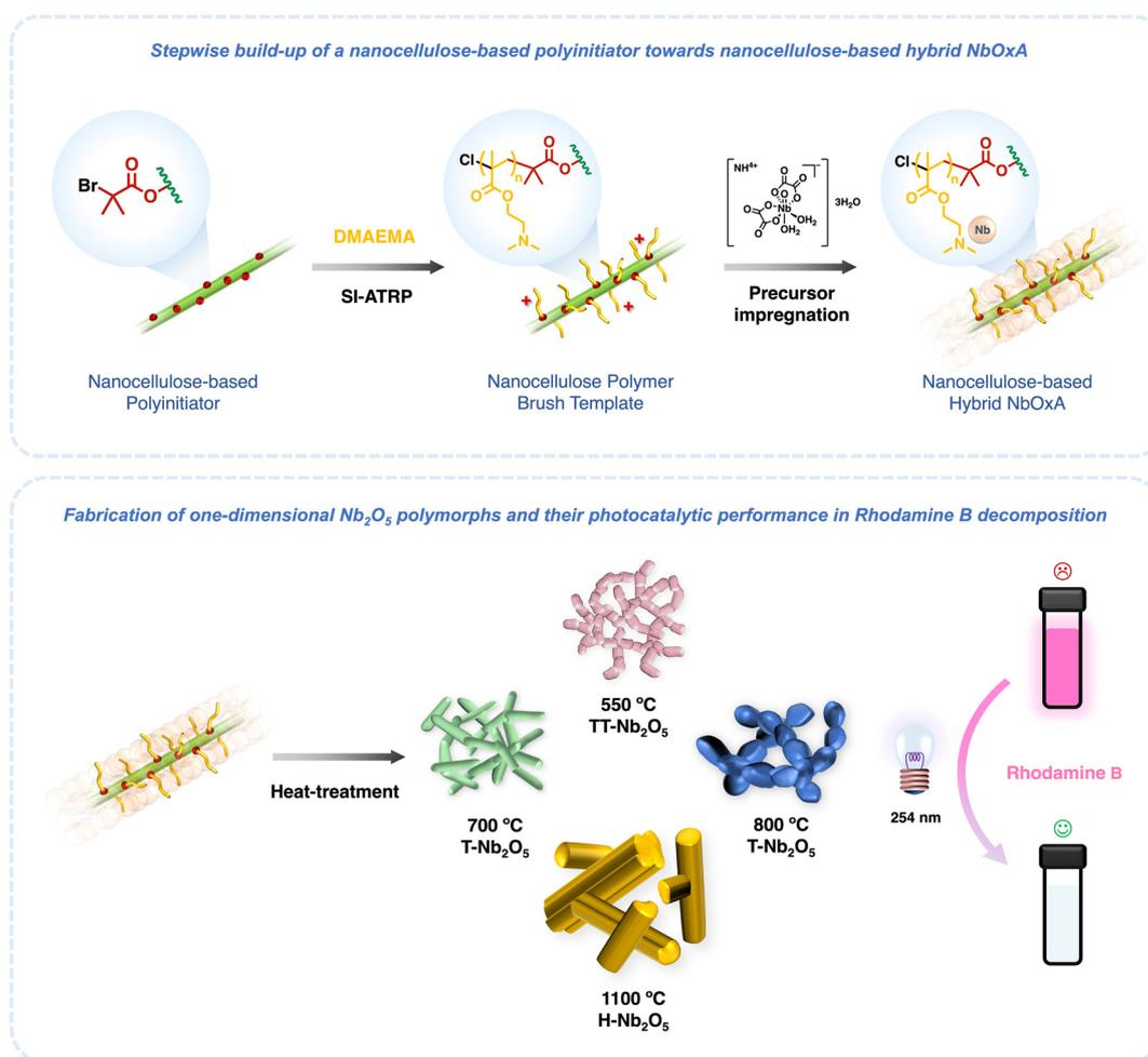
**Scheme 1** Template-directed fabrication of Nb<sub>2</sub>O<sub>5</sub> polymorphs using nanocellulose-based polymer brush templates.
