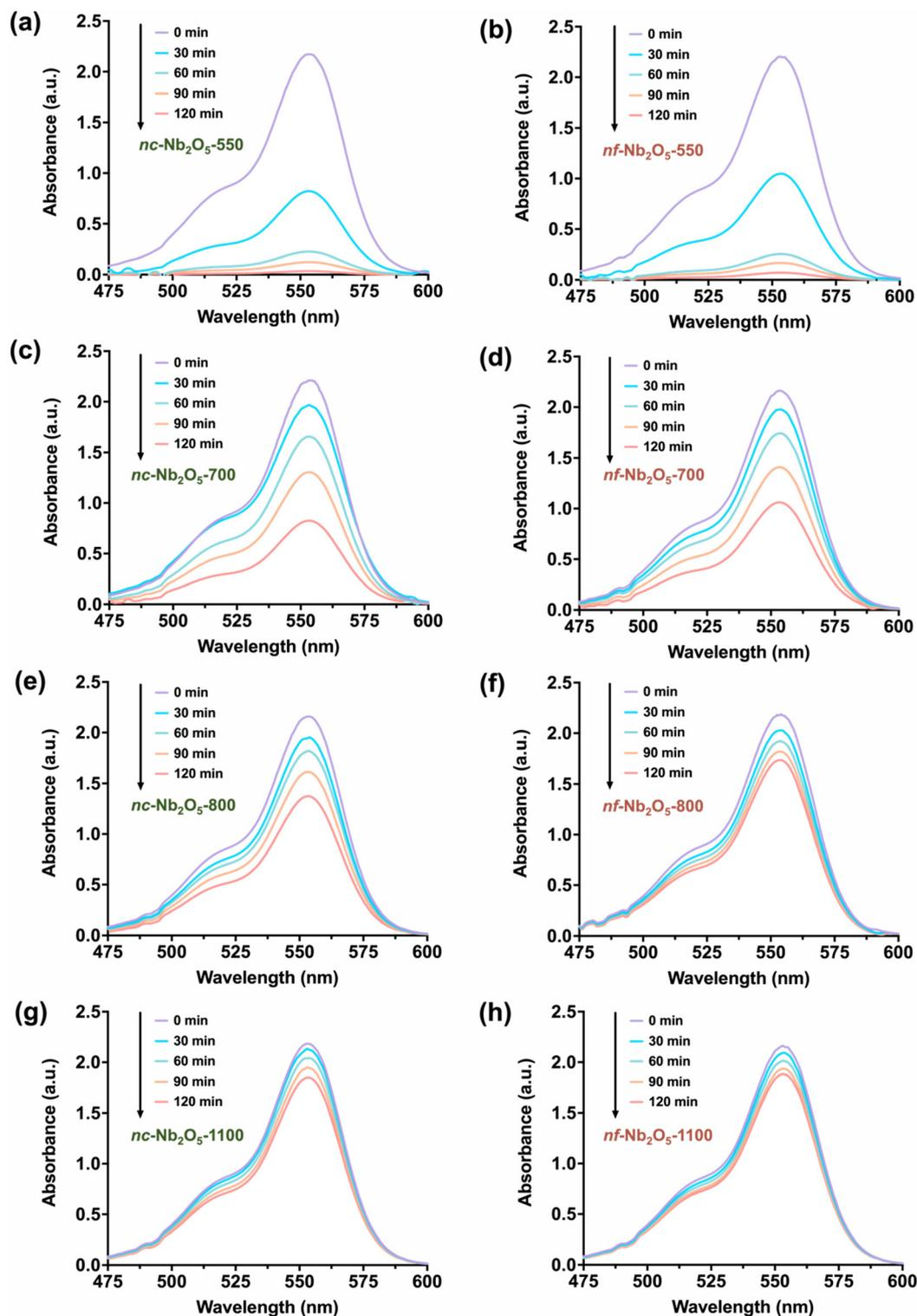
Fig. 4 Absorbance spectral changes of rhodamine B solutions under UV light irradiation in the presence of *nc*-Nb<sub>2</sub>O<sub>5</sub> or *nf*-Nb<sub>2</sub>O<sub>5</sub> prepared at (a and b) 550 °C, (c and d) 700 °C, (e and f) 800 °C and (g and h) 1100 °C.
