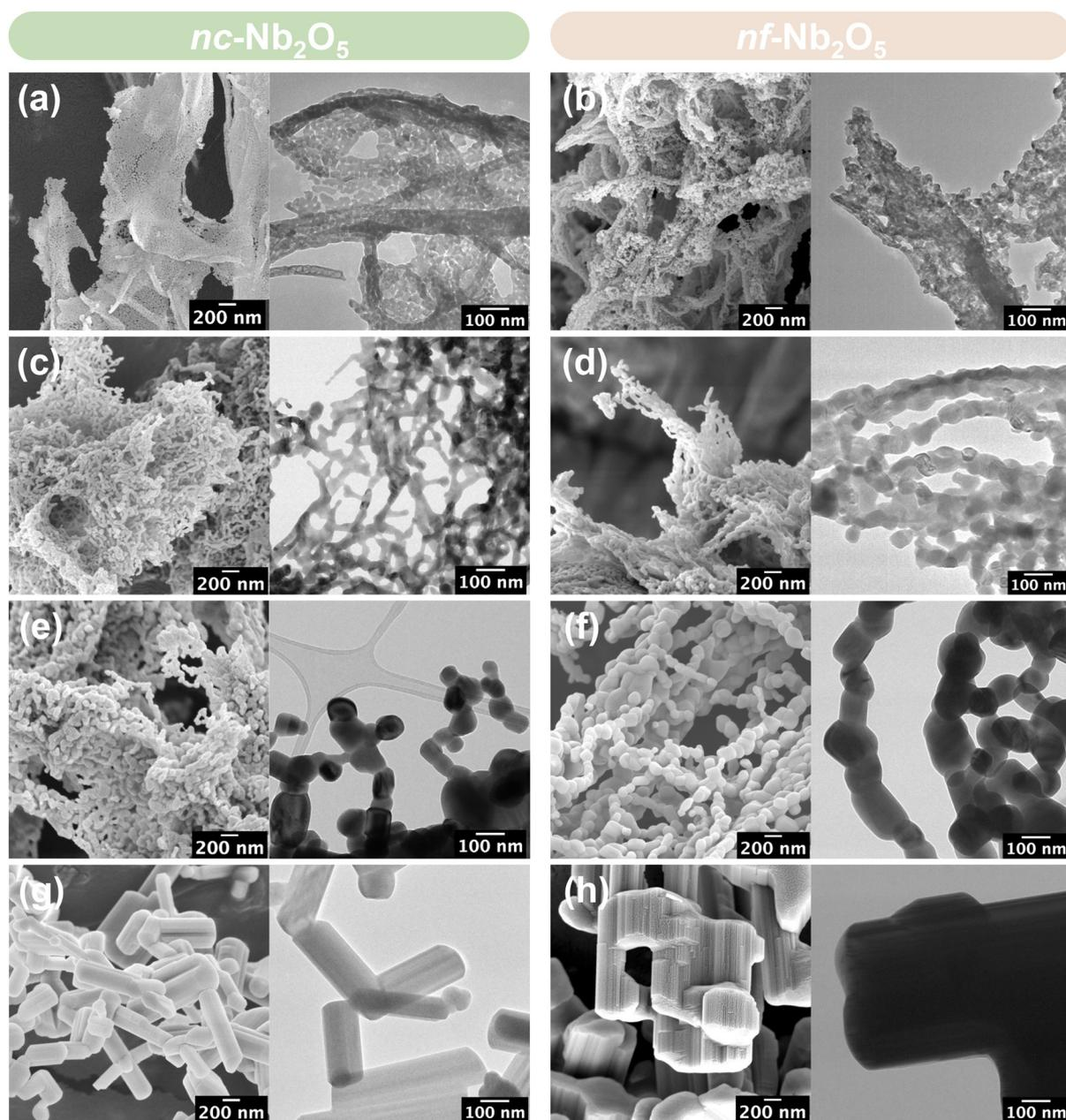
Fig. 2 SEM and TEM micrographs of *nc*-Nb<sub>2</sub>O<sub>5</sub> and *nf*-Nb<sub>2</sub>O<sub>5</sub> synthesised at (a and b) 550 °C, (c and d) 700 °C, (e and f) 800 °C and (g and h) 1100 °C.
