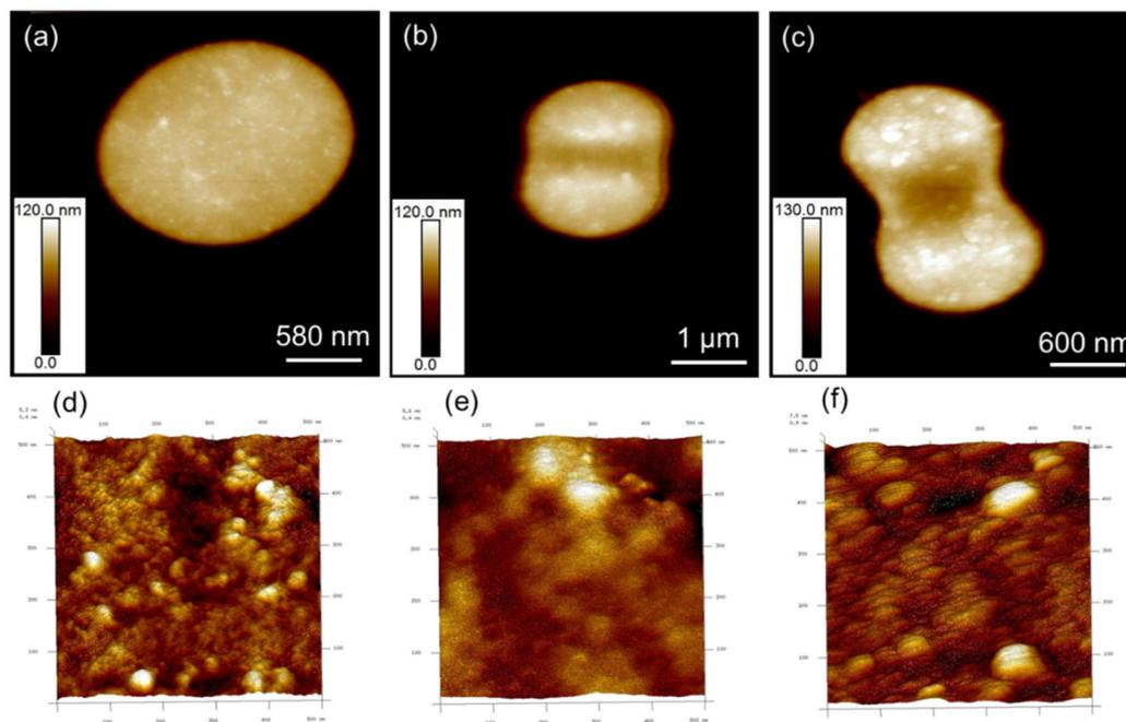
**Fig. 8** AFM height images of dried (PMAA)<sub>15</sub> multilayer hydrogel capsules of (a) ellipsoid, (b) peanut, and (c) hourglass shape. Three-dimensional rendering of the capsule surface morphology from 500 nm<sup>2</sup> areas for (d) ellipsoid-, (e) peanut-, and (f) hourglass-shaped dry (PMAA)<sub>15</sub> hydrogel capsules.
