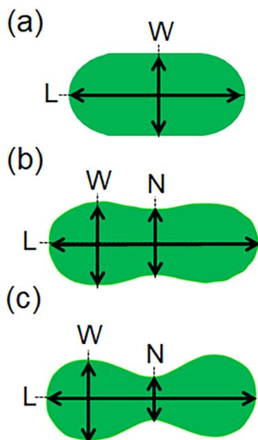
**Fig. 9** The dimensional analysis of the curved rod (PMAA)<sub>15</sub> hydrogel capsules of (a) ellipsoid, (b) peanut, and (c) hourglass shape, including the capsule length,  $L$ , maximum cross-section width,  $W$ , and narrow cross-section width,  $N$ .
