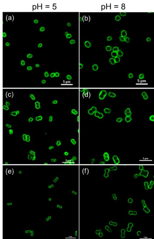
**Fig. 7** CLSM images of (PMAA)<sub>15</sub> multilayer hydrogel capsules of (a and b) ellipsoid, (c and d) peanut, and (e and f) hourglass shape in solution at pH = 5 (left column) and pH = 8 (right column). The scale bar is 5 μm in all images.
