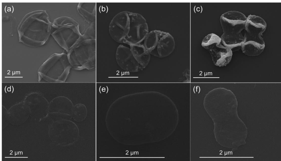
Fig. 4 SEM images of dry (a and b) hydrogen-bonded (PMAA/PVPON)<sub>10</sub> and (d–f) hydrogel (PMAA)<sub>10</sub> capsules of (a and d) ellipsoid, (b and e) peanut, and (c and f) hourglass shapes.
