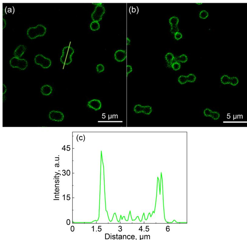
**Fig. 10** High-magnification CLSM images of (PMAA)<sub>15</sub> multilayer hydrogel capsules of (a) peanut and (b) hourglass shapes in solution at pH = 8. (c) A fluorescence profile from the peanut shape capsule in solution at pH = 8 shown in (a).
