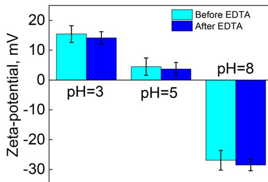
**Fig. 6**  $\zeta$ -potential measurements of (PMAA)<sub>15</sub> hydrogel capsules of hourglass shape at pH = 3, pH = 5, and pH = 8 in 0.01 M phosphate buffer before and after EDTA treatment.
