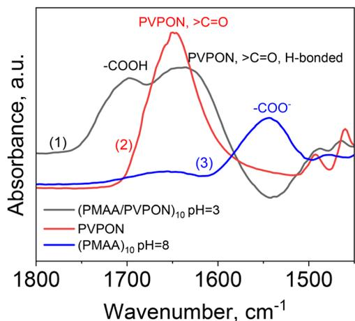
**Fig. 5** ATR-FTIR spectra of freeze-dried hydrogen-bonded (PMAA/PVPON)<sub>10</sub> and hydrogel (PMAA)<sub>10</sub> hydrogel capsules (spectrum 1 and 3, respectively). The hydrogen-bonded capsules were freeze-dried from the capsule solution at pH = 3, while the hydrogel capsules from the capsule solution at pH = 8. PVPON homopolymer was freeze-dried from pH = 3 aqueous solution (spectrum 2).
