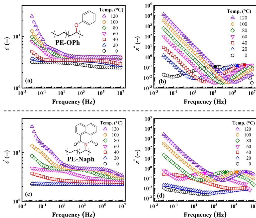
**Fig. 3** Temperature dependence of the measured dielectric properties of the PE derivatives PE-OPh (top) and PE-Naph (bottom), including the log–log plots of  $\epsilon'$  ((a) and (c)) and  $\epsilon''$  ((b) and (d)) versus frequency, respectively. The position of the  $\epsilon''$  peak is indicated by a solid symbol.
