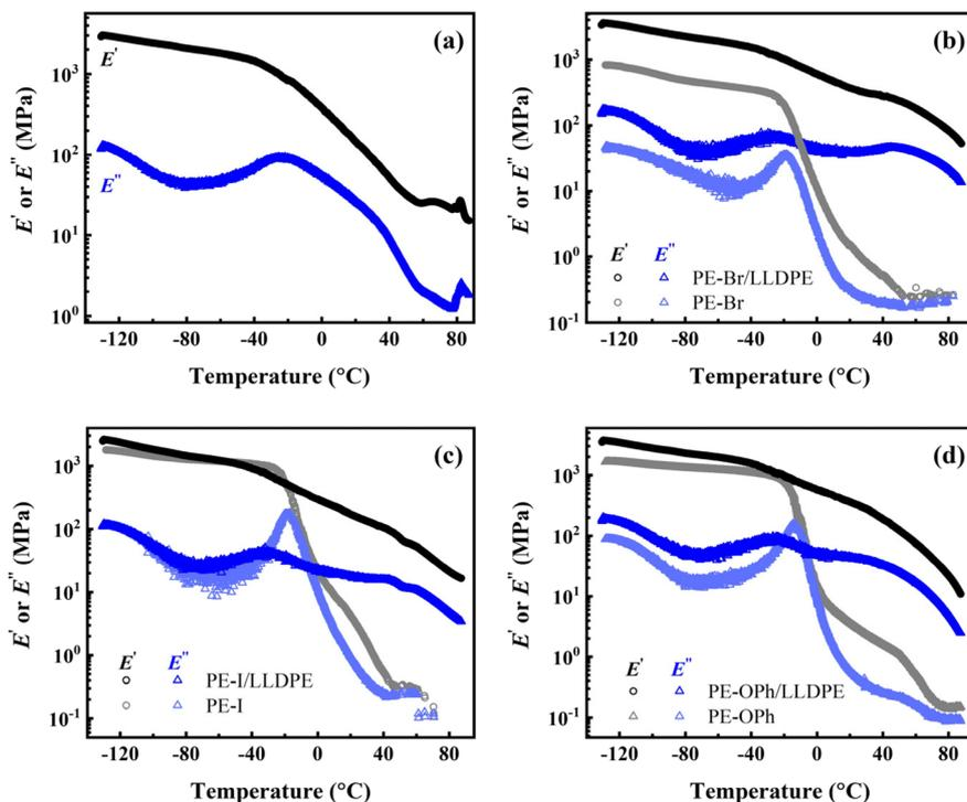
**Fig. 10** DMA curves of the studied PE derivatives and their blends: (a) LLDPE matrix, (b) PE-Br and PE-Br/LLDPE, (c) PE-I and PE-I/LLDPE, and (d) PE-OPh and PE-OPh/LLDPE. The content PE derivatives is 5.9 wt% for the blends.
