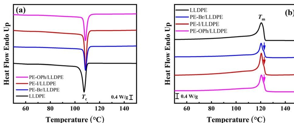
**Fig. 6** (a) Cooling and (b) second heating DSC traces of the PE-Br/LLDPE, PE-I/LLDPE, and PE-Naph/LLDPE blends, with LLDPE employed as the reference. The shoulder peaks in the heating traces are indicated by arrows. The PE derivative content is 5.9 wt% for all the three blends.
