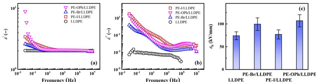
**Fig. 7** Double logarithmic plots of (a)  $\epsilon'$  and (b)  $\epsilon''$  versus frequency obtained from the PE-Br/LLDPE, PE-I/LLDPE, and PE-OPh/LLDPE blends, with a LLDPE matrix used as a reference. (c) Comparison of  $\epsilon_b$  of these blends with the LLDPE matrix. The PE content is 5.9 wt% for all the three blends.
