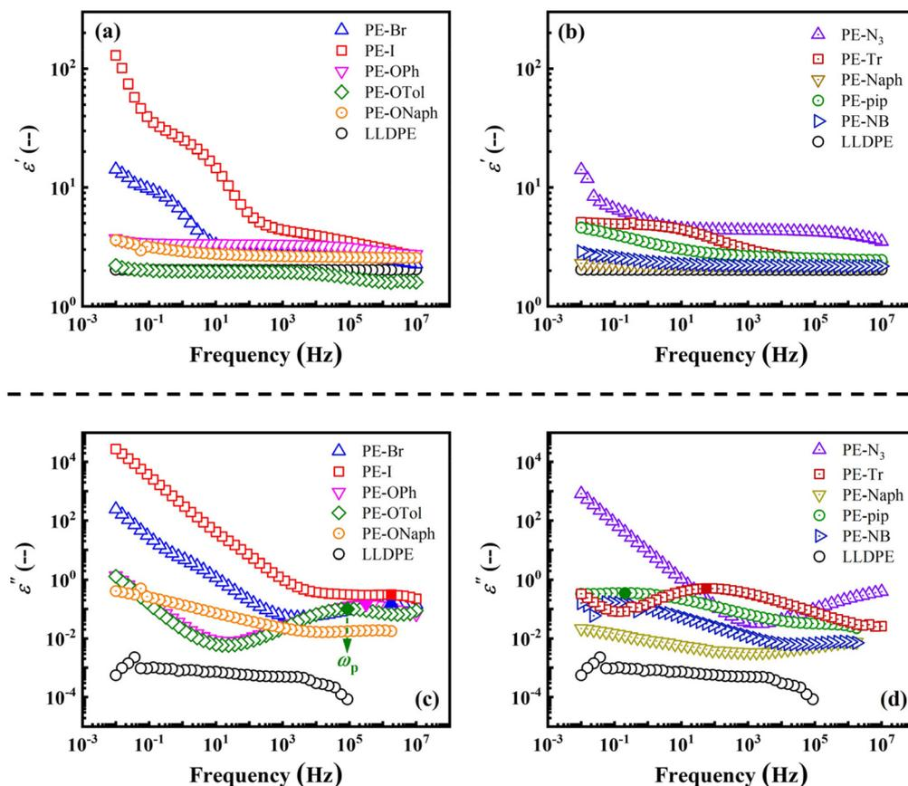
Fig. 2 Double logarithmic plots of (a) and (b)  $\epsilon'$  and (c) and (d)  $\epsilon''$  versus frequency for the synthesized PE derivatives. LLDPE is employed as a basis for comparison. The position of the  $\epsilon''$  peak is indicated by a solid symbol and the frequency at the  $\epsilon''$  peak is denoted as  $\omega_p$ .
