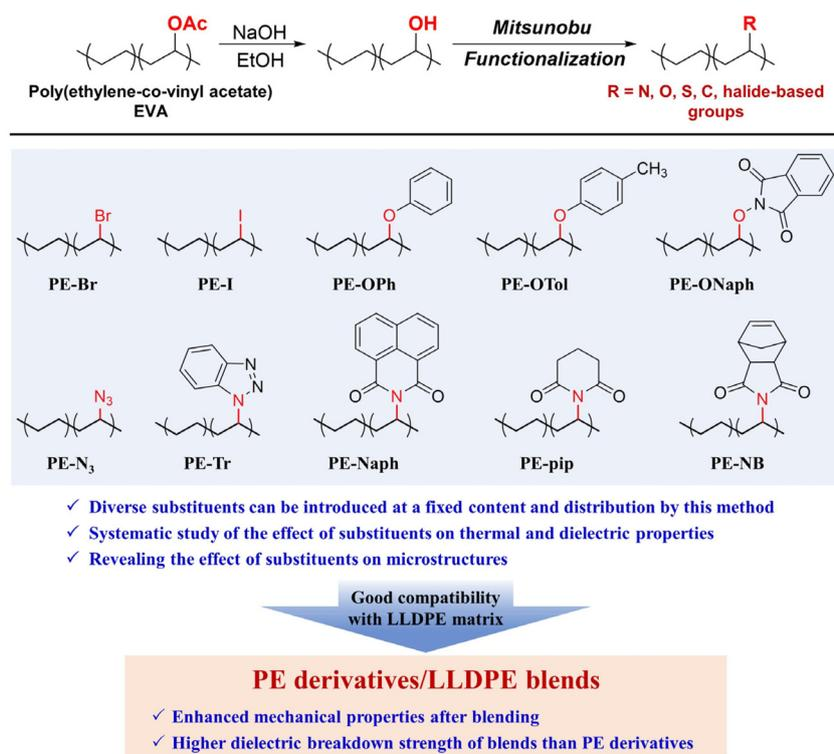
**Scheme 1** General route for preparing PE derivatives from the Mitsunobu reaction (top), and the chemical structures of ten products used in this study. The PE backbone ensures good compatibility between the resulting PE derivatives and LLDPE, facilitating the preparation of their blends.
