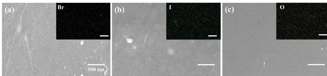
**Fig. 5** SEM images of (a) PE-Br/LLDPE, (b) PE-I/LLDPE, and (c) PE-OPh/LLDPE blends. The EDX mapping results of (a) bromine, (b) iodine, and (c) oxygen are shown in the inset images. The scale bar corresponds to 500 nm. The content of PE derivatives is 5.9 wt% for all the three blends.
