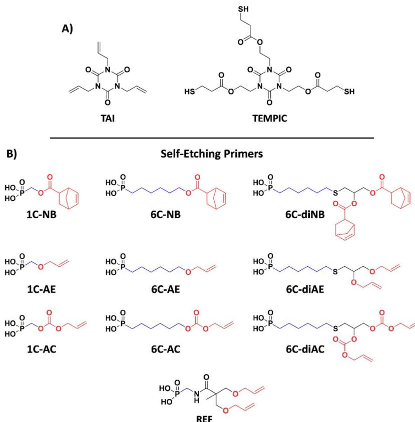
**Fig. 1** Schematic representation of the compounds of the TEC-adhesive formulation: (A) thiol-ene matrix consisting of TAI and TEMPIC and (B) structures of the novel primer molecules containing different spacer lengths (1C or 6C, marked in blue) and type and number of polymerizable groups ((di)NB, (di)AE, (di)AC, marked in red) as well as the difunctional allyl ether reference primer (REF) used by Granskog *et al.*<sup>6</sup>
