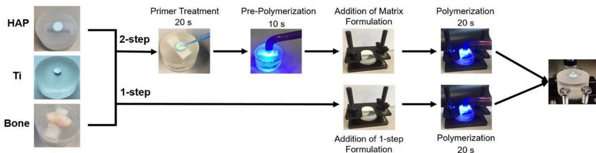
**Fig. 2** Workflows for application of the TEC adhesive for SBS measurements to the different substrates. Two-step procedure with the pre-treatment with the primer formulation, pre-polymerization, the addition of matrix formulation followed by the final polymerization step. One-step procedure with the addition of the primer formulation followed by the final polymerization step.
