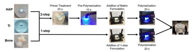
Fig. 2 Workflows for application of the TEC adhesive for SBS measurements to the different substrates. Two-step procedure with the pre-treatment with the primer formulation, pre-polymerization, the addition of matrix formulation followed by the final polymerization step. One-step procedure with the addition of the primer formulation followed by the final polymerization step.
