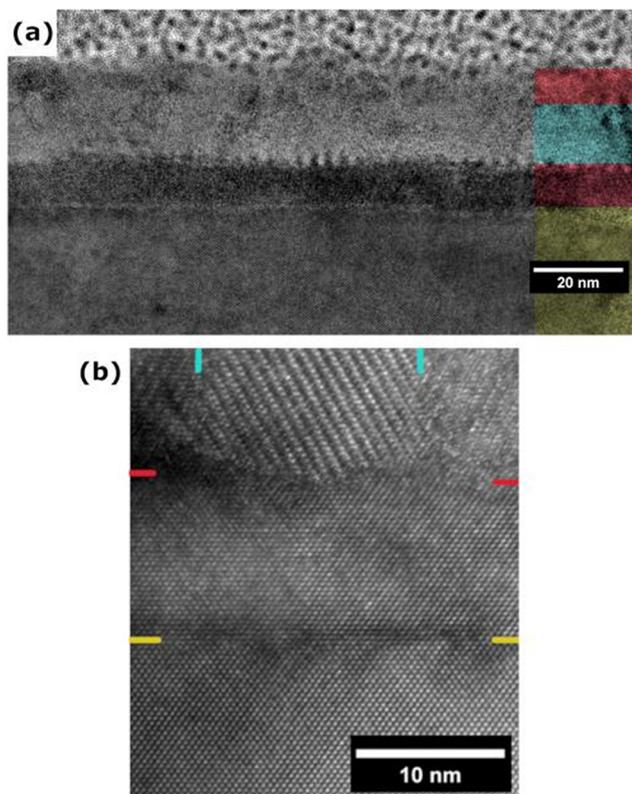
**Fig. 10** TEM images of a SrMnSb<sub>2</sub> sample grown on a GaSb buffer layer on InAs(001). Panel (a) shows an overview with colour blocks on the right highlighting the layer structure (yellow InAs, red GaSb, teal SrMnSb<sub>2</sub>). Panel (b) shows a higher resolution image of the GaSb buffer layer interfaces to the underlying InAs (yellow dashes) and the overgrown SrMnSb<sub>2</sub> (red dashes). Vertical teal dashes show two grain boundaries in the SrMnSb<sub>2</sub> epilayer.
