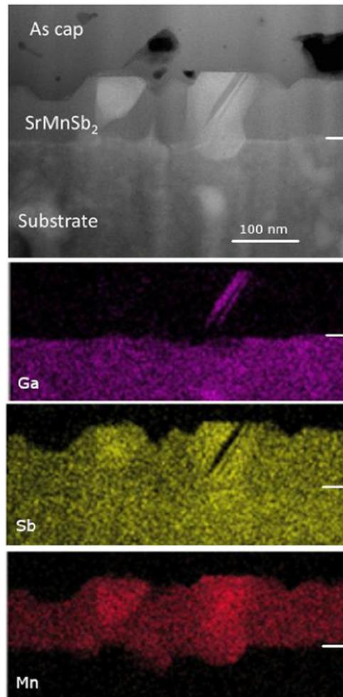
Fig. 9 STEM image and three EDX maps (Ga, Sb, Mn) for SrMnSb<sub>2</sub> grown directly on GaSb(001). The interface is highlighted by white dashes on the right in each panel.
