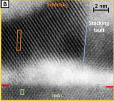
Fig. 8 TEM and STEM images for  $SrMnSb_2$  grown directly on InAs(001), with interface highlighted by red dashes. The large scale image A shows some disruption at and below the interface (red dashes), and grain structure in the film. Image B at high magnification shows the unit cells of film and substrate (orange and green rectangles). A stacking fault is highlighted by a blue line.
