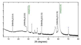
Fig. 3 XRD data for 80 nm SrMnSb<sub>2</sub> grown directly on InAs(001). Substrate and SrMnSb2 peaks are labelled. The asterisks denote secondary phases.
