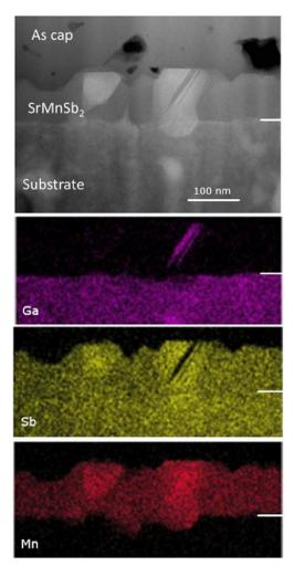
Fig. 9 STEM image and three EDX maps (Ga, Sb, Mn) for SrMnSb<sub>2</sub> grown directly on GaSb(001). The interface is highlighted by white dashes on the right in each panel.
