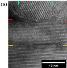
Fig. 10 TEM images of a SrMnSb<sub>2</sub> sample grown on a GaSb buffer layer on InAs(001). Panel (a) shows an overview with colour blocks on the right highlighting the layer structure (yellow InAs, red GaSb, teal SrMnSb<sub>2</sub>). Panel (b) shows a higher resolution image of the GaSb buffer layer interfaces to the underlying InAs (yellow dashes) and the overgrown SrMnSb2 (red dashes). Vertical teal dashes show two grain boundaries in the SrMnSb2 epilayer.
