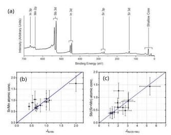
Fig. 5 (a) XPS survey scan for a SrMnSb2 sample grown directly on InAs(001), with all peaks indexed. (b) Sr/Mn composition ratio inferred from XPS as a function of Sr/Mn BEP ratio. (b) Sb/(Sr + Mn) composition ratio inferred from XPS as a function of Sb/(Sr + Mn) BEP ratio. In (b) and (c) the blue straight lines indicate stoichiometric incorporation.
