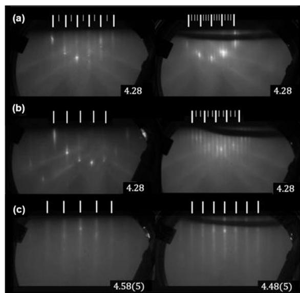
Fig. 2 RHEED patterns for SrMnSb<sub>2</sub> grown on GaSb buffer on InAs(001) in the [110] and [110] azimuths. Long white dashes indicate integer order surface streaks, while short dashes highlight fractional orders. Inset numbers show the lattice parameter in Å. Row (a) shows the as-prepared InAs(001) surface. Row (b) shows the completed GaSb(001) buffer layer. Row (c) shows the completed SrMnSb<sub>2</sub> layer.
