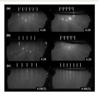
Fig. 2 RHEED patterns for SrMnSb2 grown on GaSb buffer on InAs(001) in the [110] and [110] azimuths. Long white dashes indicate integer order surface streaks, while short dashes highlight fractional orders. Inset numbers show the lattice parameter in Å. Row (a) shows the as-prepared InAs(001) surface. Row (b) shows the completed GaSb(001) buffer layer. Row (c) shows the completed SrMnSb<sub>2</sub> layer.
