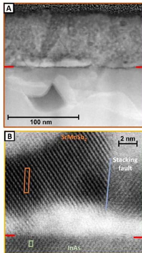
**Fig. 8** TEM and STEM images for SrMnSb<sub>2</sub> grown directly on InAs(001), with interface highlighted by red dashes. The large scale image A shows some disruption at and below the interface (red dashes), and grain structure in the film. Image B at high magnification shows the unit cells of film and substrate (orange and green rectangles). A stacking fault is highlighted by a blue line.
