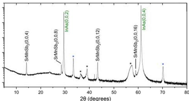
Fig. 3 XRD data for 80 nm SrMnSb<sub>2</sub> grown directly on InAs(001). Substrate and SrMnSb<sub>2</sub> peaks are labelled. The asterisks denote secondary phases.
