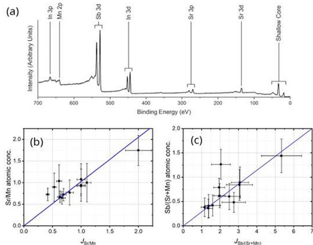
**Fig. 5** (a) XPS survey scan for a SrMnSb<sub>2</sub> sample grown directly on InAs(001), with all peaks indexed. (b) Sr/Mn composition ratio inferred from XPS as a function of Sr/Mn BEP ratio. (c) Sb/(Sr + Mn) composition ratio inferred from XPS as a function of Sb/(Sr + Mn) BEP ratio. In (b) and (c) the blue straight lines indicate stoichiometric incorporation.
