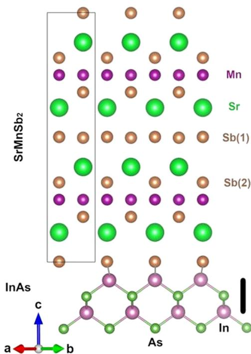
Fig. 1 SrMnSb<sub>2</sub> crystal structure and possible epitaxy on InAs(001). The crystallographic axes refer to the substrate and colour-coded atoms are labelled in the figure. The SrMnSb<sub>2</sub> is shown in the *ac*-plane and the InAs in a [110] plane. The vertical black bar represents the surface atomic step height on InAs(001).
