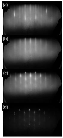
Fig. 6 RHEED patterns in the [110] direction for SrMnSb2 grown directly on InAs(001). (a) As-prepared InAs(001) surface, with 2× periodicity; (b) 1 minute SrMnSb<sub>2</sub> deposited (0.6 nm  $\approx$  0.25 ML); (c) 4 nm deposited; (d) 50 nm desposited.
