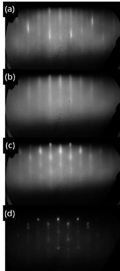
**Fig. 6** RHEED patterns in the [110] direction for SrMnSb<sub>2</sub> grown directly on InAs(001). (a) As-prepared InAs(001) surface, with 2× periodicity; (b) 1 minute SrMnSb<sub>2</sub> deposited (0.6 nm ≈ 0.25 ML); (c) 4 nm deposited; (d) 50 nm deposited.
