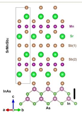
Fig. 1 SrMnSb<sub>2</sub> crystal structure and possible epitaxy on InAs(001). The crystallographic axes refer to the substrate and colour-coded atoms are labelled in the figure. The SrMnSb<sub>2</sub> is shown in the ac-plane and the InAs in a [110] plane. The vertical black bar represents the surface atomic step height on InAs(001).
