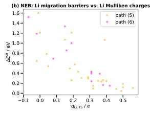
Fig. 6 Li migration barriers  $\Delta E^{\text{M}}$  (in eV), averaged over both C  $\rightarrow$  Si and Si  $\rightarrow$  C directions, plotted in (a) against the minimum Li–Si distances in the transition state  $r_{\text{Li-Si,TS}}^{\text{min}}$  (in Å) for paths (3) to (6), and in (b) against the Li Mulliken charges in the transition state  $q_{\text{Li,TS}}$  (in units of e) for paths (5) and (6).
