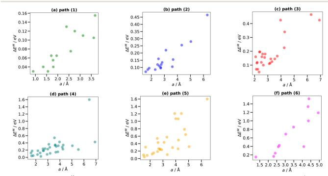
Fig. 5 Li migration barriers  $\Delta E^{M}$  (in eV), averaged over both C  $\rightarrow$  Si and Si  $\rightarrow$  C directions, plotted against Li hopping distances a (in Å) for (a) path (1), (b) path (2), (c) path (3), (d) path (4), (e) path (5), and (f) path (6).
