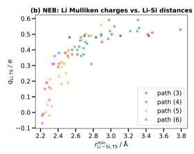
Fig. 7 (a) Median Li Mulliken charges  $\tilde{q}_{\text{Li}}$  (in units of e) for Li atoms moving freely in bulk Si at 400 K, plotted against the position of the first peaks of the Li–Si RDFs  $r_{\text{Li-Si}}^{(1)}$  (in Å). (b) Li Mulliken charges in the transition state  $q_{\text{Li,TS}}$  (in units of e), plotted against the minimum Li–Si distances in the transition state  $r_{\text{Li-Si,TS}}^{\text{min}}$  (in Å) for paths (3) to (6).
