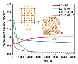
Fig. 8 Long-term PEC water splitting stability of indium sulfide thin films under continuous 1 sun illumination using a mixture of 0.025 M Na<sub>2</sub>S<sub>2</sub>9H<sub>2</sub>O and 0.025 M Na<sub>2</sub>SO<sub>3</sub> electrolyte solution (pH = 12.32). The inset highlights the strucutre of the crystallographic facets (311) and (440).
