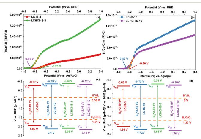
Fig. 7 Mott-Schottky plots of the prepared indium thin films were generated in 0.5 M  $Na_2SO_4$  (pH = 6.5) (a) and (b); band edge potentials vs. RHE at pH 6.5 (c); band edge potentials vs. RHE or NHE at pH 0 (d).
