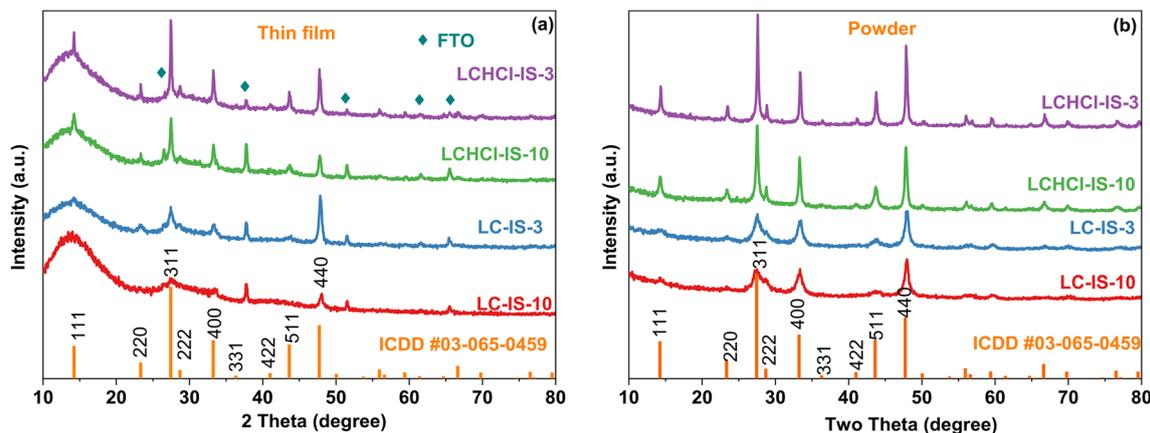
Fig. 2 XRD patterns: (a) the as-produced indium sulfide thin films, and (b) collected corresponding powders.
