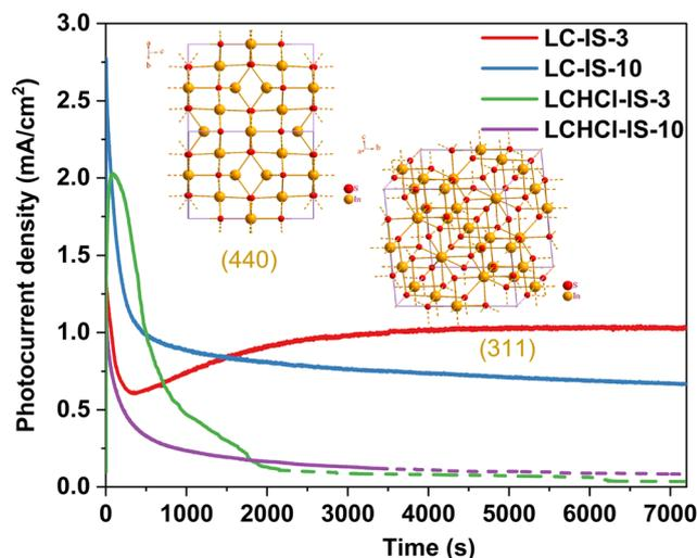
**Fig. 8** Long-term PEC water splitting stability of indium sulfide thin films under continuous 1 sun illumination using a mixture of 0.025 M  $\text{Na}_2\text{S}\cdot 9\text{H}_2\text{O}$  and 0.025 M  $\text{Na}_2\text{SO}_3$  electrolyte solution (pH = 12.32). The inset highlights the structure of the crystallographic facets (311) and (440).
