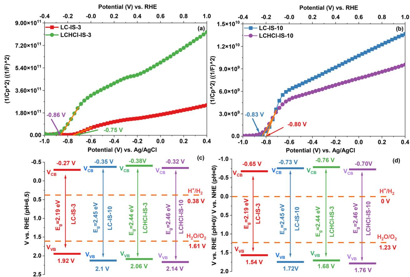
Fig. 7 Mott-Schottky plots of the prepared indium thin films were generated in 0.5 M  $\text{Na}_2\text{SO}_4$  (pH = 6.5) (a) and (b); band edge potentials vs. RHE at pH 6.5 (c); band edge potentials vs. RHE or NHE at pH 0 (d).
