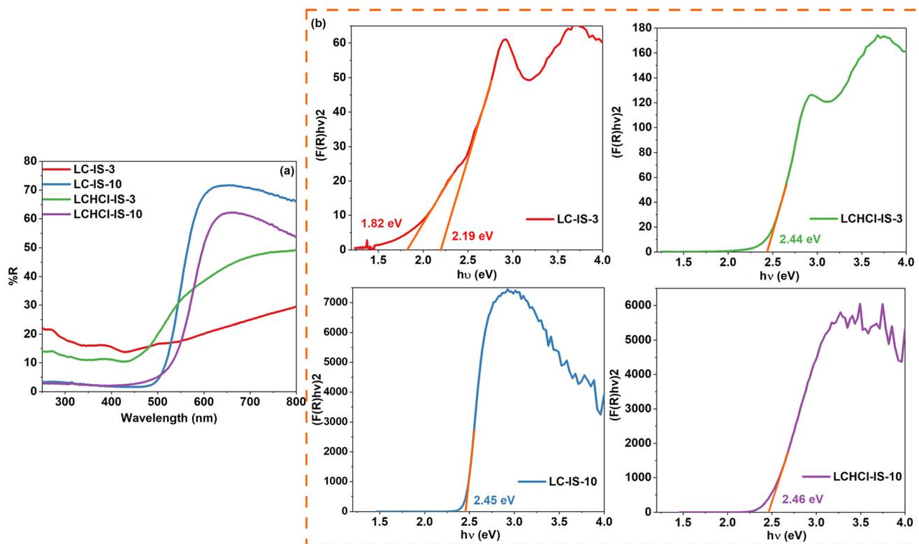
Fig. 5 UV-vis DRS of the thin films (a) and (b) corresponding  $(F(R)/hv)^2$  vs.  $h\nu$  plots derived from the Kubelka–Munk function.<sup>48</sup>
