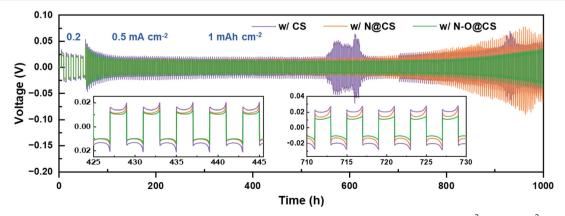
Fig. 6 Voltage profiles of symmetric Li|Li cells with the CS, N@CS, and N-O@CS separators at 0.2 and 0.5 mA cm<sup>-2</sup>, 1 mAh cm<sup>-2</sup>.
