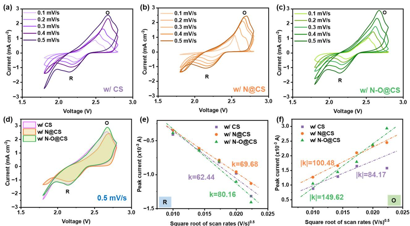
Fig. 4 Electrochemical characterization of Li-S cells using CS, N@CS, and N-O@CS separators. (a–c) Cyclic voltammetry (CV) curves of the three cells at various scan rates ranging from 0.1 to 0.5  $\text{mV s}^{-1}$ . (d) CV curves of all three separators at a fixed scan rate of 0.5  $\text{mV s}^{-1}$ . (e) Reductive peak current vs. square root of scan rates. (f) Oxidative peak current vs. square root of scan rates.
