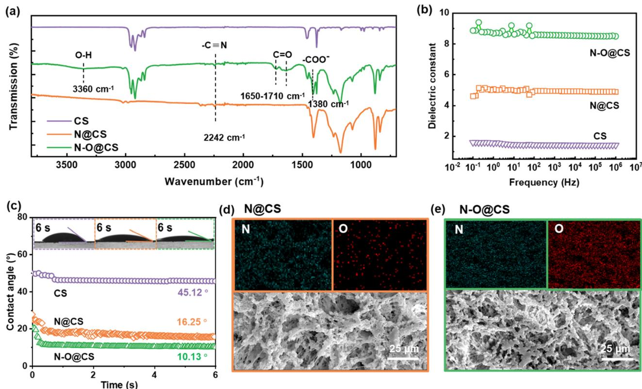
Fig. 2 (a) FTIR spectra of CS, N@CS and N-O@CS separators recorded in the range of 3750–1100 cm<sup>-1</sup>. (b) Dielectric constant of CS, N@CS, and N-O@CS separators measured from 10<sup>-1</sup> to 10<sup>6</sup> Hz. (c) Electrolyte contact angle images of CS, N@CS, and N-O@CS separators. SEM images and corresponding elemental mapping of N and O for the (d) N@CS separator and (e) N-O@CS separator.
