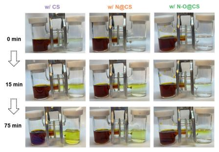
Fig. 3 Polysulfide diffusion test for the CS separator, N@CS separator, and N-O@CS separator with 0.5 M  $\text{Li}_2\text{Sg}$ , after diffusion for 15 and 75 minutes.
