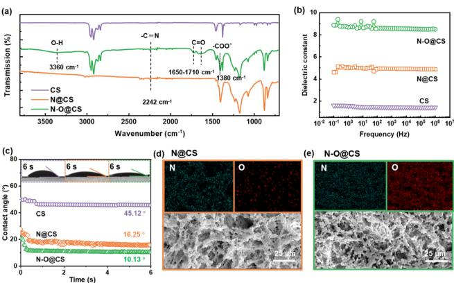
Fig. 2 (a) FTIR spectra of CS, N@CS and N-O@CS separators recorded in the range of 3750-1100 cm<sup>-1</sup>. (b) Dielectric constant of CS, N@CS, and N-O@CS separators measured from  $10^{-1}$  to  $10^{6}$  Hz. (c) Electrolyte contact angle images of CS, N@CS, and N-O@CS separators. SEM images and corresponding elemental mapping of N and O for the (d) N@CS separator and (e) N-O@CS separator.
