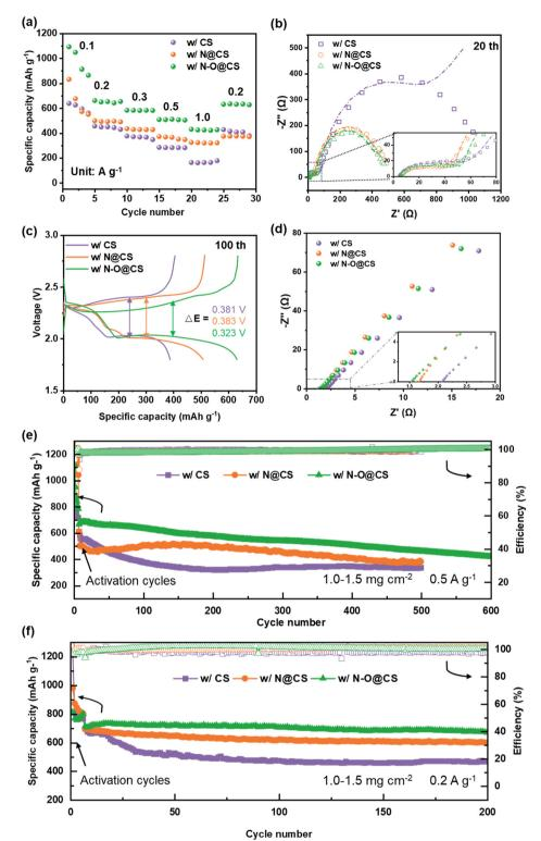
Fig. 7 Electrochemical performance of the Li-S batteries with different separators: CS, N@CS and N-O@CS separators. (a) Rate cycling performance, (b) EIS spectra along with fitted curves (inset shows the enlarged region from 0-80  $\Omega$ ), (c) voltage profiles, (d) EIS plots of SS||SS symmetric cells (inset shows the magnified region from 1.25–3  $\Omega$ ) and long cycling performance at the current density of (e) 0.5 A g<sup>-1</sup> and (f) 0.2 A g<sup>-1</sup>.
