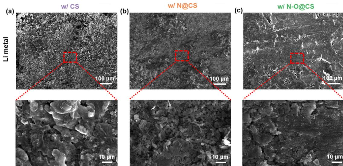
Fig. 5 SEM images of Li metal anodes after CV tests at a scan rate of  $0.1\text{--}0.5\text{ mV s}^{-1}$ . Surface morphologies of Li metal anodes cycled with (a) CS, (b) N@CS, and (c) N-O@CS separators.
