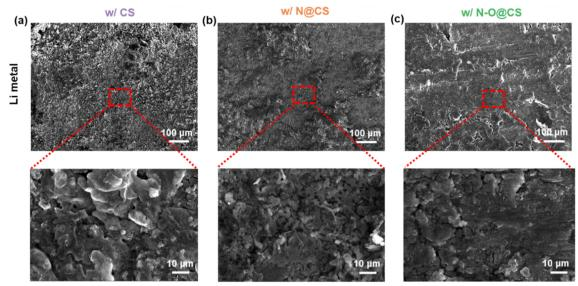
Fig. 5 SEM images of Li metal anodes after CV tests at a scan rate of 0.1-0.5 mV s<sup>-1</sup>. Surface morphologies of Li metal anodes cycled with (a) CS, (b) N@CS, and (c) N-O@CS separators.
