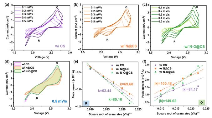
Fig. 4 Electrochemical characterization of Li-S cells using CS, N@CS, and N-O@CS separators. (a-c) Cyclic voltammetry (CV) curves of the three cells at various scan rates ranging from 0.1 to 0.5 mV s<sup>-1</sup>. (d) CV curves of all three separators at a fixed scan rate of 0.5 mV s<sup>-1</sup>. (e) Reductive peak current vs. square root of scan rates. (f) Oxidative peak current vs. square root of scan rates.
