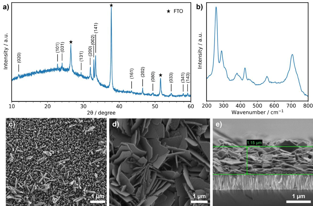
**Fig. 1** a) XRD pattern of  $\text{Ca}_2\text{Fe}_2\text{O}_5$ . The  $(hkl)$  indices are based on JCPDS No. 47-1744. b) Raman spectrum of  $\text{Ca}_2\text{Fe}_2\text{O}_5$ . SEM images of c)  $\text{FeOOH}$  nanorods, d)  $\text{Ca}_2\text{Fe}_2\text{O}_5$  nanoflakes, e) cross-section of  $\text{Ca}_2\text{Fe}_2\text{O}_5$  deposited on FTO glass.
