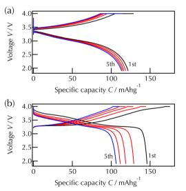
Fig. 6 Charge-discharge curves of (a) 50% Li-polymer/LiNbO<sub>3</sub>/ LiCoO2-LGPS and (b) LiNbO3/LiCoO2-LGPS composite cathodes in the voltage region of 4.0-1.9 V. The charge-discharge tests are conducted at 298 K and 0.05C.
