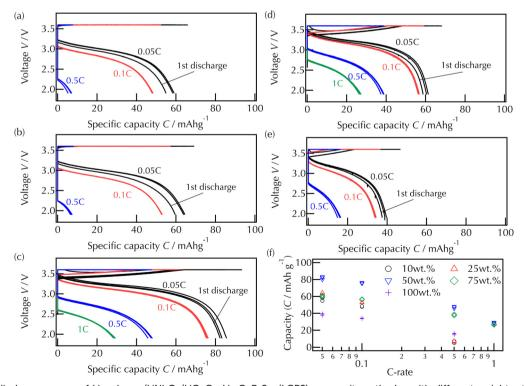
Fig. 2 Charge-discharge curves of Li-polymer/LiNbO<sub>3</sub>/LiCoO<sub>2</sub>-Li<sub>10</sub>GeP<sub>2</sub>S<sub>12</sub> (LGPS) composite cathodes with different weight ratios of LiMTFSI to PEGMA: (a) 10, (b) 25, (c) 50, (d) 75, and (e) 100 wt%. (f) Variations in the discharge capacity retention with different C rates. All tests were conducted at 298 K (25 °C). The discharge current density increased from 0.05 and 1C every three cycles.
