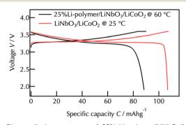
Fig. 4 Charge-discharge curves of 25% Li-polymer/LiNbO<sub>3</sub>/LiCoO<sub>2</sub>-LGPS at 333 K (60  $^{\circ}$ C) and LiNbO<sub>3</sub>/LiCoO<sub>2</sub>-LGPS at 298 K (25  $^{\circ}$ C). The charge-discharge current density is 0.05C. Charge-discharge curves of 25% Li-polymer/LiNbO3/LiCoO2-LGPS at 298 K is shown in Fig. 2b.
