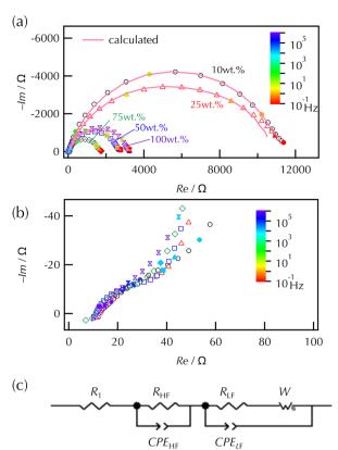
Fig. 3 (a) Nyquist plots and fitting curves of all-solid-state batteries using Li-polymer/LiNbO<sub>3</sub>/LiCoO<sub>2</sub>-LGPS composite cathodes at varying weight ratios of LiMTFSI to PEGMA of 10, 25, 50, 75, and 100 wt%. EIS data were collected after the cycle tests. (b) Enlarged spectra of (a) high-frequency region. (c) Equivalent circuit model used for curvefittina.
