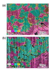
Fig. 5 SEM-EDX images of (a) 25% Li-polymer/LiNbO<sub>3</sub>/LiCoO<sub>2</sub>-LGPS and (b) LiNbO<sub>3</sub>/LiCoO<sub>2</sub>-LGPS cathode composites.
