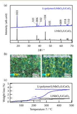
Fig. 1 (a) XRD patterns, (b) SEM-EDX images, and (c) TG curves of  $\label{eq:linbo3} LiNbO_3/LiCoO_2 \ and \ Li-polymer/LiNbO_3/LiCoO_2. \ The \ Li-polymer/LiNbO_3/LiCoO_3.$ LiCoO<sub>2</sub> was dried in vacuum at 213 and 323 K. The weight ratio of lithium 3-[(trifluoromethane)sulfonamidosulfonyl]propyl methacrylate (LiMTFSI) to PEGMA was 50%.
