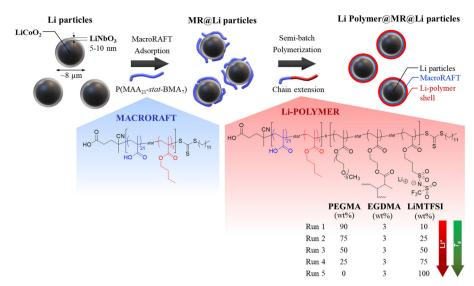
Scheme 1 RAFT assisted encapsulating polymerisation of LiNbO<sub>3</sub>/LiCoO<sub>2</sub> with different LiMTFSI/PEGMA content.
