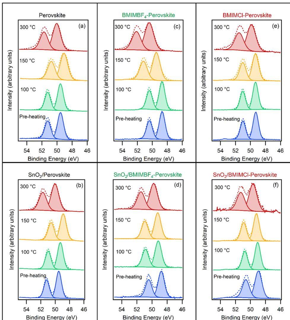
**Fig. 3** High-resolution I 4d core level XPS spectra of pure (a) and (b) and IL-modified ((c)–(f)) perovskite films deposited on Ti foil ((a), (c) and (e)) and SnO<sub>2</sub> coated Ti foil ((b), (d) and (f)). The dotted lines represent the raw data and the coloured areas represent the fitted components. Spectra have been normalised to the intensity of the I 4d<sub>5/2</sub> peak.
