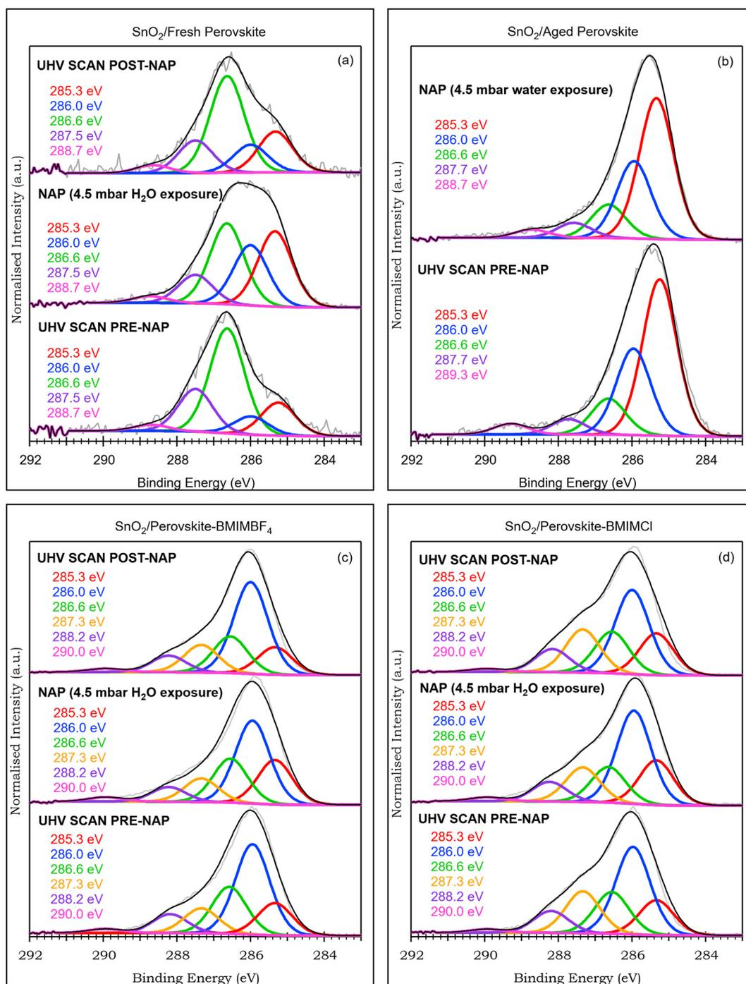
**Fig. 8** High-resolution core level C 1s spectra of pure (a) and (b) and IL-modified ((c) and (d)) perovskite films on SnO<sub>2</sub> coated Ti foil measured before exposure, during exposure and after exposure to 4.5 mbar water vapour at room temperature. Spectral intensities are normalised to the intensity of the highest peak. BEs of fitted peaks are shown next to each spectrum and are assigned to the same chemical environments as described in Fig. 1.
