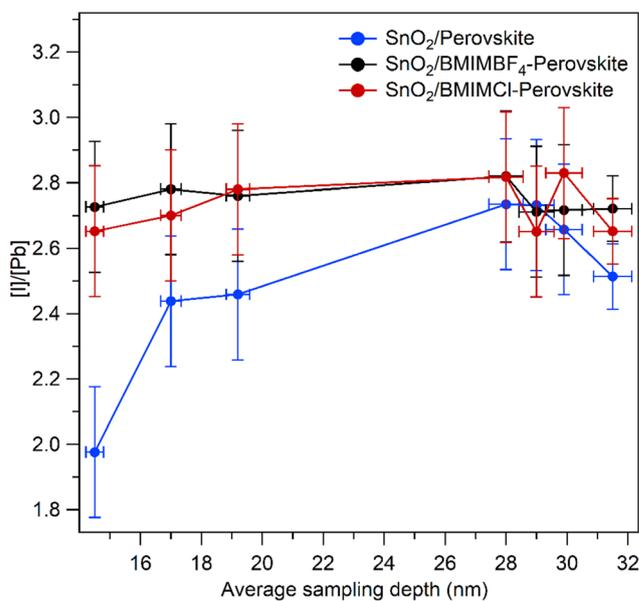
Fig. 7 I/Pb ratios from HAXPES as a function of averaging sampling depth for pure and IL-modified perovskite films on SnO<sub>2</sub>.
