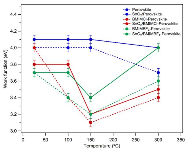
Fig. 5 Work function values of pure and IL-modified perovskite films as a function of temperature. Solid lines represent the films with a SnO<sub>2</sub> layer while the dashed lines represent films without the SnO<sub>2</sub> layer.
