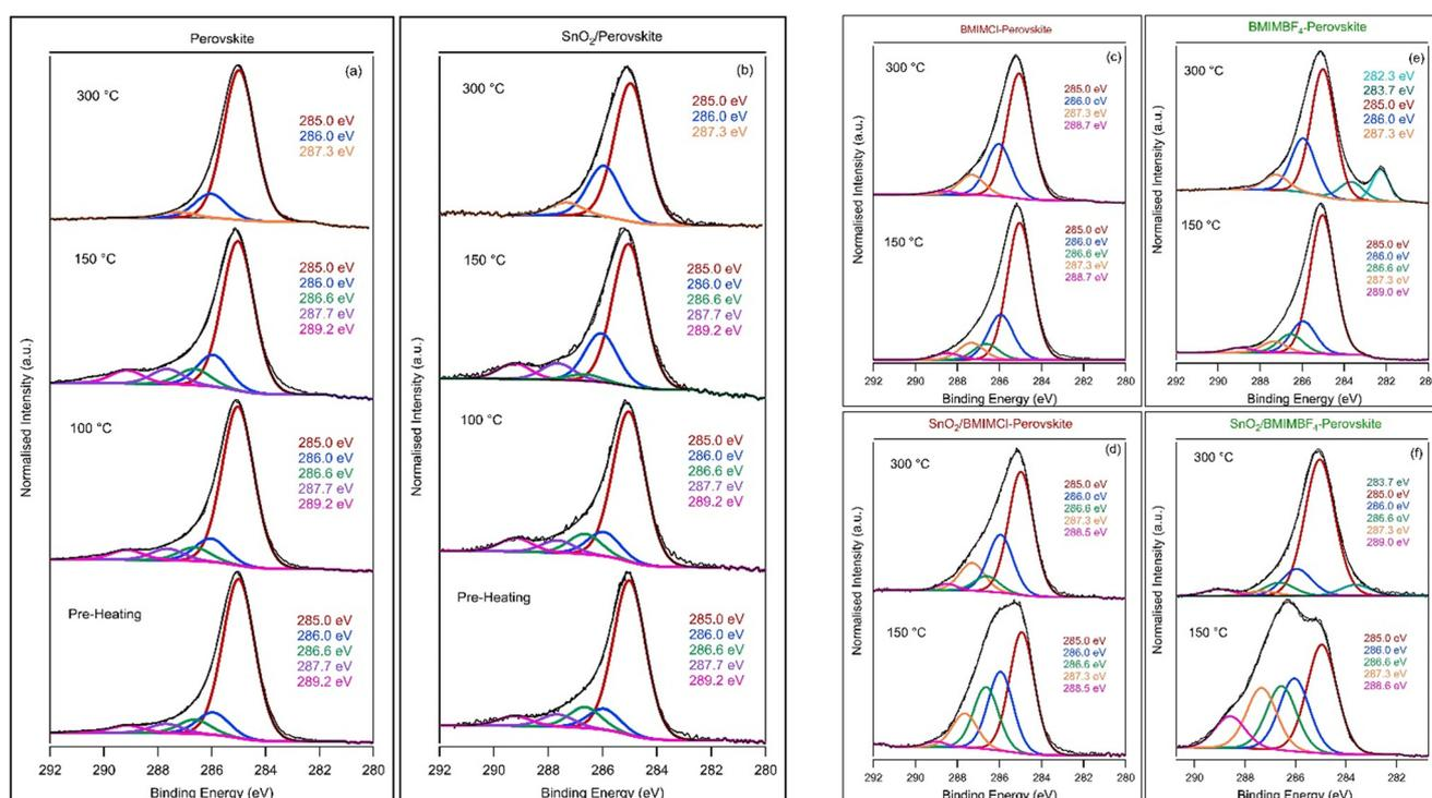
Fig. 2 High-resolution C 1s core level XPS spectra of the pure ((a) and (b)) and IL-modified ((c)–(f)) perovskite films deposited on Ti foil ((a), (c) and (e)) and SnO<sub>2</sub> coated Ti foil ((b), (d) and (f)). Peak intensities are normalised to the intensity of the adventitious carbon peak. BEs of fitted peaks are shown next to each spectrum and a summary of C 1s peak assignments is shown in Fig. 1.
