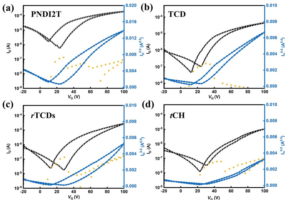
Fig. 3 Transfer characteristics of the pristine FET devices: (a) *PNDI2T*, (b) *TCD*, (c) *rTCDs*, and (d) *tCH* films. The yellow scatter points following the left y-axis represent the gate current measured during  $V_G$  sweeps from -20 to 100 V under a fixed  $V_{DS}$  of 100 V.
