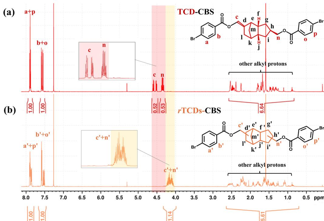
**Fig. 1**  $^1\text{H}$  NMR spectral differences highlighting the structural distinction between (a) the structurally and regio-selective TCD-CBS and (b) the structurally and regio-random  $r\text{TCDs}$ -CBS.
