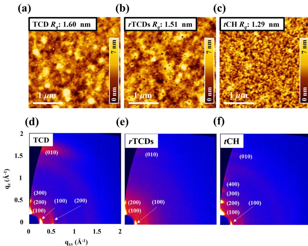
Fig. 4 AFM topographies of the (a) TCD, (b) *r*TCDs, and (c) *t*CH films. (b) 2D diffraction patterns from GIWAXS of the (d) TCD, (e) *r*TCDs, and (f) *t*CH films. These pristine films were characterized without film transfer and stretching.
