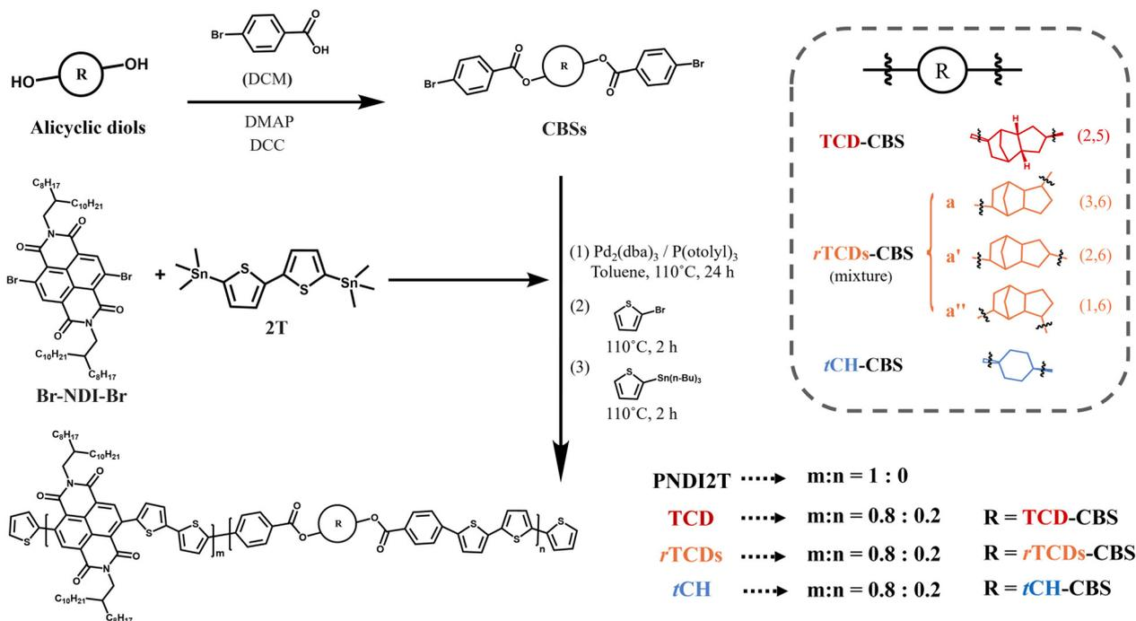
**Scheme 1** Chemical structures and synthetic route of the N-type conjugated polymers incorporating alicyclic units as conjugation break spacers (CBSs) and their copolymerization compositions. Note that the TCD-CBS is in an *endo* configuration with pure 2,5 structure selectivity, and the rTCDs-CBS are in mixed *endo/exo* configurations with the 3,6-, 2,6-, and 1,6-isomers accounting for 90 wt% of the mixture from the commercial source.
