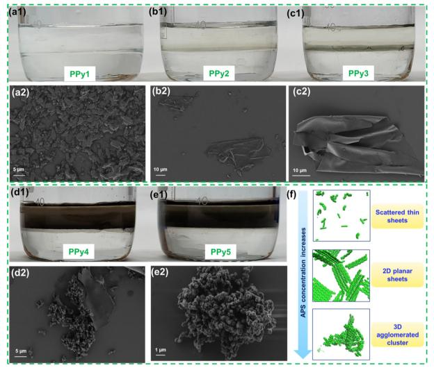
Fig. 8 (a1-e1) Optical images of the formation of PPy at the water-chloroform interface after the polymerization completion PPy1-PPy5, and (a2e2) the corresponding FE-SEM images. (f) Illustration of the transition of product morphology from scattered thin sheets to agglomerated clusters with increasing APS concentrations.
