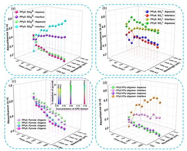
Fig. 7 Absorption peaks for  $SO_4^{2-}$  ions (a) at lower concentrations of APS (PPy2 and PPy3) in the aqueous phase, (b) in higher concentrations of APS (PPy4 and PPy5) in the aqueous phase and (c) absorption peaks of pyrrole in the organic phase for PPy2, PPy3, PPy4, and PPy5. The inset shows the depletion percentage of pyrrole monomers during the reaction. (d) The oligomeric absorbance observed in PPy2 and PPy3 was sample collected from the aqueous and interface.
