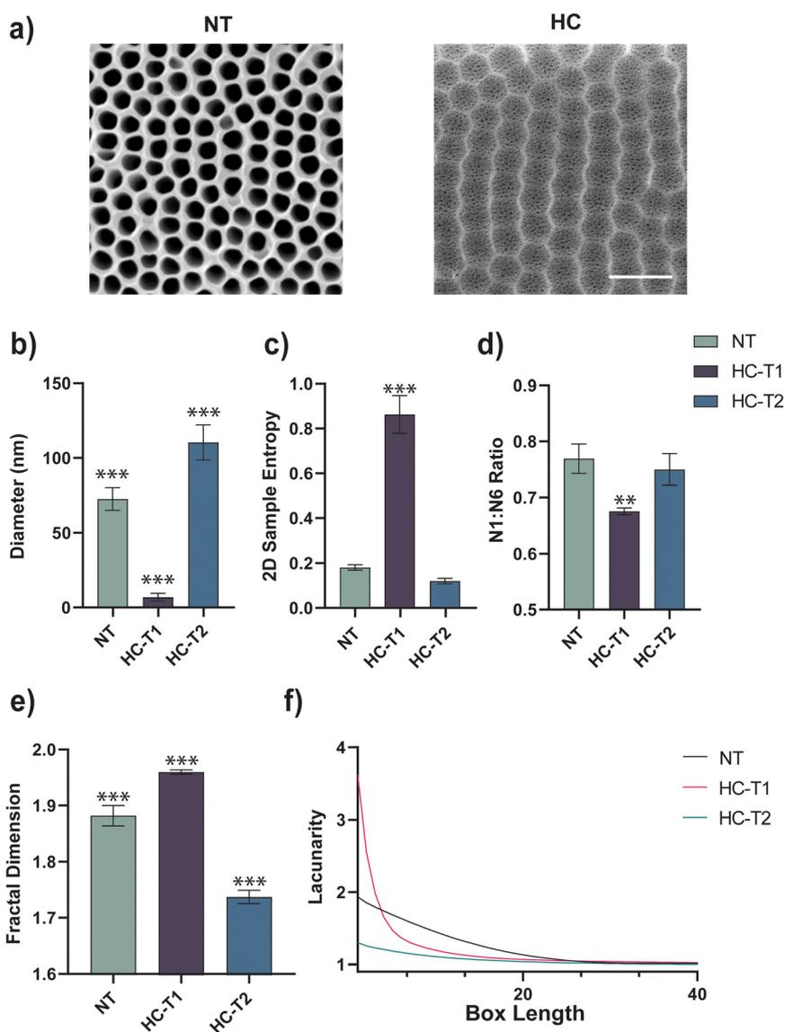
**Fig. 1** SEM images and spatial metrics of the NT and HC surfaces. a) SEM micrographs of the NT surface (left) and the HC architecture (right). Scale bar: 200 nm. b) Nanotube diameter for the NT and the HC surfaces. Spatial statistics: c) surface entropy, d) N1:N6 ratio, e) fractal dimension and f) lacunarity.
