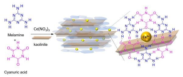
Fig. 5 Proposed schematic representation of the formation mechanism of KCeMC.
