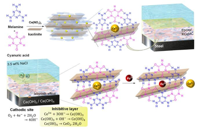
Fig. 8 Illustration outlining the mechanism of protection.
