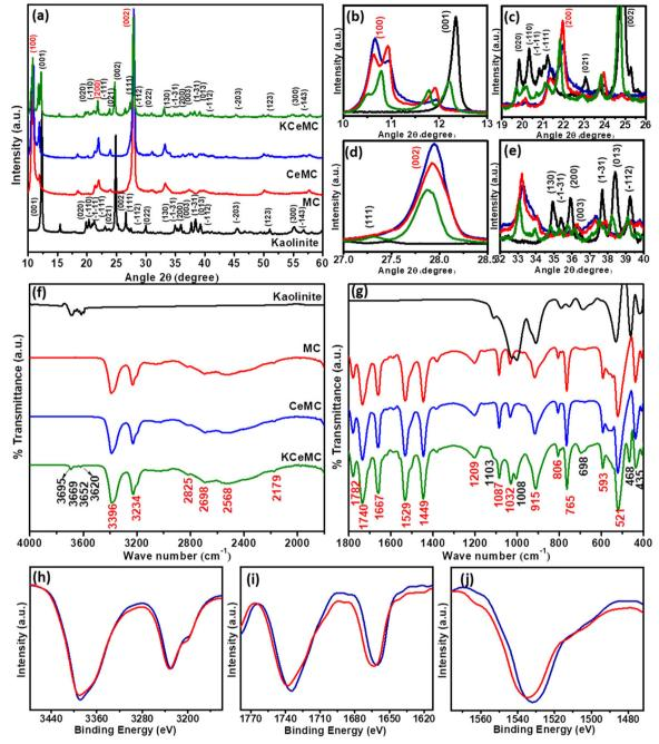
Fig. 2 (a-e) XRD patterns and (f-j) IR bands of kaolinite, MC, CeMC and KCeMC.
