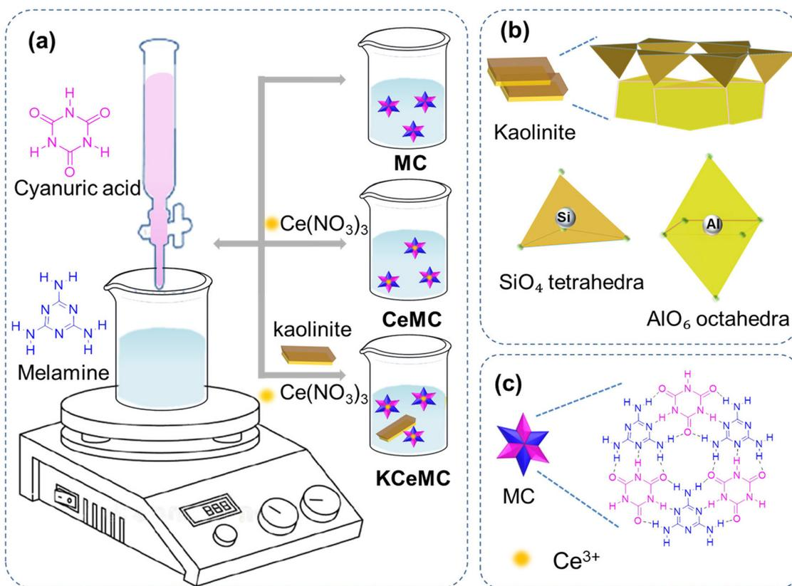
**Fig. 1** (a) Schematic representation of the synthesis process of MC, CeMC and KCeMC, (b) 1:1 layered kaolinite structure formed by silica tetrahedral and alumina octahedral sheets and (c) schematic illustrating MC with alternating complementary H-bonds between melamine and cyanuric acid.
