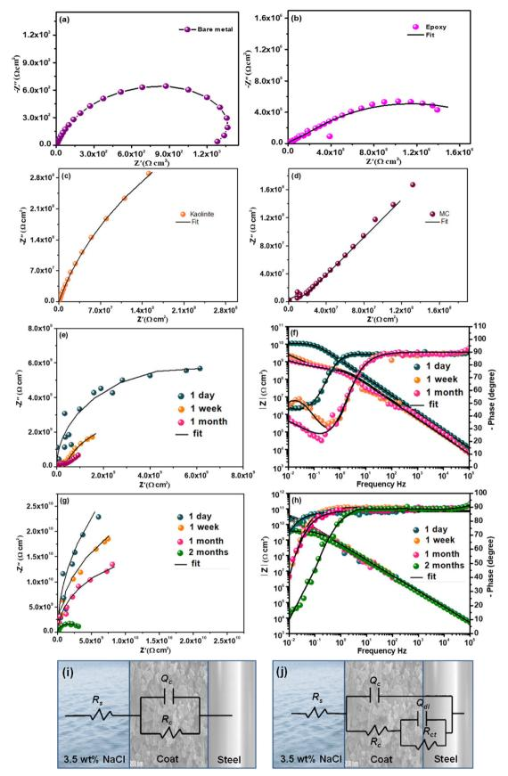
Fig. 6 Nyquist plots of (a) bare steel, (b) pristine epoxy, (c) kaolinite/epoxy, and (d) MC/epoxy and Nyquist and corresponding Bode plots of 1 wt% synthesised anticorrosive pigments with different immersion times in 3.5 wt% NaCl solution: (e and f) CeMC and (g and h) KCeMC. (i) and (j) Schematic images of the equivalent electrochemical circuit model applied to fit the experimental impedance data.
