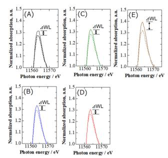
Fig. 10 XANES spectra of  $(PtCl_n)_{0.9nm}/Fe-N-C$  electrode with (A) N=0, (B) N=5, (C) N=25, and (D) N=75 and (E) commercial Pt/C (N=0) at (----) 0.4 V and (—) 1.0 V in N2-purged 0.1 M HClO4.
