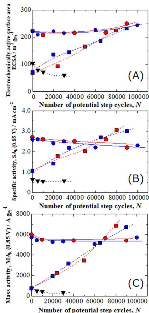
**Fig. 6** (A) ECSA, (B) SA<sub>k</sub>, and (C) MA<sub>k</sub> for the ORR for Nafion-coated (●) (PtCl<sub>n</sub>)<sub>1.3nm</sub>/Fe-N-C, (●) \*[(PtCl<sub>n</sub>)<sub>1.3nm</sub>/Fe-N-C], (■) (PtCl<sub>n</sub>)<sub>0.9nm</sub>/Fe-N-C, (■) \*[(PtCl<sub>n</sub>)<sub>0.9nm</sub>/Fe-N-C], and (▼) commercial Pt/C electrodes as a function of *N*.
