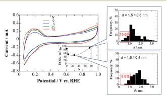
Fig. 9 Cyclic voltammograms employed to determine the ECSA values and particle size distribution histograms for Nafion-coated (PtCl<sub>n</sub>)<sub>0.9nm</sub>/Fe-N-C electrode in 0.1 M HClO<sub>4</sub> solution deaerated with  $N_2$  at room temperature at a scan rate of 50 mV s<sup>-1</sup>.
