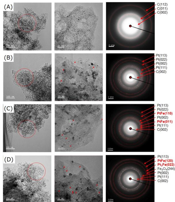
Fig. 7 TEM images and ED patterns for  $(PtCl_n)_{0.9nm}/Fe-N-C$  powder after (A)  $N = 0$ , (B)  $N = 25$ , (C)  $N = 50$ , and (D)  $N = 75$ . Red circles in the low-magnification TEM images (left row) indicate regions where ED patterns were obtained. Arrows in the high-magnification TEM images (middle row) indicate where  $Pt_{subnano}$  is present.
