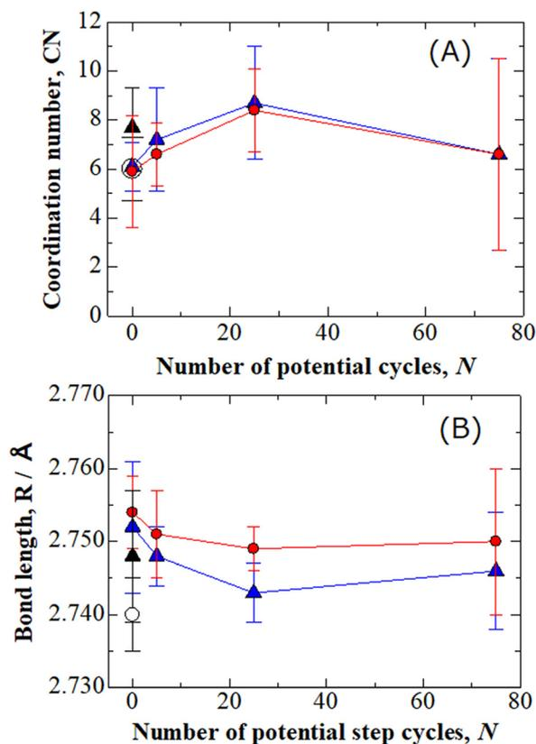
Fig. 11 (A) CN and (B) *R* as a function of *N*. The working electrode potentials were (▲) 0.4 V and (●) 1.0 V. The (▲) and (○) plots are the results for a commercial Pt/C electrode at 0.4 V and 1.0 V, respectively.
