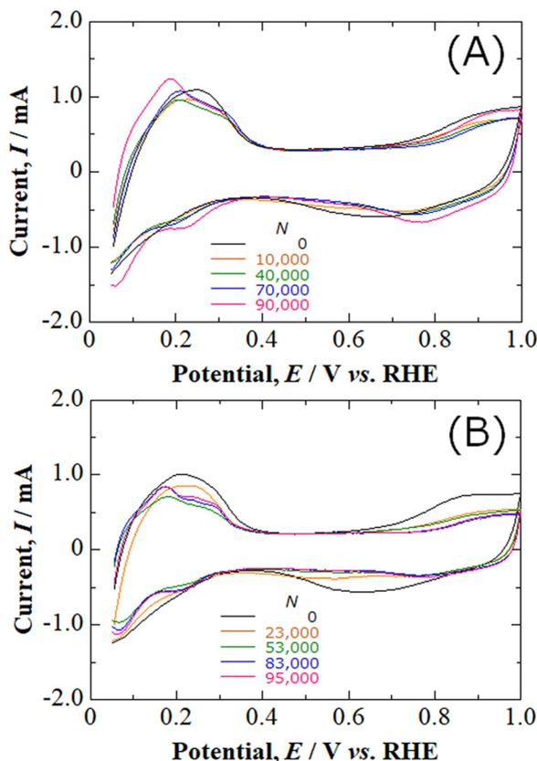
Fig. 3 Cyclic voltammograms to determine the ECSA for Nafion-coated (A)  $\text{PtCl}_n/\text{Fe-N-C}$  and (B)  $\text{Pt}/\text{Fe-N-C}$  electrodes in 0.1 M  $\text{HClO}_4$  solution deaerated with Ar at 25 °C.
