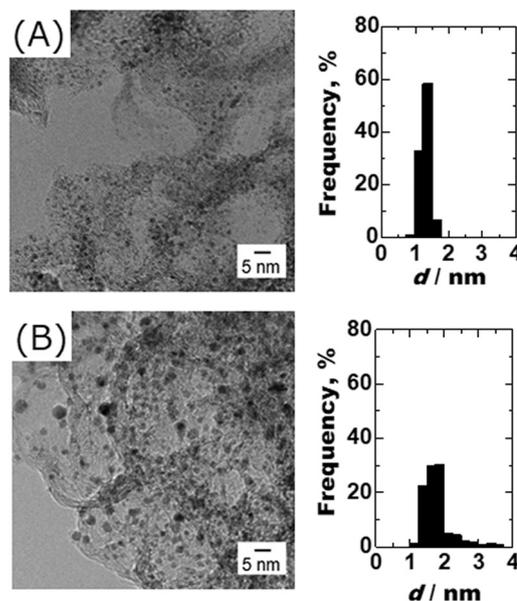
Fig. 2 TEM images and particles size distributions for (A)  $\text{PtCl}_n/\text{Fe-N-C}$  and (B) Pt/Fe-N-C powders.
