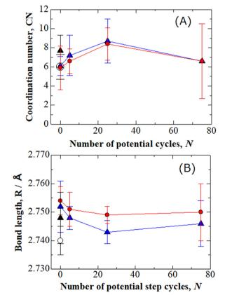
Fig. 11 (A) CN and (B) R as a function of N. The working electrode potentials were (A) 0.4 V and (I) 1.0 V. The (A) and (I) plots are the results for a commercial Pt/C electrode at 0.4 V and 1.0 V, respectively.
