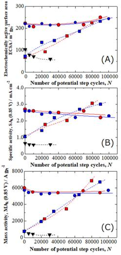
Fig. 6 (A) ECSA, (B)  ${\rm SA_{k\prime}}$  and (C)  ${\rm MA_{k}}$  for the ORR for Nafion-coated (  $\bullet$  )  $(PtCl_n)_{1.3nm}/Fe-N-C$ , (•) \*[ $(PtCl_n)_{1.3nm}/Fe-N-C$ ], (•)  $(PtCl_n)_{0.9nm}/Fe-N-C$ , (•) \*[( $PtCl_n$ )<sub>0.9nm</sub>/Fe-N-C], and ( $\blacktriangledown$ ) commercial Pt/C electrodes as a function
