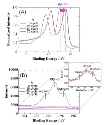
Fig. 8 XPS (A) Pt 4f and (B) Cl 2p spectra obtained from (PtCl<sub>n</sub>)<sub>0.9nm</sub>/ Fe-N-C powders before and after potential cycles (N).
