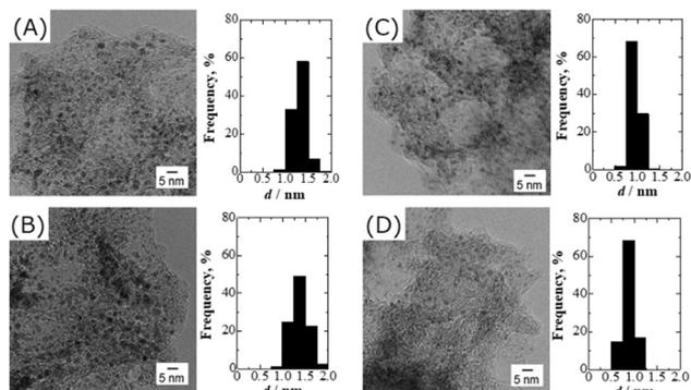
**Fig. 5** TEM images and particle size distributions for (A) (PtCl<sub>n</sub>)<sub>1.3nm</sub>/Fe-N-C, (B) \*[(PtCl<sub>n</sub>)<sub>1.3nm</sub>/Fe-N-C], (C) (PtCl<sub>n</sub>)<sub>0.9nm</sub>/Fe-N-C, and (D) \*[(PtCl<sub>n</sub>)<sub>0.9nm</sub>/Fe-N-C] powders.
