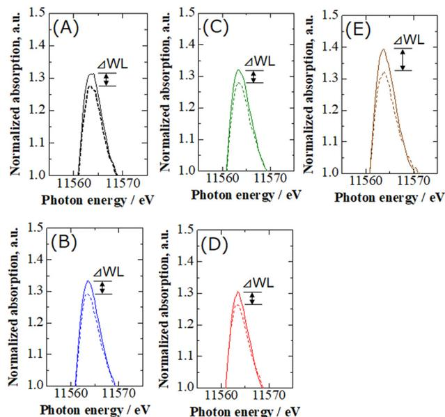
**Fig. 10** XANES spectra of  $(\text{PtCl}_n)_{0.9\text{nm}}/\text{Fe–N–C}$  electrode with (A)  $N = 0$ , (B)  $N = 5$ , (C)  $N = 25$ , and (D)  $N = 75$  and (E) commercial Pt/C ( $N = 0$ ) at (---) 0.4 V and (—) 1.0 V in  $\text{N}_2$ -purged 0.1 M  $\text{HClO}_4$ .
