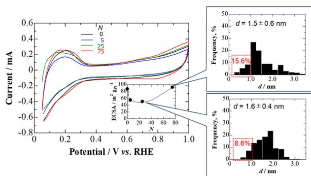
**Fig. 9** Cyclic voltammograms employed to determine the ECSA values and particle size distribution histograms for Nafion-coated  $(\text{PtCl}_n)_{0.9\text{nm}}/\text{Fe–N–C}$  electrode in 0.1 M  $\text{HClO}_4$  solution deaerated with  $\text{N}_2$  at room temperature at a scan rate of  $50 \text{ mV s}^{-1}$ .
