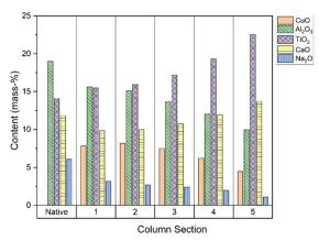
Fig. 12 Metal oxide distribution in the column after adsorption by XRF. The concentration of copper solution after 31 adsorptiondesorption cycles was 1000 mg L<sup>-1</sup>, pH was 4.5 and temperature 25 °C. Fresh adsorbent is labeled as native for comparison.
