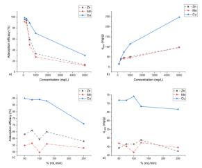
Fig. 8 The effect of concentration and flow rate on adsorption efficacy (a and c) and q-values (b and d). (a and b) Flow rate 100 mL min<sup>-1</sup>, pH 4.5 and temperature 25 °C. (c and d) Concentration 500 mg L<sup>-1</sup>, pH 4.5 and temperature 25 °C.
