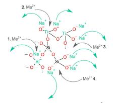
Fig. 14 Possible adsorption mechanism of Me<sup>2+</sup> titanatemodified AAM.
