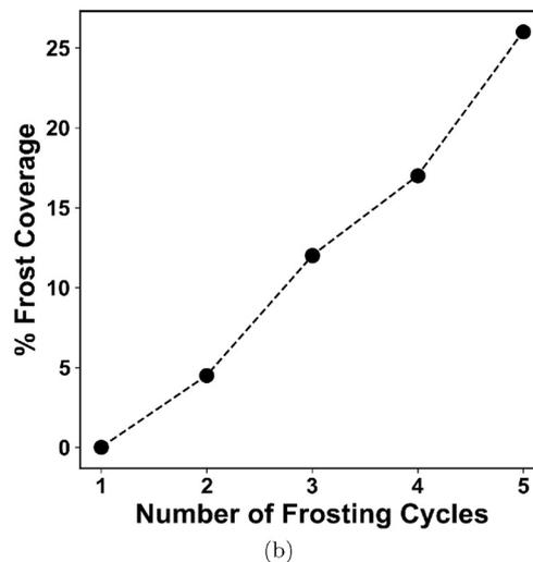
**Fig. 6** (a) Anti-icing performance of E-ICE coating under multiple freeze–thaw cycles. Frosting conditions employed are: surface temperature =  $-20\text{ }^{\circ}\text{C}$ , room conditions =  $28\text{ }^{\circ}\text{C}$  and 60% RH, cycle time = 60 min. The first row depicts the surface at the start of the cycle while the second row depicts the surface at the end of the 60 min cycle (b) quantitative representation of % frost coverage on E-ICE with the number of cycles.
