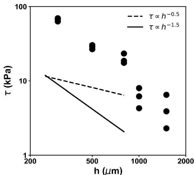
Fig. 8 Variation of ICE adhesion stress (IAS) of E-ICE coating with the thickness of the coating. Experiments were performed at the surface temperature of  $-20\text{ }^{\circ}\text{C}$ , and the coating thickness was varied as indicated.
