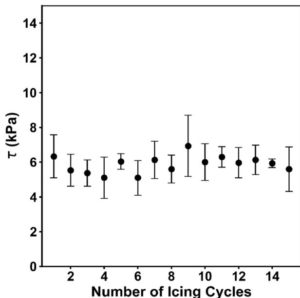
Fig. 7 Variation of ICE adhesion stress (IAS) of E-ICE coating with the number of icing cycles. Experiments were performed at, surface temperature =  $-20\text{ }^{\circ}\text{C}$ , and coating thickness =  $\sim 1\text{ }\mu\text{m}$ .
