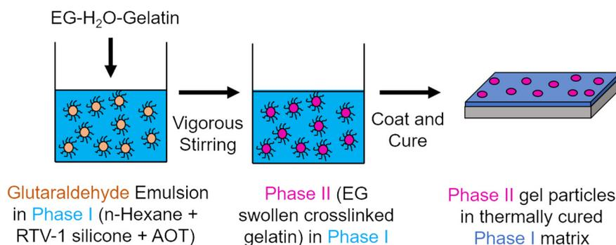
Fig. 3 Schematic of preparation of E-ICE coating.
