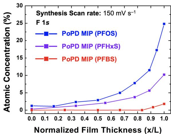
Fig. 8 Normalized XPS SDP of the F 1s signal for the representative MIP films imprinted with PFOS, PFHxS, and PFBS at the same synthesis scan rate of  $150 \text{ mV s}^{-1}$ . Values are the averaged values from separate measurements ( $N \geq 3$ ).
