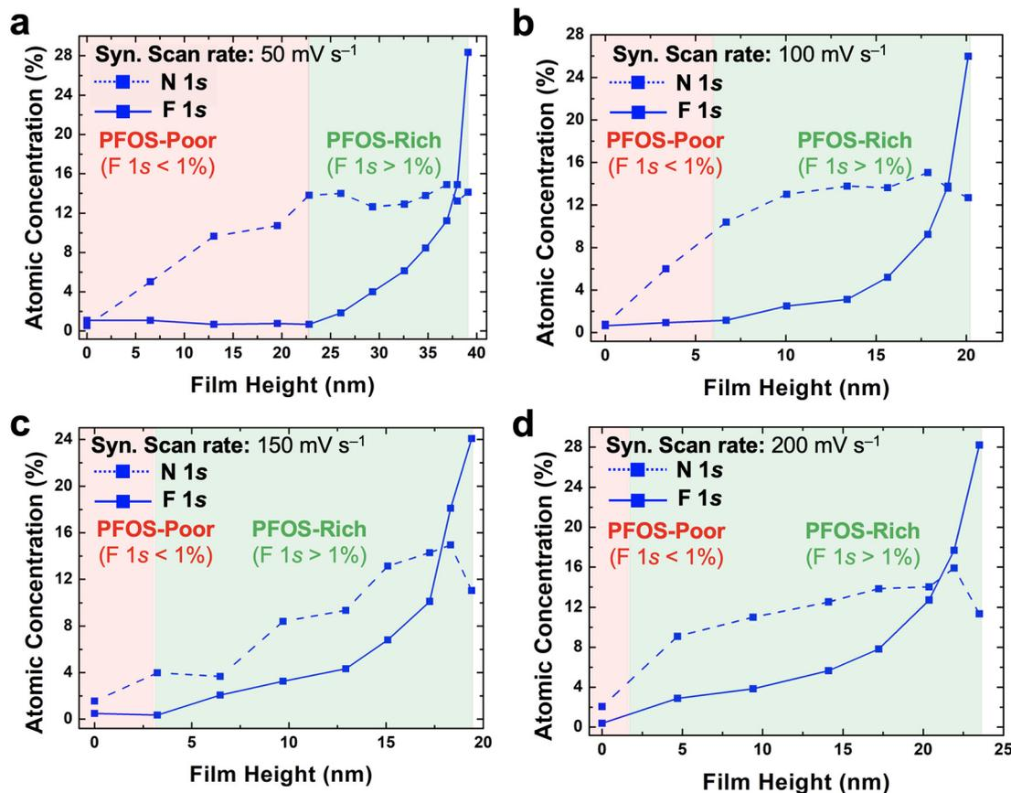
Fig. 4 Representative elemental analyses using XPS SDP for MIP films imprinted with PFOS using different synthesis scan rates (“syn. scan rate”): (a) 50, (b) 100, (c) 150, and (d) 200  $\text{mV s}^{-1}$ . We used the N 1s signal to designate the presence of the MIP films and the F 1s signal for the presence of imprinted PFOS. We defined the PFOS-poor region where the F 1s signal was less than 1% of the atomic concentration, and the PFOS-rich region where the F 1s signal was greater than 1%.
