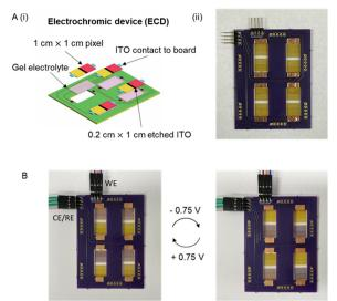
Fig. 3 Integration of the PGE with arrayed pixels. (A)(i) Schematic of the board and pixel integration scheme and (ii) image showing the integrated pixels (each consisting of two 1 cm<sup>2</sup> printed squares) with the PGE on the printed circuit board before polarization. (B) Chronoamperometric application of a ±0.75 V DC potential (200 s per cycle) demonstrated the capability for synchronized colour change. Within the pixel array.
