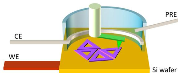
**Fig. 1** Schematic representation of the experimental setup. The electrochemical cell (blue) is placed on top of the Si wafer, which acts as the working electrode (WE). The cell houses the platinum counter electrode (CE) and the platinum pseudo-reference electrode (PRE). The AFM cantilever (green) is not used as an electrode.
