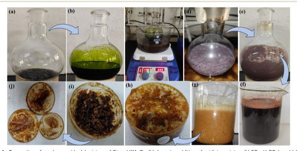
Scheme 1 Preparation of graphene oxide: (a) mixture of Gt and  $KMnO_4$ , (b) dropwise addition of oxidizing mixture ( $H_2SO_4$ :  $H_3PO_4$ ), and (c) stirring at 55 °C at 650 rpm. (d) Mixture after 12 hours and (e) at room temperature, (f) addition of ice-cold water at a slow rate, (g) treatment with H<sub>2</sub>O<sub>2</sub> (30%), (h) coagulation with petroleum ether (i) corresponding image after 2 hour, and (j) developed 2D-GO sheet by using the modified hummer's method.26
