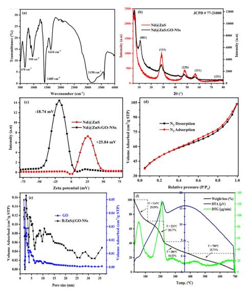
Fig. 1 (a) FT-IR spectrum of Nd@ZnS:GO-NSs, (b) P-XRD pattern of Nd@ZnS:GO-NSs (black) and Nd@ZnS (red), (c) comparative zeta potential of Nd@ZnS:GO-NSs (black) and Nd@ZnS (red), (d) N<sub>2</sub> adsorption-desorption isotherm of Nd@ZnS:GO-NSs at 77 K, (e) comparative pore size of GO (blue) and Nd@ZnS:GO-NSs (black), and (f) TGA, DTA, and DTG analysis of Nd@ZnS:GO-NSs.
