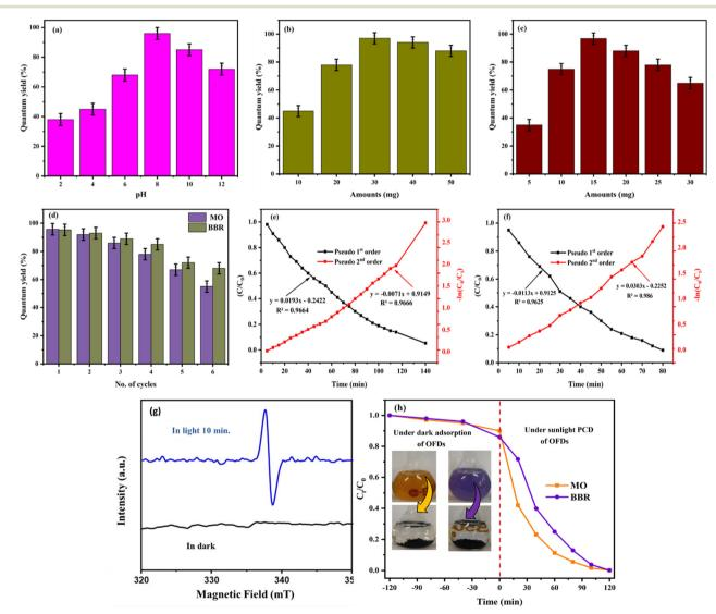
Fig. 4 (a) Effect of pH on photodegradation activities. (b and c) Effect of Nd@ZnS:GO-NSs dosage on MO and BBR photodegradation. (d) Reusability of the catalyst. (e) and f) Kinetics of the catalyst. (g) EPR analysis of the catalyst. (h) Degradation kinetics in the dark and in the presence of sunlight.
