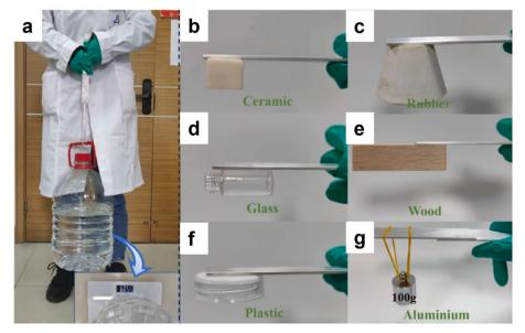
Fig. 13 Digital images of (a) weight support of the steel substance adhered by the NIPU adhesive exposed under -37 °C. (b)-(g) adhesion of NIPU to different substances. Reproduced with permission from ref. 13. Open access: Polym. Test.
