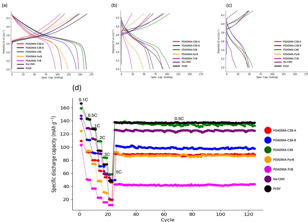
**Fig. 4** (a) Cycling performance of NMC622 cathode and lithium anode using different binders at 0.1C (fourth cycle). (b) Cycling performance of NMC622 cathode and lithium anode using different binders at 2C (fourth cycle). (c) Cycling performance of NMC622 cathode and lithium anode using different binders at 5C (fourth cycle). (d) Cycling performance for 100 cycles at 0.5C using different binders.
