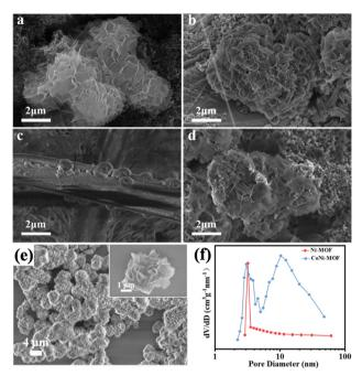
Fig. 20 SEM images of the CoNi-MOF cathodes: (a) fresh cathode, (b) discharge to 600 mAh  $\rm g^{-1}$ , (c) discharged to 2000 mAh  $\rm g^{-1}$  and (d) recharged to 2000 mAh  $\rm g^{-1}$ . (e) SEM images of CoNi-MOF (the inset is an enlarged SEM image). (f) Pore size distribution curve of Ni-MOF and CoNi-MOF. (a-f) Reproduced with permission. 134 Copyright 2024, the American Chemical Society.
