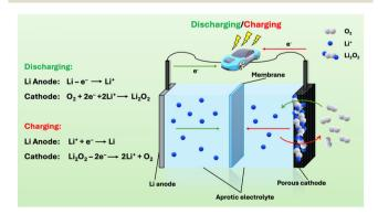
Fig. 1 Structure and working principles of aprotic LOBs. During discharge,  $Li^+$  ions move from the anode zone to the cathode zone, where  $O_2$  molecules are reduced on the cathode and then combine with  $Li^+$  to form insoluble  $Li_2O_2$ . During charge,  $Li^+$  ions move backwards, and  $Li_2O_2$  is oxidized to  $O_2$ , ideally.
