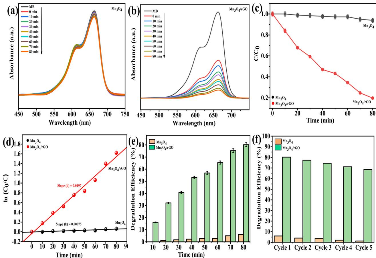
Fig. 5 (a and b) Absorption spectra showing the breakdown of MB in the presence of Mn<sub>3</sub>O<sub>4</sub> NMs and Mn<sub>3</sub>O<sub>4</sub>/rGO NCs, (c) analysis of the degradation rate, (d) pseudo-first-order kinetics for the reaction, (e) efficiency of dye degradation, and (f) reusability test for the Mn<sub>3</sub>O<sub>4</sub> NM and Mn<sub>3</sub>O<sub>4</sub>/rGO NC catalysts.
