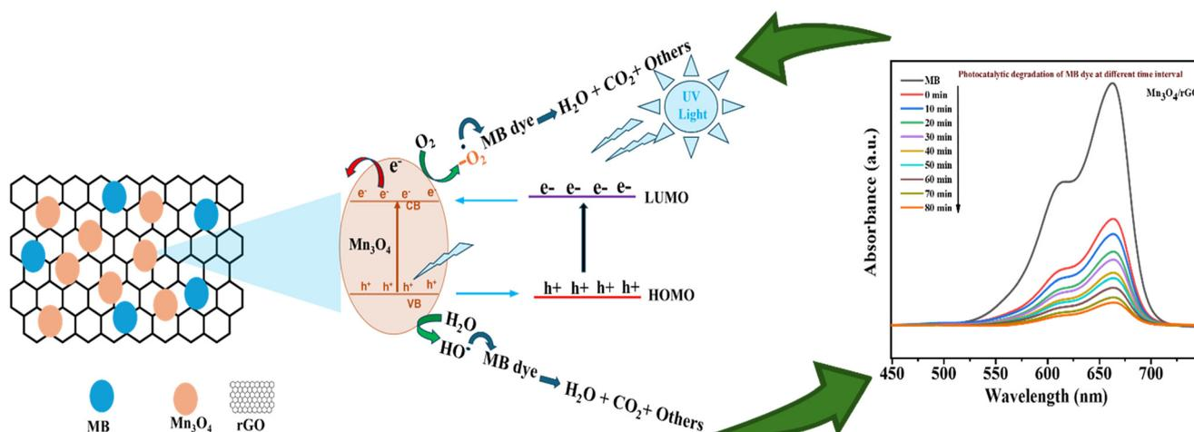
Scheme 3 Detailed degradation of MB dye in the presence of Mn<sub>3</sub>O<sub>4</sub>/rGO NC catalysts.
