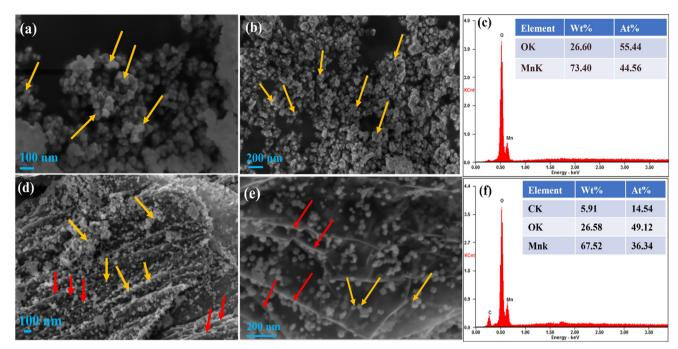
Fig. 2 (a and b) SEM images of  $Mn_3O_4$  NMs, (c) EDS energy spectrum of  $Mn_3O_4$  NMs, (d and e) SEM image of  $Mn_3O_4/rGO$  NCs, (f) EDS energy spectrum of  $Mn_3O_4/rGO$  NCs.
