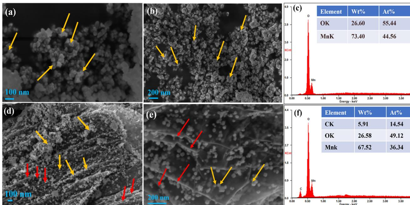
Fig. 2 (a and b) SEM images of  $\text{Mn}_3\text{O}_4$  NMs, (c) EDS energy spectrum of  $\text{Mn}_3\text{O}_4$  NMs, (d and e) SEM image of  $\text{Mn}_3\text{O}_4/\text{rGO}$  NCs, (f) EDS energy spectrum of  $\text{Mn}_3\text{O}_4/\text{rGO}$  NCs.
