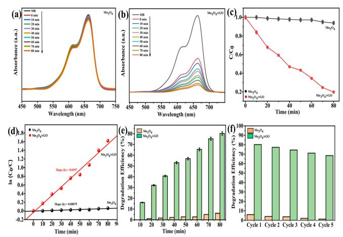
Fig. 5 (a and b) Absorption spectra showing the breakdown of MB in the presence of Mn<sub>3</sub>O<sub>4</sub> NMs and Mn<sub>3</sub>O<sub>4</sub>/rGO NCs, (c) analysis of the degradation rate, (d) pseudo-first-order kinetics for the reaction, (e) efficiency of dye degradation, and (f) reusability test for the Mn<sub>3</sub>O<sub>4</sub> NM and Mn<sub>3</sub>O<sub>4</sub>/rGO NC catalysts.
