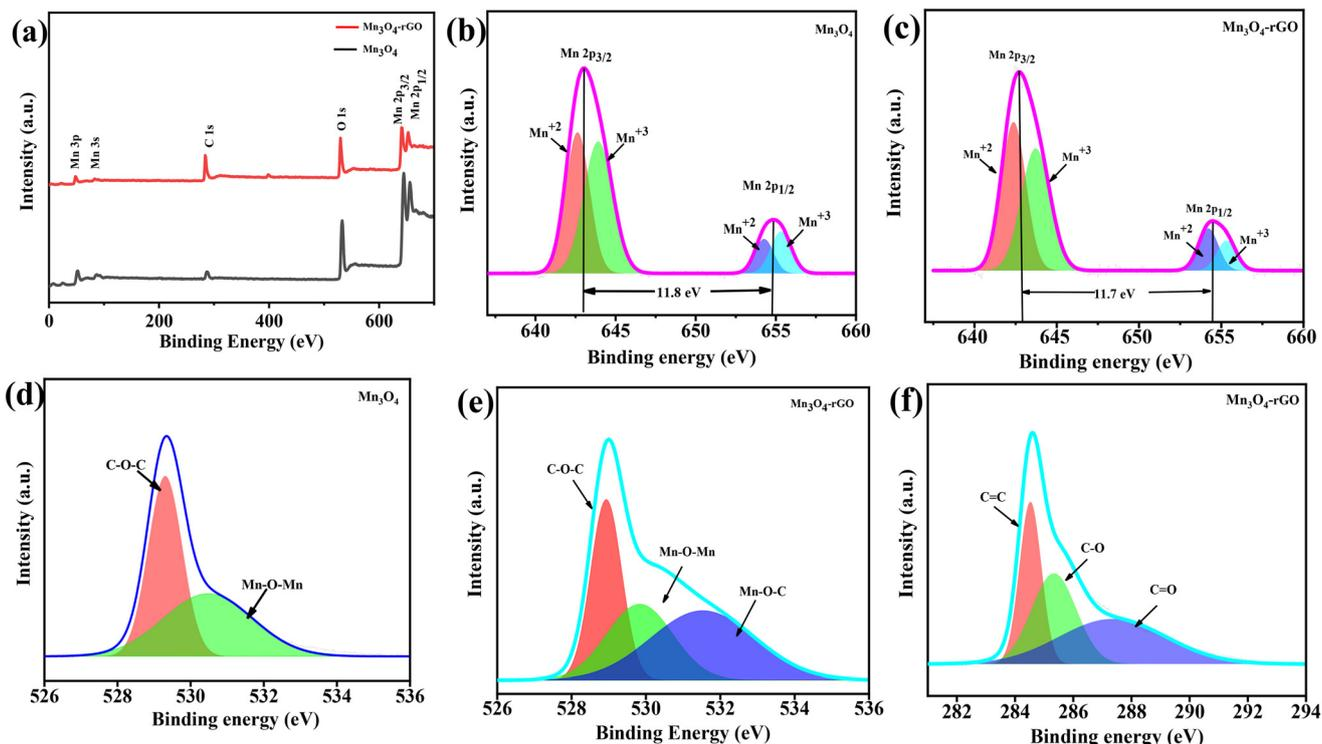
Fig. 4 (a) Survey spectrum, (b and c) HR Mn 2p spectra, (d and e) HR Mn O 1s spectrum of  $\text{Mn}_3\text{O}_4$  NMs and  $\text{Mn}_3\text{O}_4/\text{rGO}$  NCs, and (f) HR Mn C 1s spectrum of  $\text{Mn}_3\text{O}_4/\text{rGO}$  NMs.
