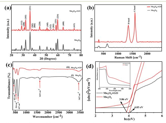
Fig. 1 (a) XRD, (b) Raman, (c) FTIR, and (d) UV spectra of the as-synthesized Mn<sub>3</sub>O<sub>4</sub> NMs and Mn<sub>3</sub>O<sub>4</sub>/rGO NCs.
