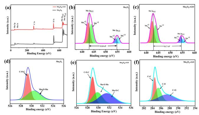
Fig. 4 (a) Survey spectrum, (b and c) HR Mn 2p spectra, (d and e) HR Mn O 1s spectrum of  $Mn_3O_4/rGO$  NCs, and (f) HR Mn C 1s spectrum of  $Mn_3O_4/rGO$  NMs.
