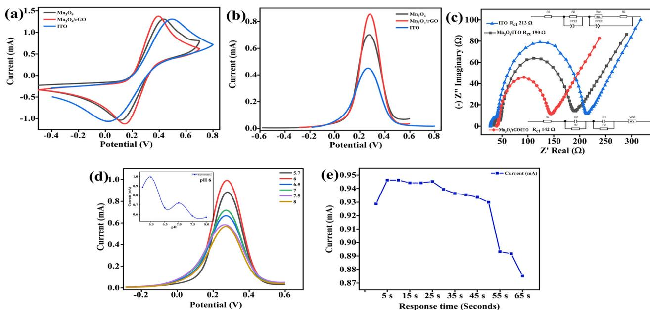
Fig. 7 (a) CV of modified electrodes in PBS containing ferri-/ferrocyanide at 0.05 V s<sup>-1</sup> scan rate. (b) DPV of various modified electrodes in PBS containing ferri-/ferrocyanide. (c) EIS of various modified electrodes in PBS containing ferri-/ferrocyanide. (d) CV spectrum of Mn<sub>3</sub>O<sub>4</sub>/rGO/ITO at distinct pH (5.7 to 8) PBS with an inset of pH calibration curve. (e) Response time calibration plot of the Mn<sub>3</sub>O<sub>4</sub>/rGO/ITO electrode.
