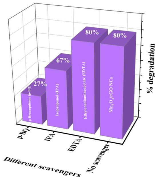
Fig. 6 MB dye degradation with and without scavengers.
