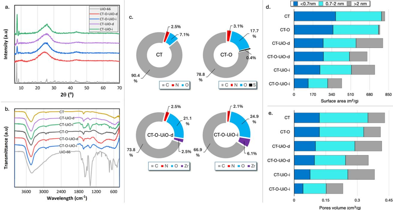
Fig. 2 X-Ray diffractogram (a), FTIR spectra (b), XPS results of C, N, O, and Zr atomic (%) concentration<sup>26</sup> (c), contributions of surface areas (d), and pore volumes in specific pore sizes (e) derived from N<sub>2</sub> adsorption experiments.
